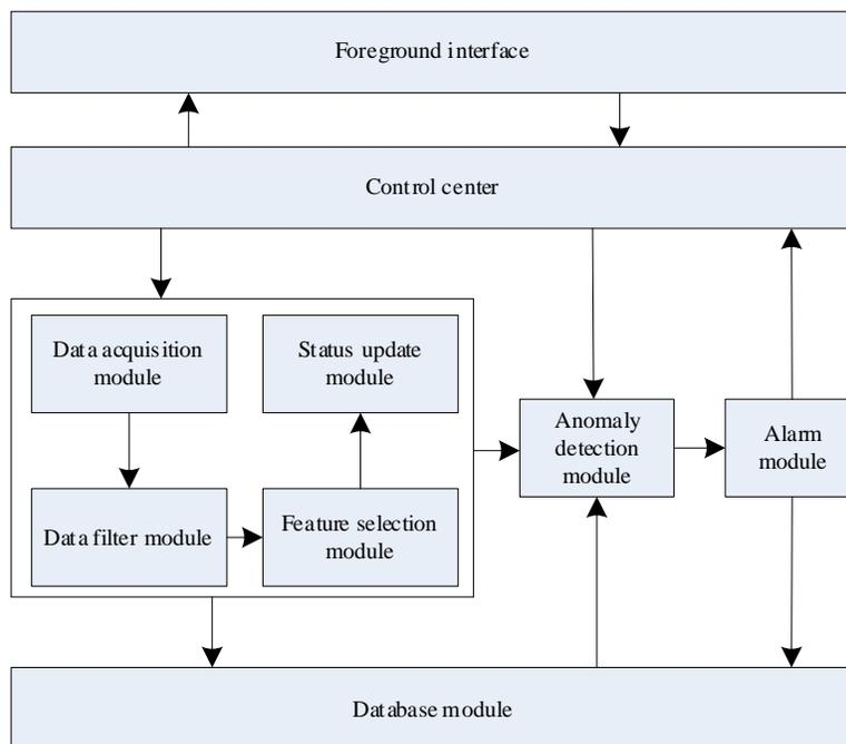
Fig. 1. Overall design of network security detection architecture.
