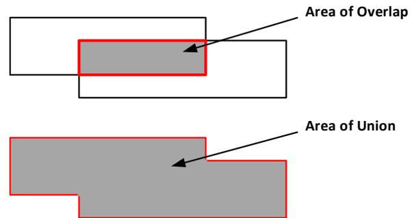
Fig. 4. Diagrammatic example intersection over union (IoU) calculation.
