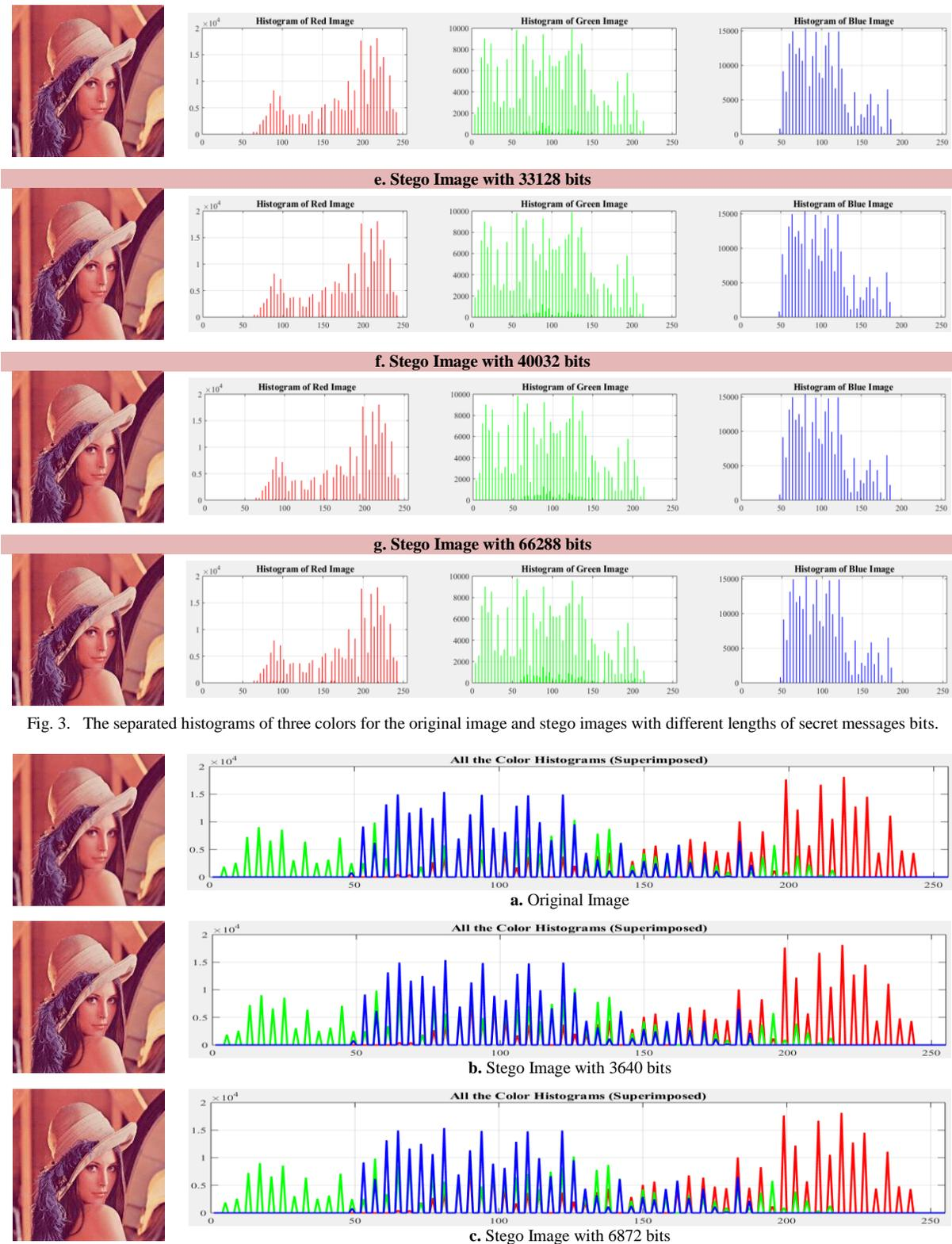
Fig. 3. The separated histograms of three colors for the original image and stego images with different lengths of secret messages bits.
