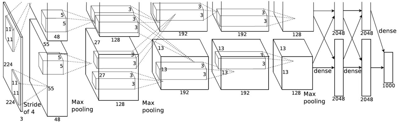
Fig. 3. The concept of AlexNet [29].
