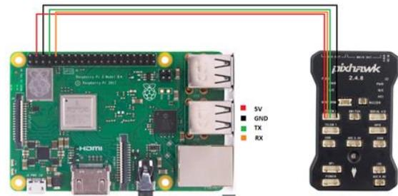
Fig. 1. Connections from raspberry Pi to Pixhawk 2.4.8.
