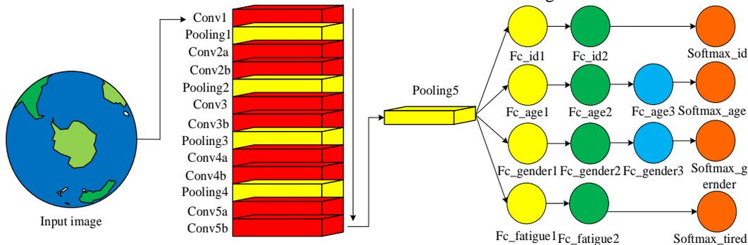
Fig. 4. Multi task face recognition network structure.
