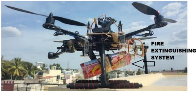
Fig. 12. Setup of the fire extinguishing system.
