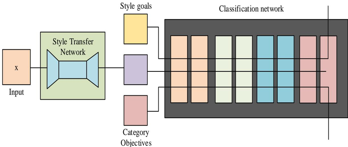
Fig. 4. Network structure of real-time style transfer network.
