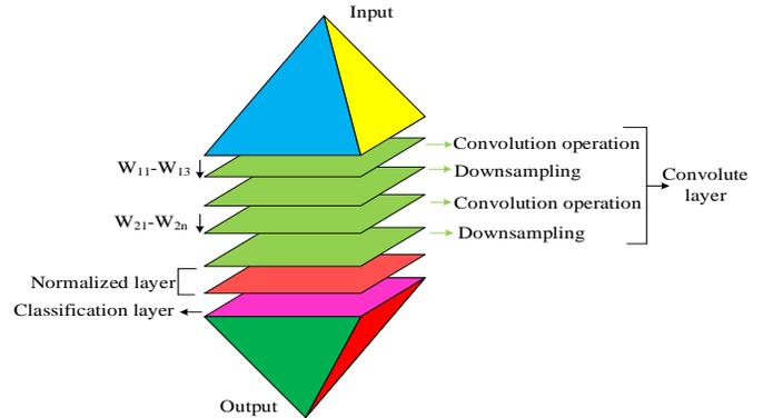
Fig. 1. Principle and structure of CNN.
