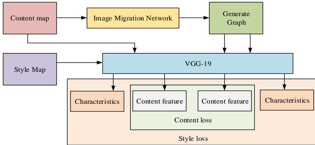
Fig. 6. Improved real-time style migration network structure diagram.
