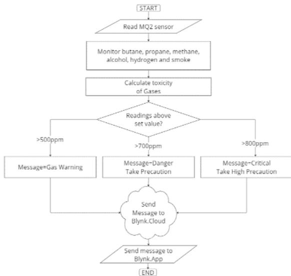
Fig. 8. Workflow of air quality monitoring system.
