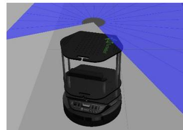
Fig. 6. The Turtlebot2 robot equipped with a lidarsensor.
