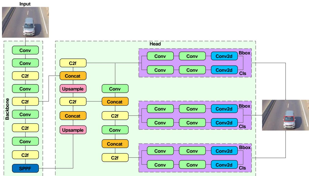
Fig. 5. The architecture of the YOLOv8 model.
