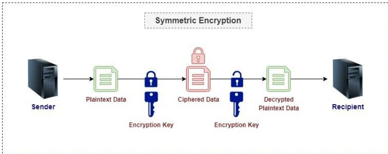
Fig. 3. Symmetric encryption.
