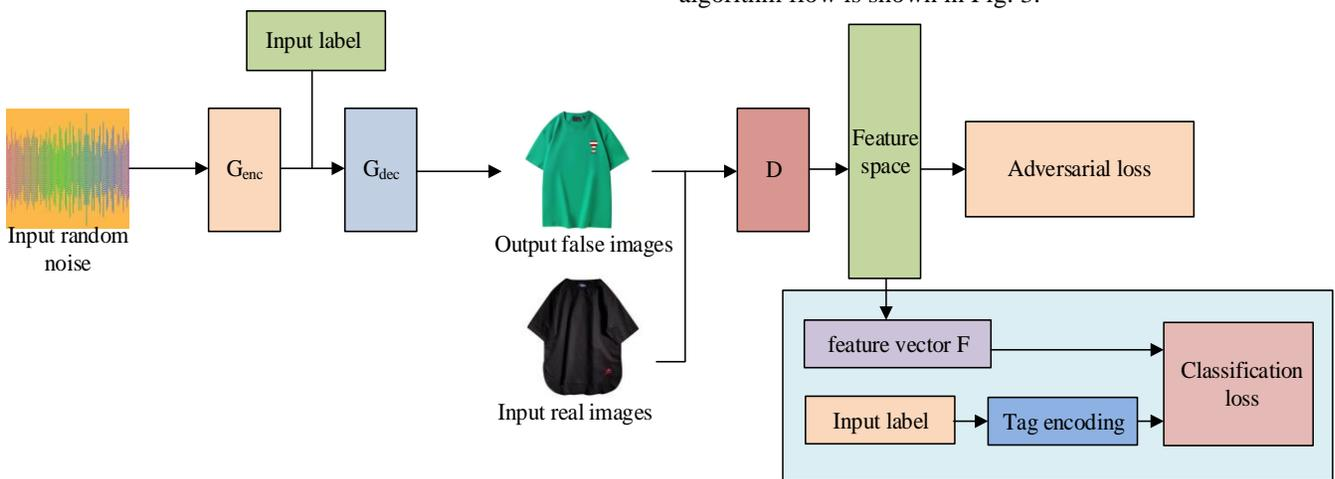
Fig. 2. Improved DCGAN network training stage structure diagram.
