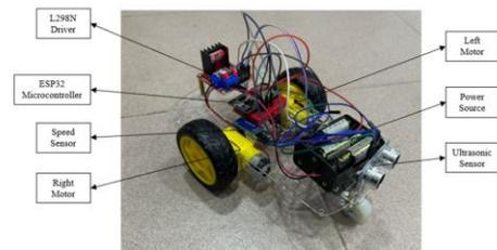
Fig. 7. Robot prototype used in this study.
