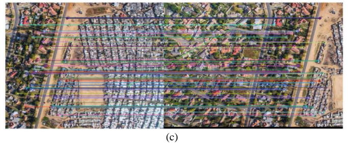
Fig. 6. Matching features (a) SIFT (b) BRISK (c) Proposed.
