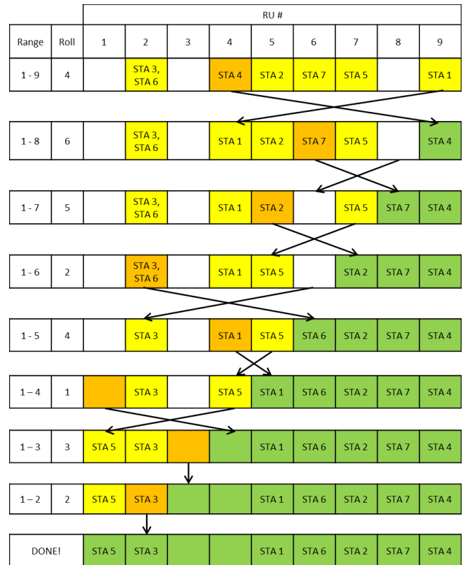
Fig. 4. Recomputation of array for RUs allocation by using Fisher-Yates shuffle.
