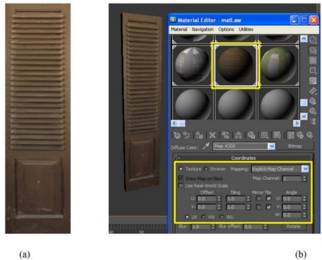
Fig. 11. Illustrations of (a) that is the door profile image used in the image texture mapping implementation for a 3D box object (b).
