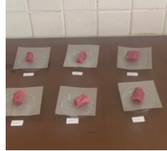
Fig. 4. The samples are placed on a petri dish with a wire mesh base.
