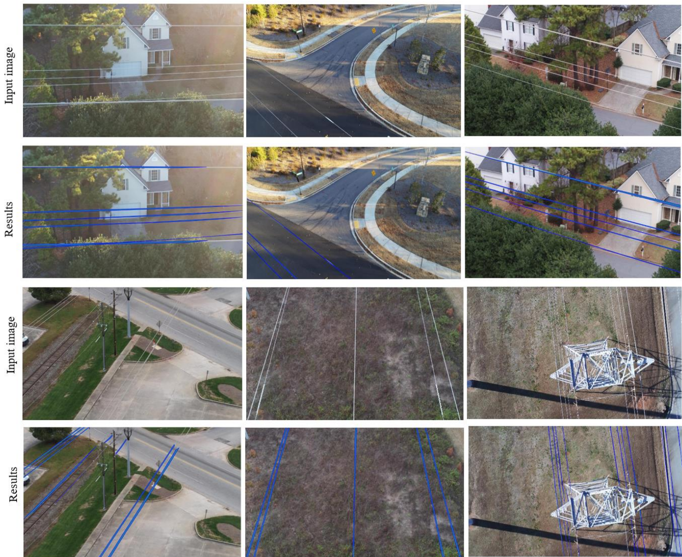
Fig. 4. Sample transmission line segmentation results of the proposed model.
