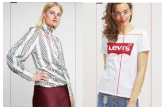
Fig. 14. Detectron open pose detection results (better but some important points are still missing).
