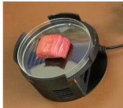
Fig. 10. NeoSpectra development kit with case and sample.
