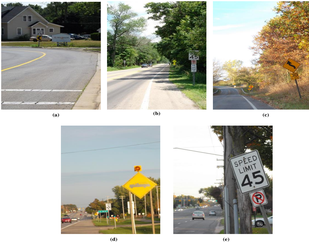
Fig. 4. Examples of low visibility road signs due to: a) Color difference between sign and surroundings, b) Occlusion, c) Complexity of surrounding regions, d) Readability of sign foreground, e) Tilting.
