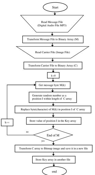
Fig. 2. Algorithm of steganography in images using bytes
