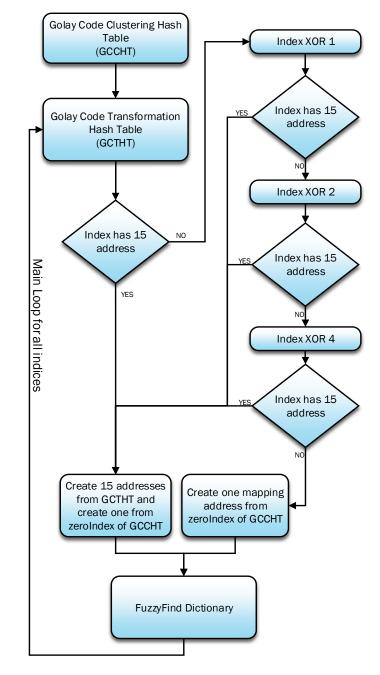
Fig. 1. Pipeline of generating FuzzyFind Dictionary using Golay Code Clustering Hash Table (GCCHT) and indicates the generating Golay Code Transformation Hash Table (GCTHT), and finally create FuzzyFind Dictionary, "This algorithms is pre-processing algorithm for text manning and searching through big data"
