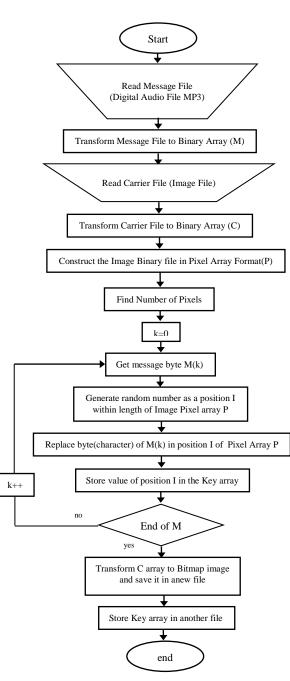
Fig. 7. Algorithm of steganography in images using pixels
