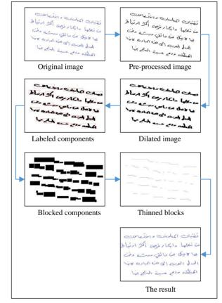
Fig. 6. Steps of skew detection and correction
