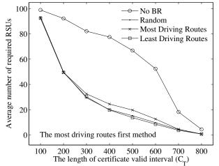
Fig. 7: The average number of required RSUs when the most driving routes first RSU allocation method is employed
