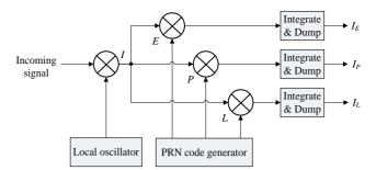
Fig. 4. Basic code tracking loop block diagram
