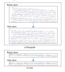
Fig. 7. Sample of skew detection and correction, a) a paragraph b) a line
