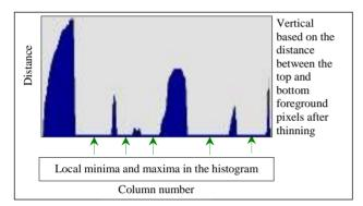
Fig. 10. Extracting the word images based on horizontal histogram after thinning
