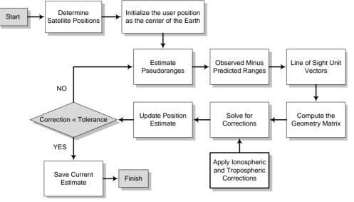
Fig. 6. Computational flow diagram of our positioning algorithm
