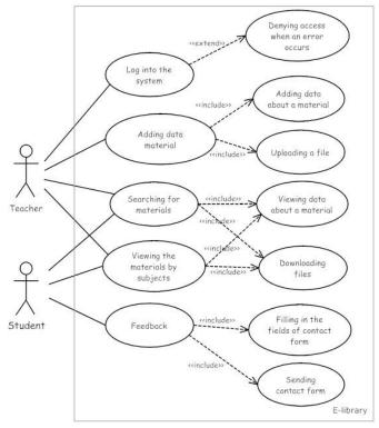
Fig. 1. Interface with UML diagram
