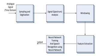
Figure 2. Connectionist based speech recognition model
