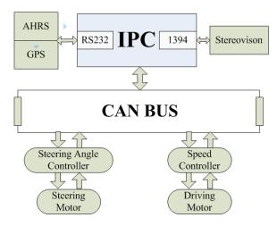
Figure 2. Hardware block diagram of UGV.
