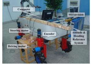
Figure 1. UGV used for navigation experiment.
