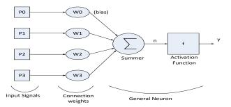
Figure 1. Mathematical Model of a basic neural network
