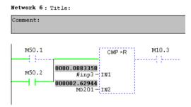
Figure 10. Compare Logic Element (CMP) in FB1
