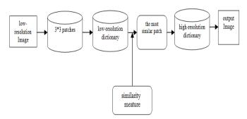
Figure 2. Deblurring License Plate Image Framework
