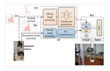
Figure 1. Structure of the designed AMPCS.
