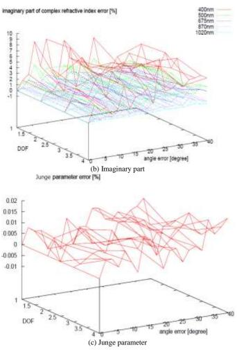
Fig. 6. Solar direct pointing angle error on the estimated real part, imaginary part of refractive index and Junge parameter
