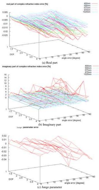
Fig. 8. Solar diffuse pointing angle error on the estimated real part, imaginary part of refractive index and Junge parameter
