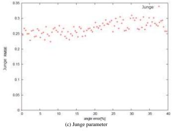
Fig. 5. RMSE of the aerosol parameter estimation caused by solar direct pointing angle errors
