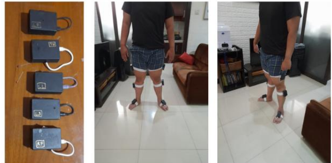
Fig. 7. Place the IMU sensor device on the respondent's leg using a rubber band.
