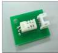
Figure 2: Humidity Sensor Module HSM-20G
