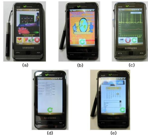
Figure 7. Mobile Phone Configuration: (a) monitoring system main view; (b) wireless connection; (c) real-time display of the ECG measurement; (d) the ECG parameters calculation value; (e) data history and management
