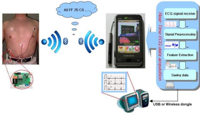
Figure 1. Real-time ECG system block diagram
