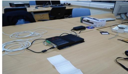
Fig. 4. RFID system (the Alien ALR-8800 RFID reader)
