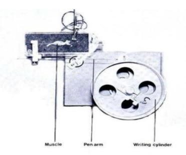
Fig. 1. Conventional Kymograph (front view)
