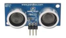
Fig. 3. Ultrasonic distance sensor [6]
