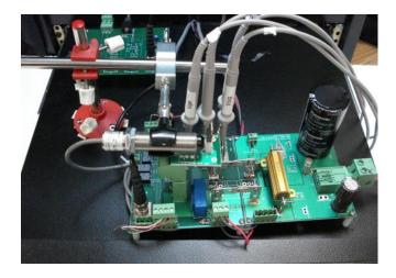
Fig. 1. IGBT accelerated aging experiments hardware [10].
