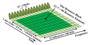
Fig. 1. The resource block and subcarrier in LTE-SCFDMA
