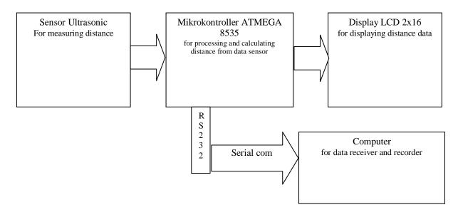
Fig. 8. Hardware system in Computerized kymograph
