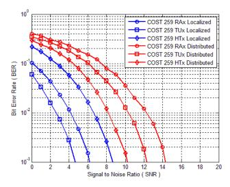
Fig. 12. The performance under COST 259 channel models
