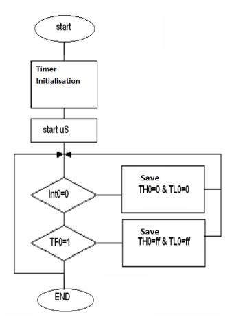
Fig. 4. Flowchart of Ultrasonic distance sensor
