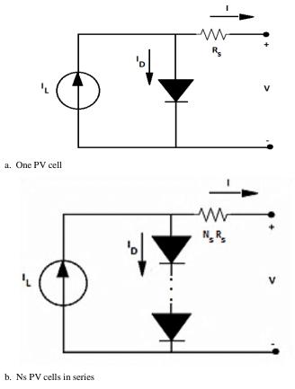
Fig. 1. PV cell models
