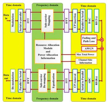
Fig. 2. The block diagram of the SCFDMA system
