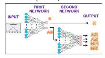
Fig. 4. Classification of 5 categories of heart sound signal using hierarchical MLP network.
