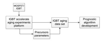
Fig. 2. Process of IGBT prognostic algorithm development.
