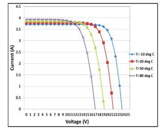
Fig. 4. ig. 4. I-V plots for various temperatures with Ns = 36, n = 1.2, suns = 1, Np = 1
