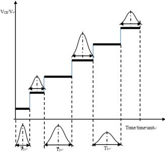
FIGURE 5: IGBT Degradation Model.
