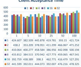
Fig. 10. Client acceptance Time ( $TC_{acc}$ ) in nanoseconds versus number ARP cache records for different number of users in normal worload
