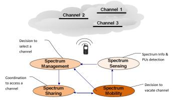
Fig. 1. Cognitive radio main functions
