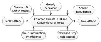
Fig. 4. Common security threats in conventional wireless and CR Networks
