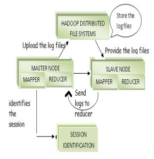
Fig. 5. Data processing in hadoop file system
