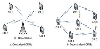
Fig. 3. Cognitive radio architecture
