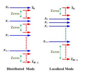
Fig. 3. The two types of sub-carrier mapping
