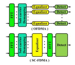
Fig. 7. The equalization in OFDMA and SCFDMA
