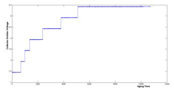
Fig. 4. Collector-Emitter Voltage after K-Mean Clustering.
