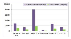
Fig. 4. UPX Compression Ratio [18]
