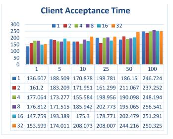
Fig. 9. Client acceptance Time (TCacc) in nanoseconds versus number ARP cache records for different number of users in light worload
