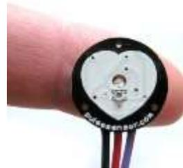
Fig. 4. Pulse rate sensor SEN-11574
