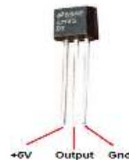
Fig. 5. Temperature sensor LM-35
