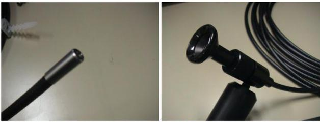
(a) Tip of fiber image scope (b) Outoptics of fiber image scope
