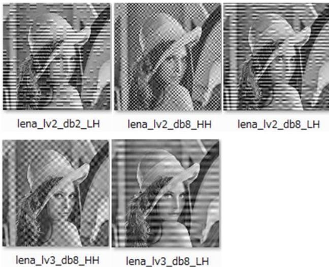
Figure 2 Some examples of reconstructed images of MRA based data hiding (lv<sub>i</sub> db<sub>j</sub> denotes i level and Daubechies base function with support length of j, respectively)
