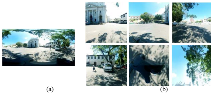
Fig. 4. (a) Represents a raw 2:1 photosphere, (b) Represents the 6 images which can be obtained after converting the photosphere to a cube map.
