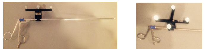
Fig. 2. Laparoscopic scissors with passive markers.
