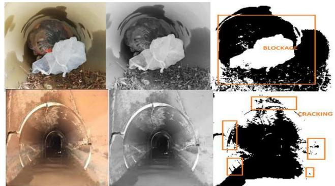
Fig. 7. Image Processing Sewer Defect Analysis.
