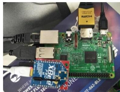
Fig. 12. Raspberry Pi 3 and Zigbee RF Module Connectivity.
