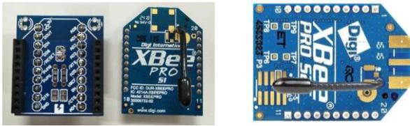
Fig. 10. Zigbee RF Module.
