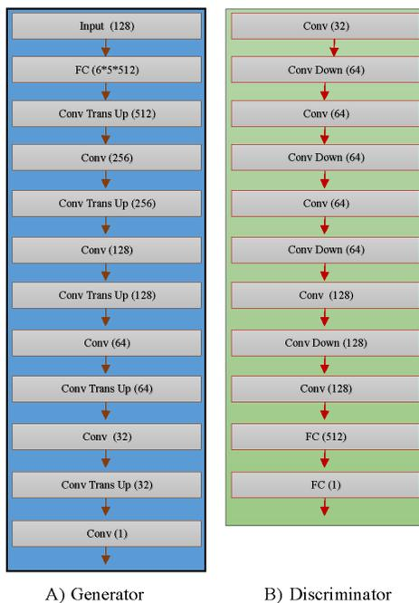
Fig. 3. DAGAN architecture: A) Generator structure and B) Discriminator structure
