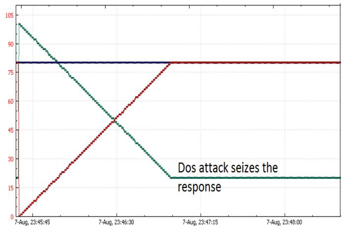
Fig. 5. DoS Attack Seized the Response from PLC.
