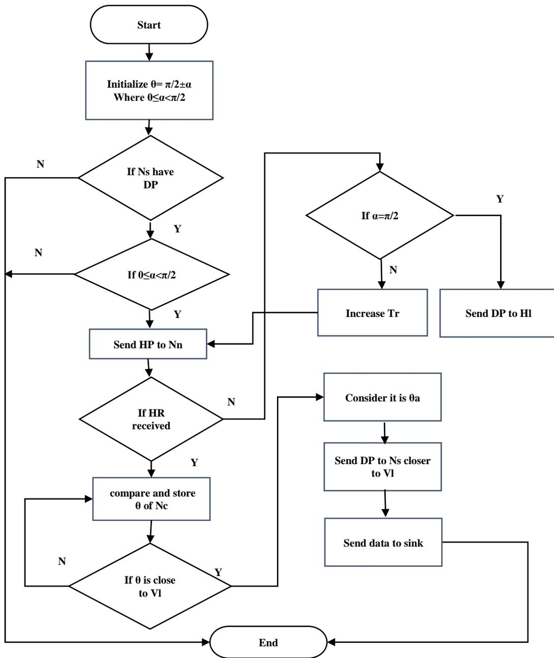
Fig. 9. Flow Chart for Data Packet Forwarding.
