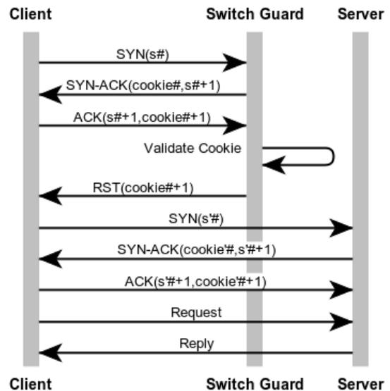
Fig. 2. TCP Reset method
