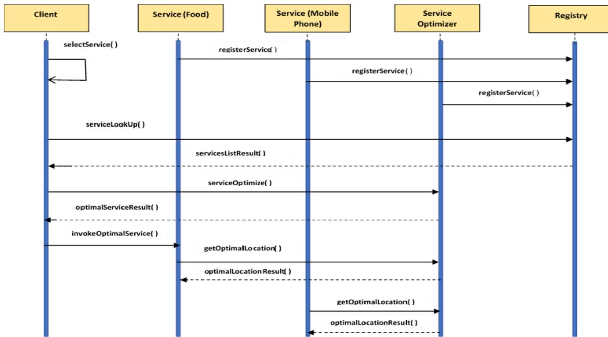
Fig. 4. The Service Distribution Sequence Diagram.
