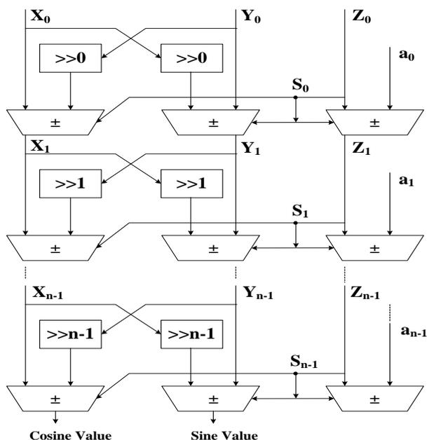
Fig. 3. Pipelined Structure used in Optimized CORDIC Model..
