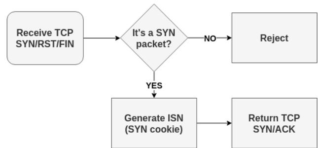
Fig. 4. Handling TCP SYN packets chart
