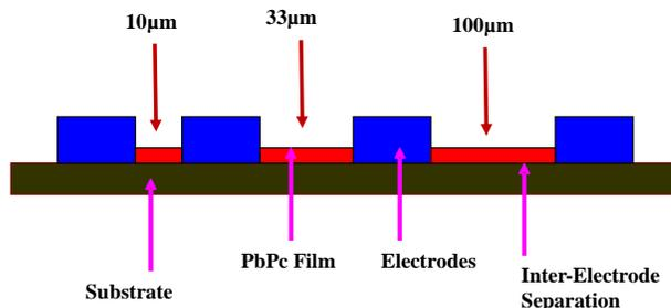
Fig. 2. Cross Section of the used PbPc Chemiresistor Array.
