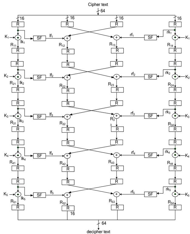
Fig. 4. Architecture of Decryption Module.
