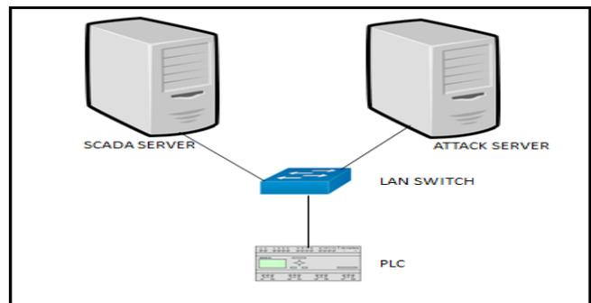
Fig. 3. Network Connectivity Diagram of Test Set up.
