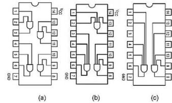
Figure 2.4 Data information (a) IC7408 (b) IC7411 (c) IC7421
