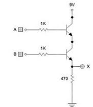
Figure 2.3 AND Gate Circuits with Transistors
