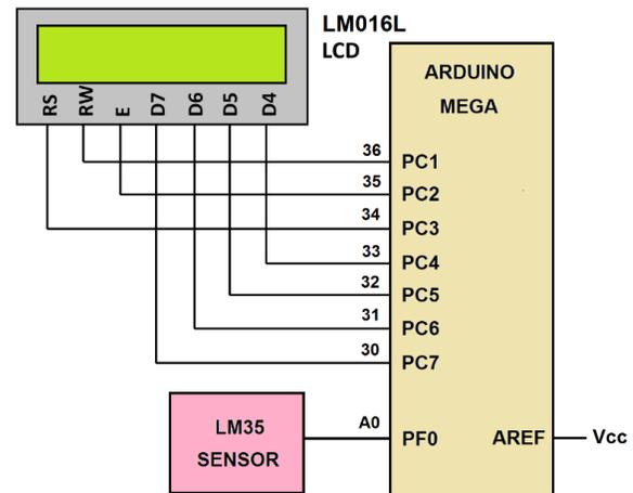
Fig. 1. Circuit Example based on the Arduino Mega.
