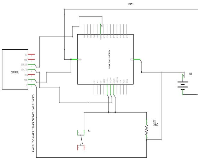
Fig. 4. The Circuit Diagram of the Device. Here, S1, R1, and U1 denotes the Switch, Resistance and Battery, Individually.
