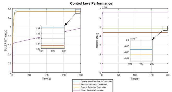
Fig. 8. EULERINT and ASCCT performance for control laws (27), (33), (41), and (52) without effects of miscellaneous disturbance torque.
