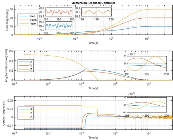
Fig. 4. Euler Angles and Angular Rate Errors produced by the miscellaneous disturbance torque in the Controller defined in (32) with a settling time (ts) of  $6.81, \pm 0.04$  degrees in the Euler Angles oscillations,  $\pm 1.9 \times 10^{-3}$  rad/s oscillations in angular rates, and  $\pm 2.1 \times 10^{-3}$  Nm in Control Torque.
