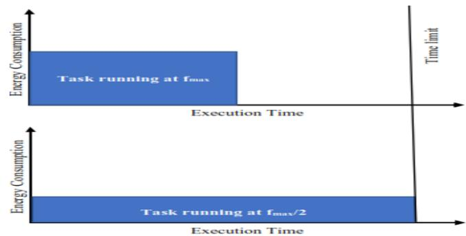
Fig. 1. Dynamic Voltage Frequency Scaling.
