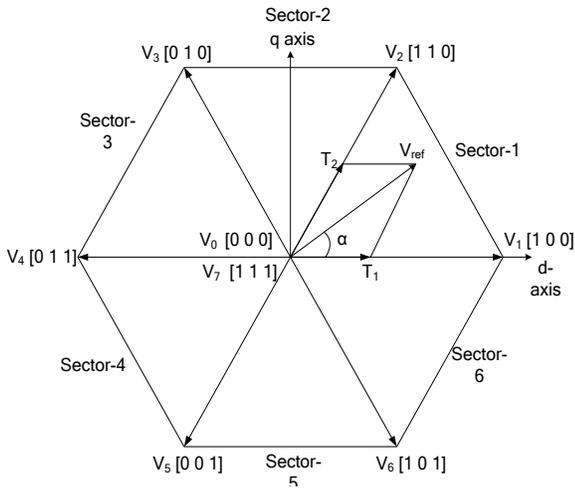
Fig. 2. Fundamental Sectors and Switching Vectors.
