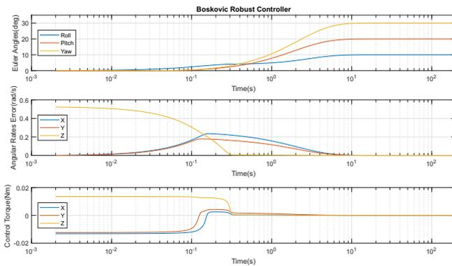
Fig. 10. Euler Angles, Angular Rate Errors and Control Torque produced by the Boskovic Robust Controller defined in (33) with a settling time (ts) of 6.32 s and average computational cost (O) of 0.159 ms. The Control Torque saturation time was 100.5 ms.
