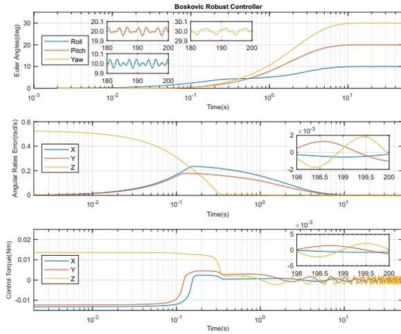
Fig. 5. Euler Angles and Angular Rate Errors produced by the miscellaneous disturbance torque in the Controller defined in (33) with a settling time (ts) of  $6.44, \pm 0.04$  degrees in the Euler Angles oscillations,  $\pm 1.8 \times 10^{-3}$  rad/s oscillations in angular rates, and  $\pm 2.1 \times 10^{-3}$  Nm in Control Torque.
