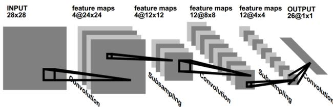
Fig. 1. Convolutional Neural Network Architecture.
