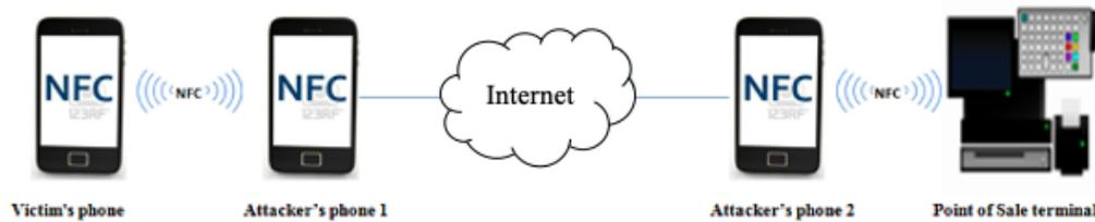
Fig. 5. NFC Relay Attack.
