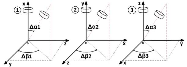
Fig. 2. Misalignments in the reaction wheels. ' $\Delta\alpha_1$ ', ' $\Delta\alpha_2$ ', ' $\Delta\alpha_3$ ' are small angles and ' $\Delta\beta_1$ ', ' $\Delta\beta_2$ ', ' $\Delta\beta_3$ ' are in the range of ' $[-\pi, \pi]$ '. Adapted from [12].
