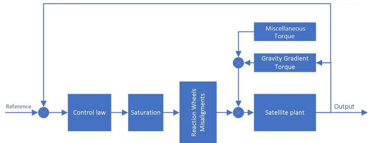
Fig. 3. Block diagram for a CubeSat subject to gravity gradient torque, and misalignment. The control law block may have adaptation algorithms depending on the simulated control law.
