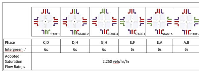
Fig. 5. Adjustment Signal Configuration of Study Site.
