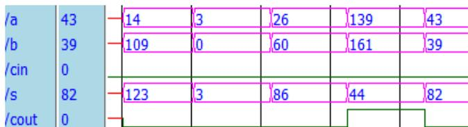
Fig. 7. Carry Save Adder (CSA) Module Simulation Results.
