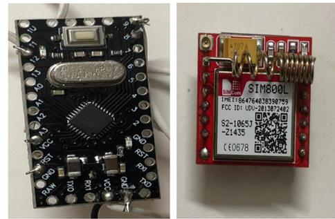
(a) Arduino Pro-Mini. (b) SIM800L Module.
