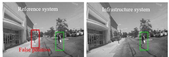
Fig. 16. Left image shows a false positive for the stop sign reported by the reference algorithm, the right image shows the detection result for the same image with no false positive using the infrastructure model
