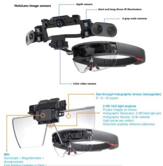
Fig. 1. Sensors on the HOLOLENS.
