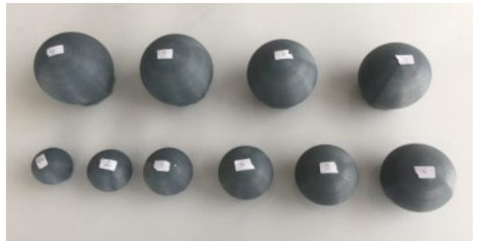
Fig. 8. Set of Different Size PLA Spheres
