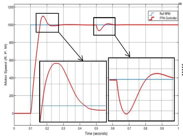
Fig. 8. FPA Speed Controller Output Applying 48V.
