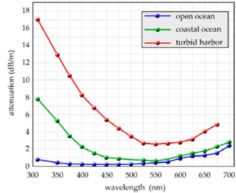
Fig. 6. Attenuation for different Waters [3].
