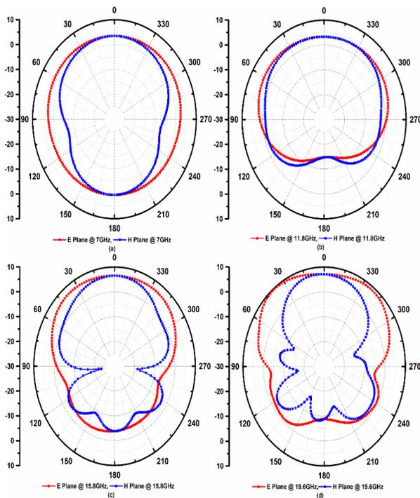
Fig. 7. Radiation Pattern at Azimuth and Elevation Plane of the Proposed Antenna at Multiple Resonances; (a) 7GHz at  $\theta=0^\circ$  and  $\theta=90^\circ$ , (b) 11.8GHz at  $\theta=0^\circ$  and  $\theta=90^\circ$ (c) 15.8GHz at  $\theta=0^\circ$  and  $\theta=90^\circ$ (b) 19.6GHz at  $\theta=0^\circ$  and  $\theta=90^\circ$ .
