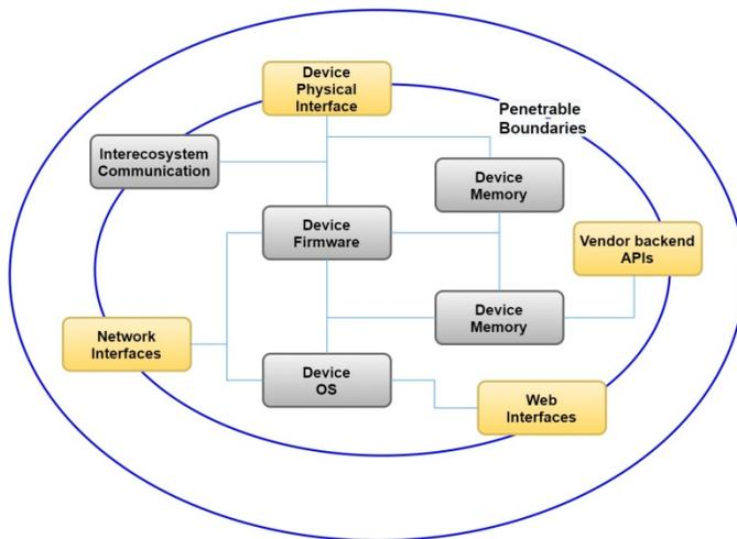
Fig. 3. Attack Surface, and Considered Entry Points, Adapted from [26].
