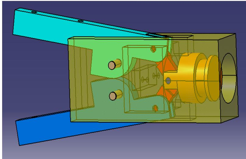
Fig. 13. The Optimal Assembly Solution of the Grip Module.
