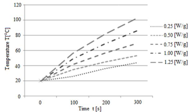
Fig. 6. Values of the Maximum Temperature Calculated in the Mass of the Oat According to Microwave Power at a Processing Time of 300[s].
