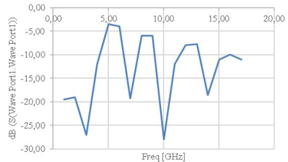
Fig. 5. Reflected Power to the Magnetron S Parameter.
