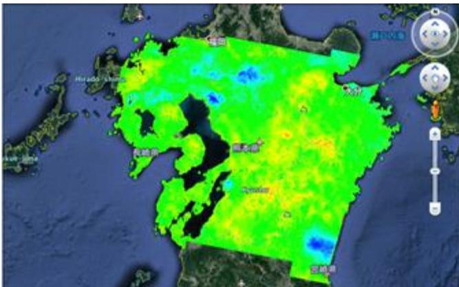
Fig. 8 Interferogram showing elevation changes between two time periods, before and after the Typhoon No.18
