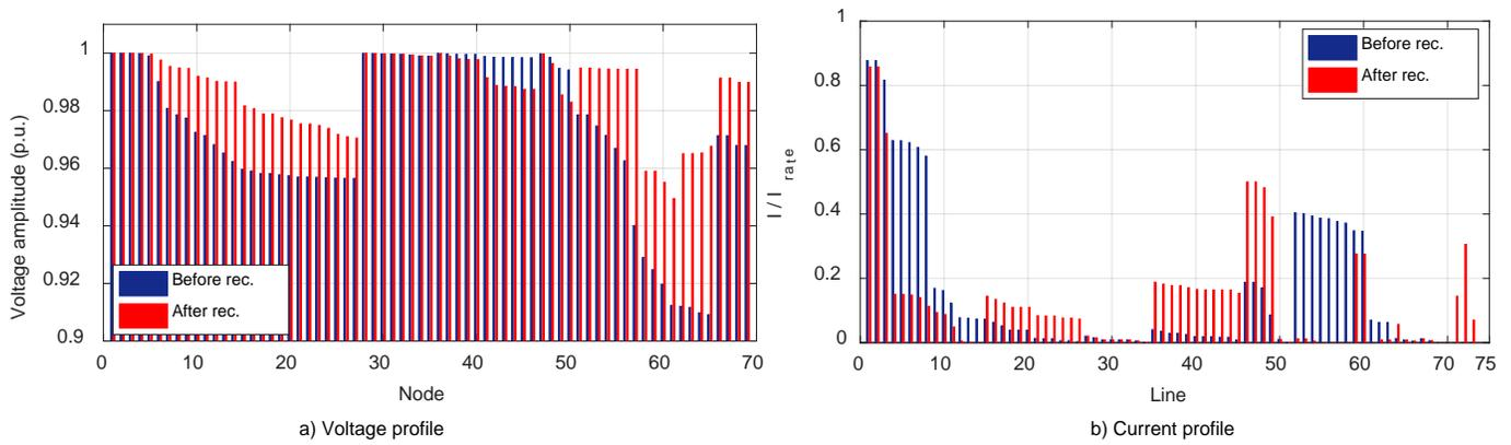
Fig. 3. Voltages and Currents of the 69-Nodes System before and after Reconfiguration.
