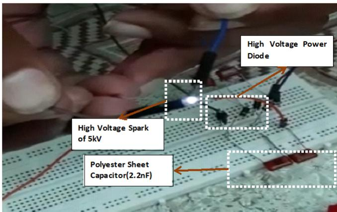
Fig. 13. CWM Design using Polyester Capacitor
