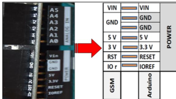
Fig 7. Connect GSM to the Arduino POWER.
