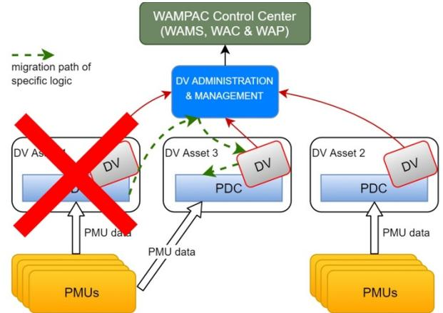
Fig. 10. System State after Migration Process Triggered by a Faulty Connection.
