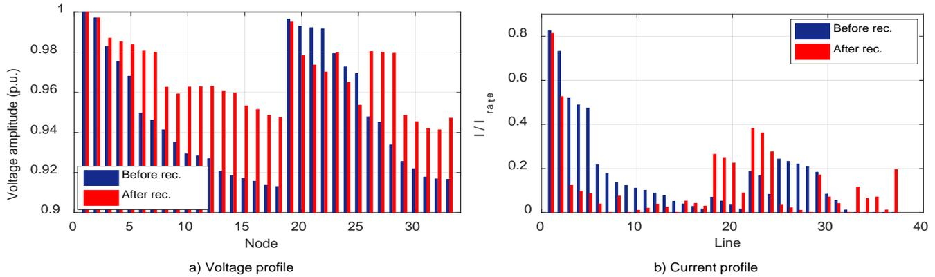
Fig. 2. Voltages and Currents of the 33-Nodes System before and after Reconfiguration.
