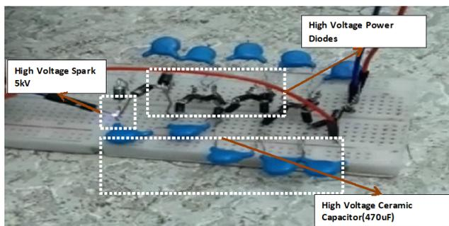
Fig. 14. CWM Design using Ceramic Capacitor
