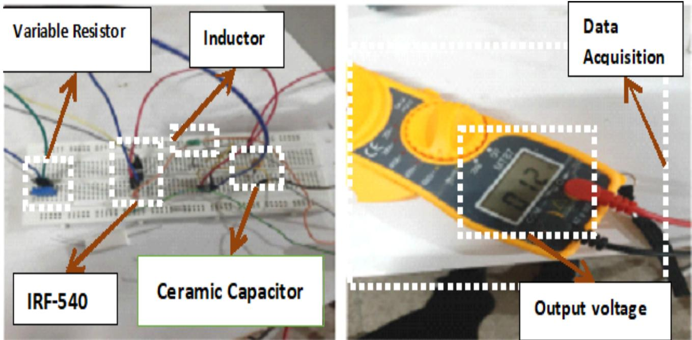
Fig. 12. Experimental Setup of Boost Converter
