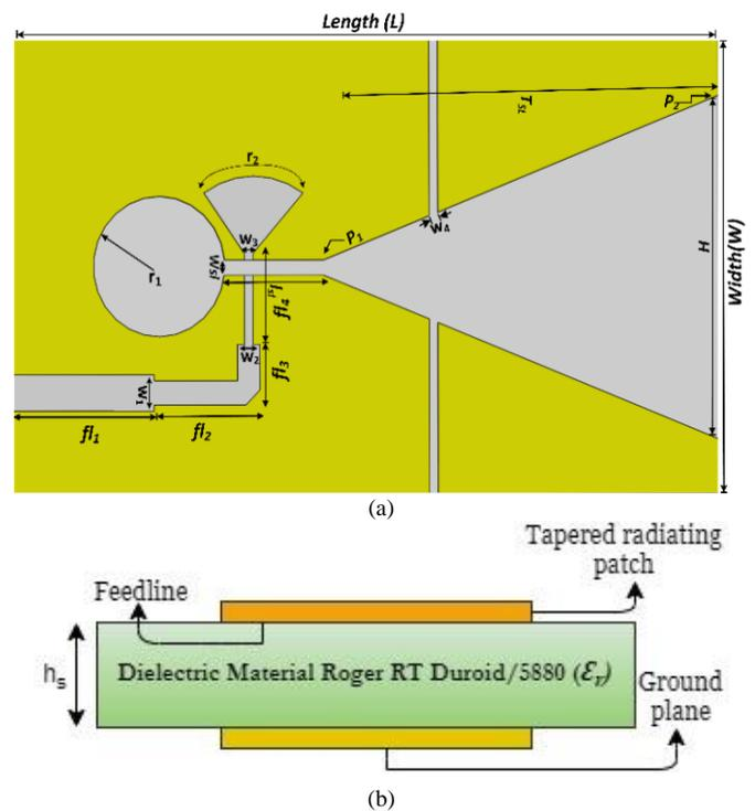
Fig. 1. (a & b) Top and Side view Geometry of the Proposed Antenna.
