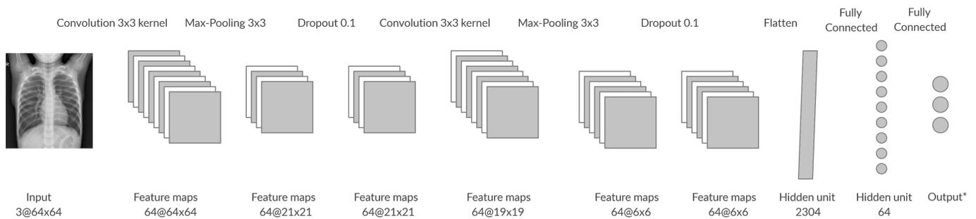
Fig. 2. A Convolutional Neural Networks Architecture for the Classification Tasks. “\*\*” denotes the Number of Output Neurons depends on the Classification Tasks (if the Binary Classification Task needs One Output whereas, for the Classification of Three Classes (the Normal Sample-Viral Pneumonia-Bacterial Pneumonia, the Network Produces Three Output).
