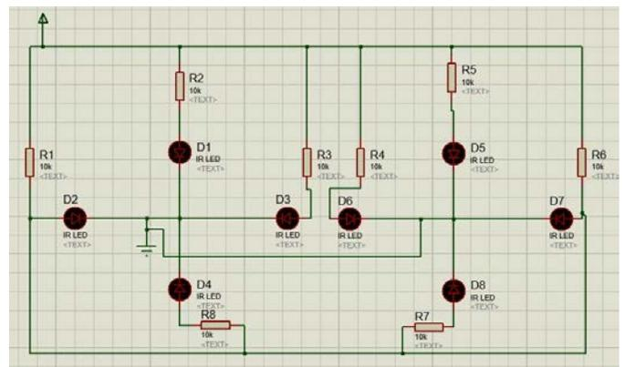
Fig. 2. IR LED Design Schematic for Two Cameras. The IR LEDs are Arranged in Parallel and Placed in Front of the Lens.
