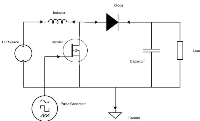
Fig. 1. Boost Converter System
