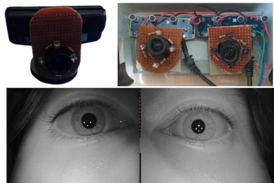
Fig. 1. Customized PS3 Camera with IR LEDs. Single and Double Camera and Captured Image Result from a Double Camera.
