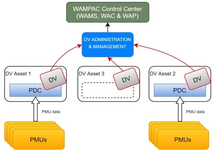
Fig. 9. Grid Monitoring use-case using PMU Measurements with DV Components Integrated.
