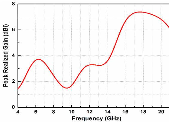
Fig. 6. Simulated Peak Realized Gain Across the Operating Frequency Span.
