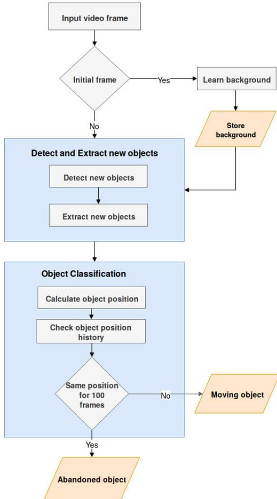
Fig. 2. The Proposed Method Block Diagram. The Method Consists of Input Frames to Build the Background Model. Later the New Object is Detected and Tracked in the Image Scene using Frame Differencing and Background Subtraction. Next, we do Object Classification whether the Object is Moving or Static based on Computing the Object Position History. Finally, we Mark or Declare the Static Object as the Left Luggage or Abandoned Baggage based on the Position History.
