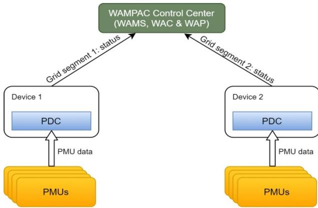
Fig. 8. Simple Grid Monitoring use-case using PMU Measurements.
