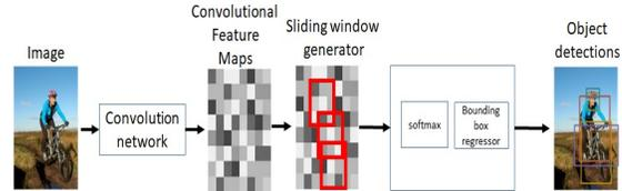
Fig. 1. Faster R-CNN Generates Anchors of Different Ratios and Scales for each Sliding Windows on Convolutional Feature Map. After that, the Output of Regressor Determines a Predicted Bounding Box.
