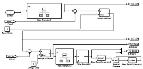
Fig. 3. The FPA based Controller for BLDC.
