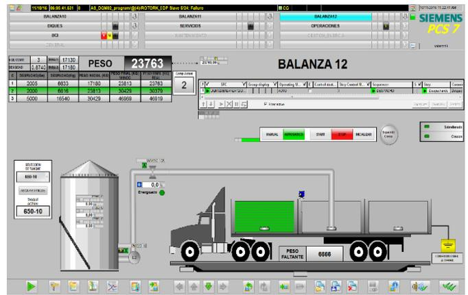
Fig. 16. Commissioning of the SCADA System: Filling Process of Container 2 of the Tank Truck.
