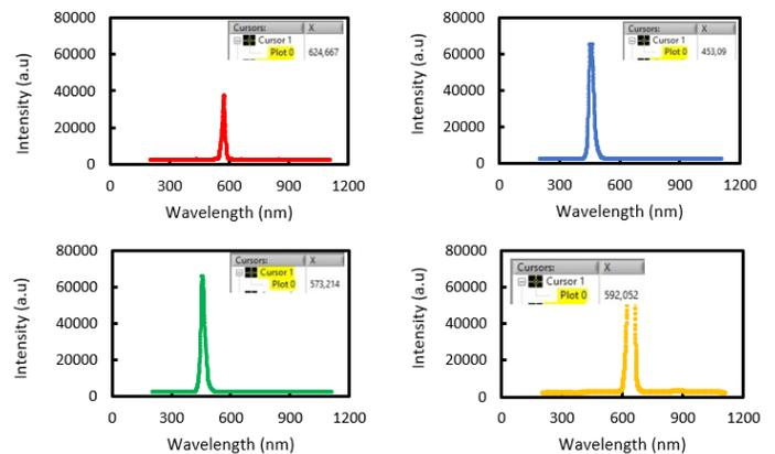
Fig. 7. The Various Wavelength on the Red, Blue, Green and Yellow LED.
