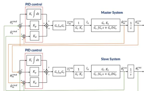
Fig. 6. General Block Diagram for a Bilateral Robotic Arm with Two Separate Subsystems.
