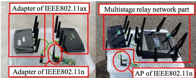
Fig. 10. Device of IEEE802.11n and IEEE802.11ax. (Left : SN, Right : Mobile Robot).
