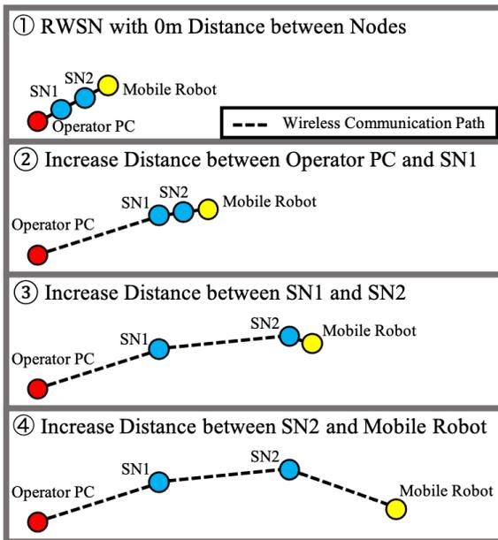
Fig. 2. Increasing Distance between Nodes while Maintaining Communication Connectivity in RWSNs.
