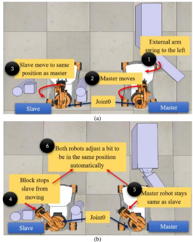
Fig. 9. (a) and (b). Overall view and Operation Steps for the Bilateral Control System.
