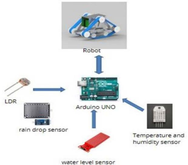
Fig. 6. Pictorial Representation of all the Sensors Carried by the UGV.
