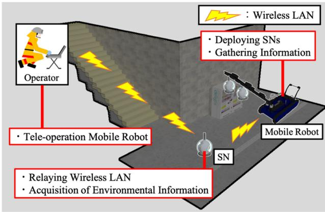
Fig. 1. Gathering Information by Mobile Robot (Robot Wireless Sensor Networks : RWSN).
