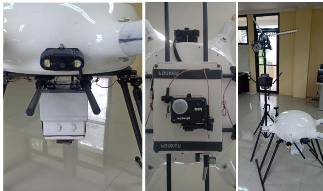
Fig. 14. Installed Prototype as Payload underneath the Drone.
