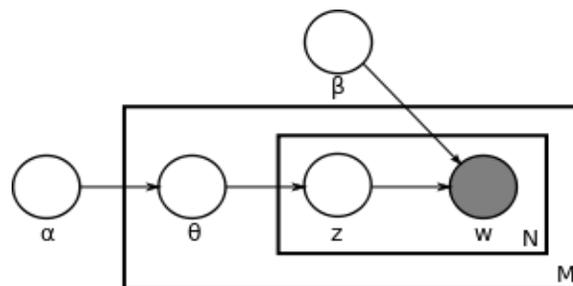
Fig. 4. Plate Notation Visualizing the LDA Model Parameters, Plate M Represent The Total Number of Documents, N Represent the Numbers of Terms in a Document,  $\alpha$  the Per-Document Topic Distributions,  $\beta$  the Per-Topic Word Distribution,  $\theta$  the Topic Distribution For Document m, z the Topic for the n-th Word, w is a Specific Word.
