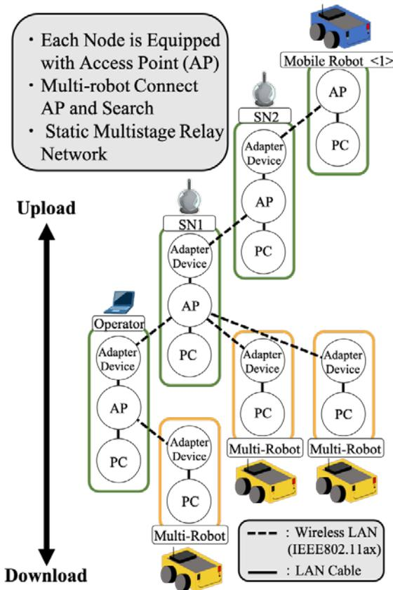
Fig. 5. Network Topology of Multi-robot System.
