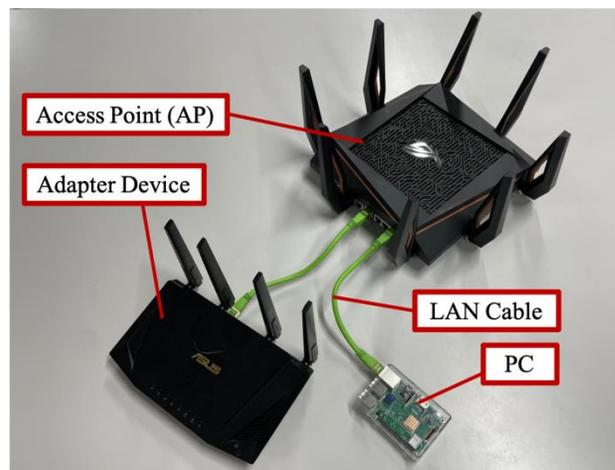
Fig. 5. Device of a Node Constituting the Multistage Relay Network.
