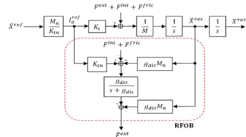
Fig. 3. A Block Diagram for RFOB based on an Open-Loop Control System.
