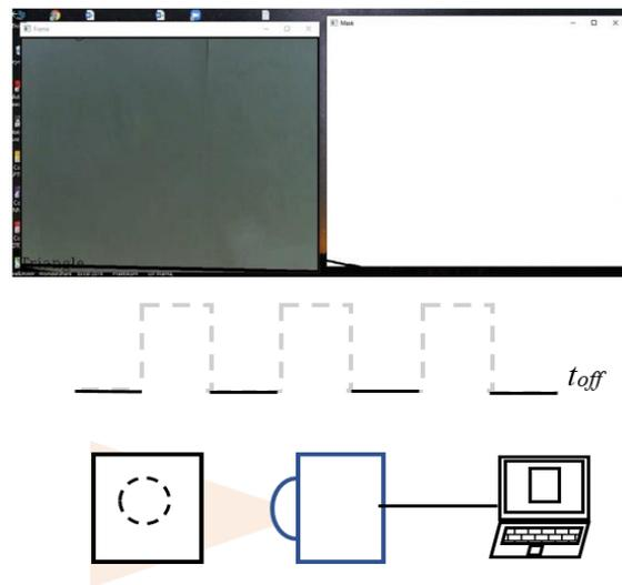
Fig. 10. In the  $t_{off}$  Condition, the Marker is not Captured All the Time by the Camera.
