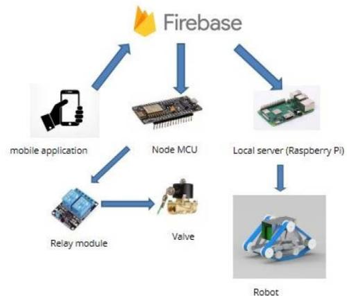
Fig. 10. Pictorial Representation of the Mobile Application-based Control System.
