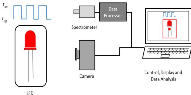
Fig. 1. Encoding LED Blinking Mechanism. A Camera Captured the Display of LED, and a Spectrometer Captured the PWM Signal.
