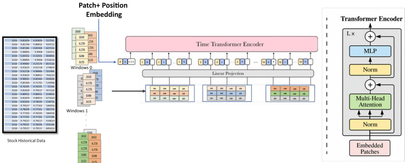
Fig. 2. Proposed Transformer Encoder Model Overview (Illustration Inspired by [22]).
