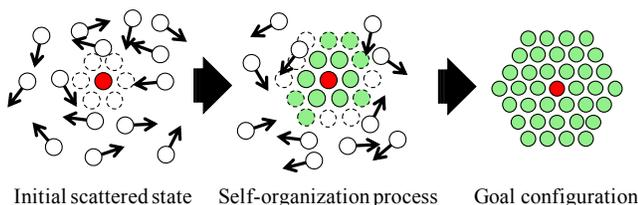
Fig. 1. Self-organizing a Regularly Arranged Group from Scattered Robots.
