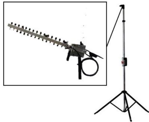
Fig. 6. A 2.5 Meters Tripod Stand where the Wi-Fi Dongle, Yagi.
