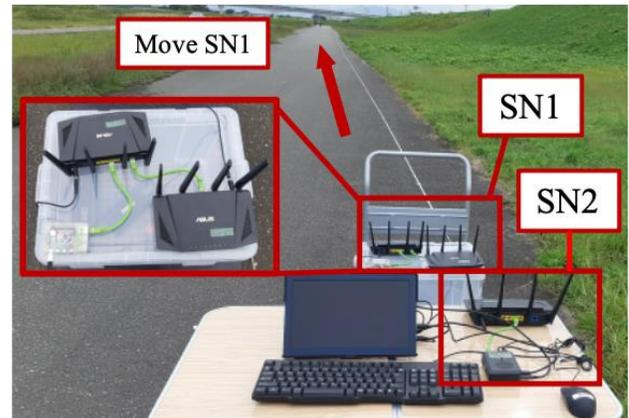
Fig. 8. Experimental Environment; Increase in Distance between Nodes.
