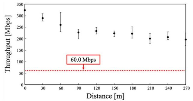
Fig. 12. Throughput of Upload between Operator PC and Mobile Robot <1> in Triple-hop Multistage Relay Network.
