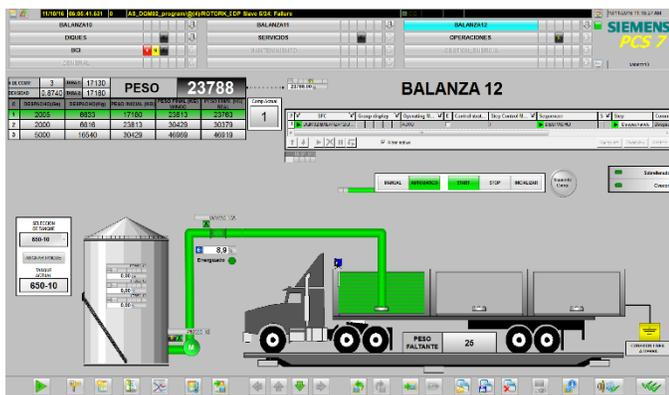
Fig. 14. SCADA System Start-Up: Filling System Control, Valve Restriction to 85%.
