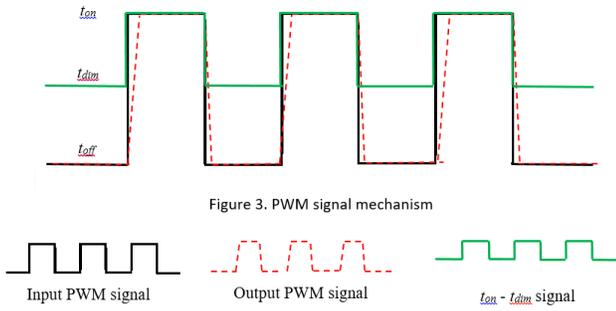
Figure 3. PWM signal mechanism
