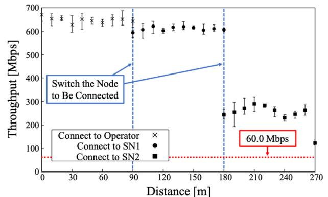
Fig. 15. Throughput of Download between Operator PC and Mobile Robot during Mobile Robot Teleoperation.
