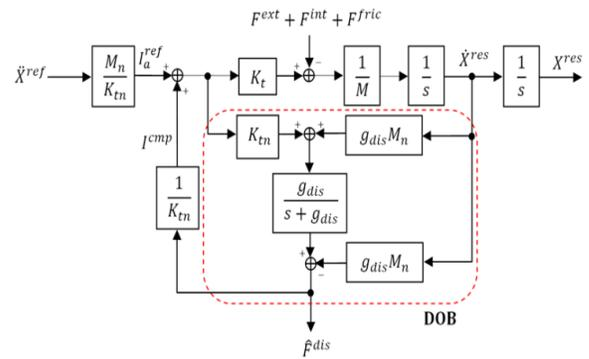
Fig. 1. A Block Diagram for a DOB based Open-loop Control System.
