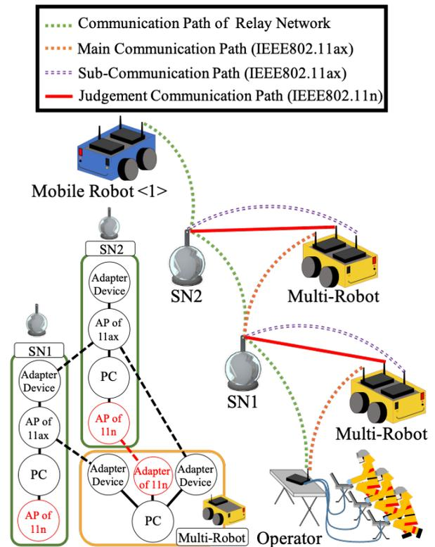
Fig. 7. Method for Changing Communication Path while Maintaining Communication Connectivity for Mobile Robots.
