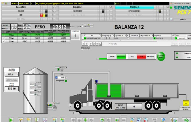
Fig. 15. Commissioning of the SCADA System: Complete Filling of Container 1.
