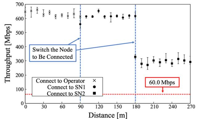
Fig. 14. Throughput of Upload between Operator PC and Mobile Robot during Mobile Robot Teleoperation.
