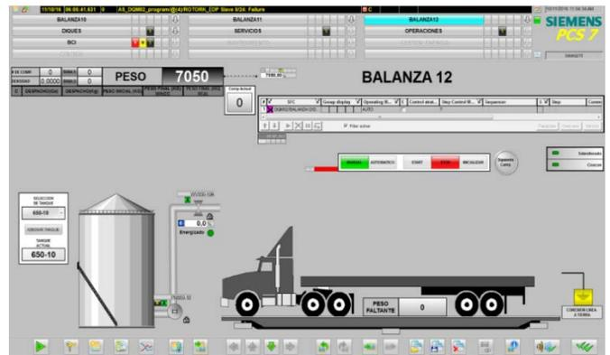
Fig. 11. Configuration of the Tank Selection and Start of the Dispatch Process, in the SCADA System.
