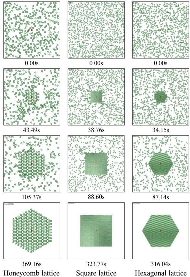
Fig. 7. Group Enlargements up to Self-organization of 15-layer Robot Groups on Different Lattice Types.
