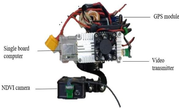
Fig. 9. HD Wireless Video Transmitter System with Installed NDVI Camera and GPS Module.
