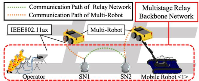
Fig. 3. Gathering Information by Multi-robot using Multistage Relay Network.
