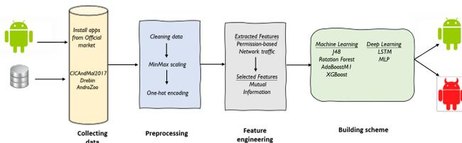
Fig. 1. Architecture of the Implemented Scheme.
