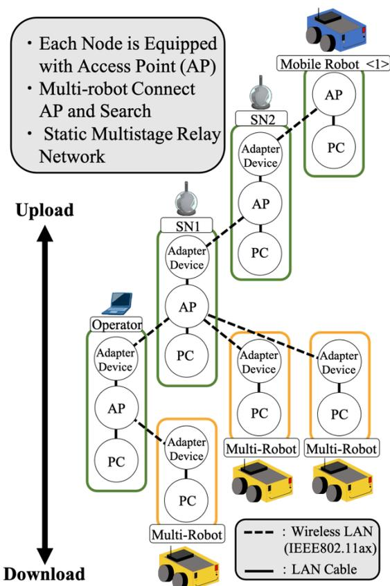
Fig. 4. Proposed Topology for Constructing a Multi-robot Environment.
