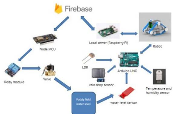
Fig. 11. Pictorial Representation of the Independent Cloud-based Control System.
