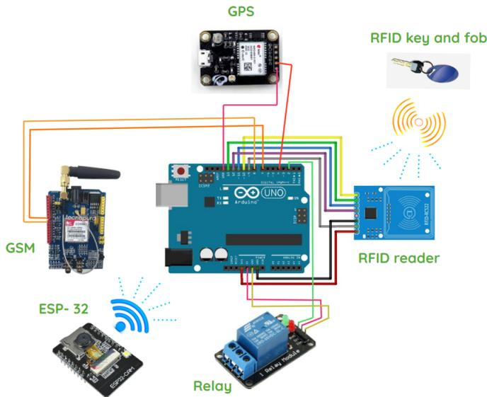
Fig. 3. Physical Diagram of the Anti-theft System.
