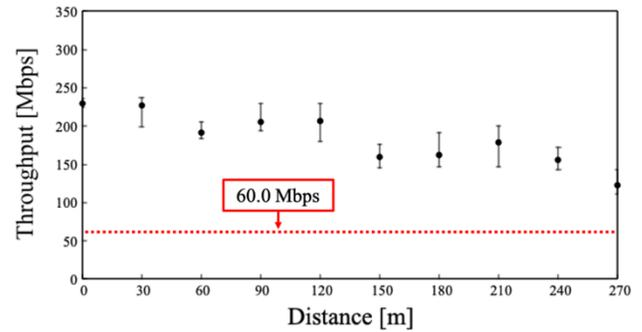
Fig. 13. Throughput of Download between Operator PC and Mobile Robot <1> in Triple-hop Multistage Relay Network.
