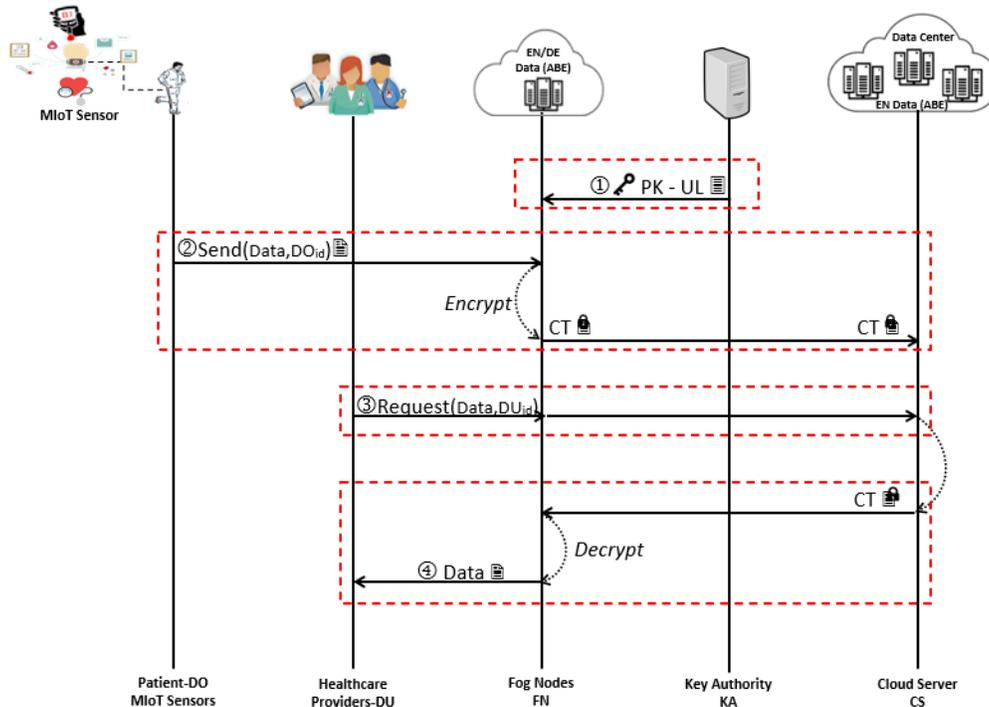
Fig. 2. System Workflow.
