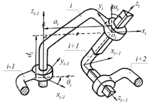
Fig. 4. Denavit-Hartenberg Compatible Coordinate Systems.
