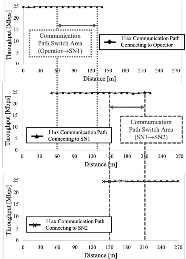
Fig. 12. Throughput between Operator and Mobile Robot. ( Top : Mobile Robot Connecting to Operator, Middle : Mobile Robot Connecting to SN1, Bottom : Mobile Robot Connecting to SN2).
