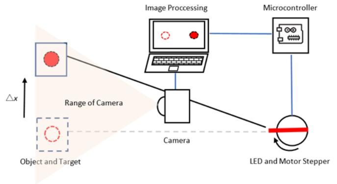
Fig. 2. Object Recognition System consists of the Camera, Image Processing, LED as a Marker Embedded to the Servo Motor and Microcontroller.
