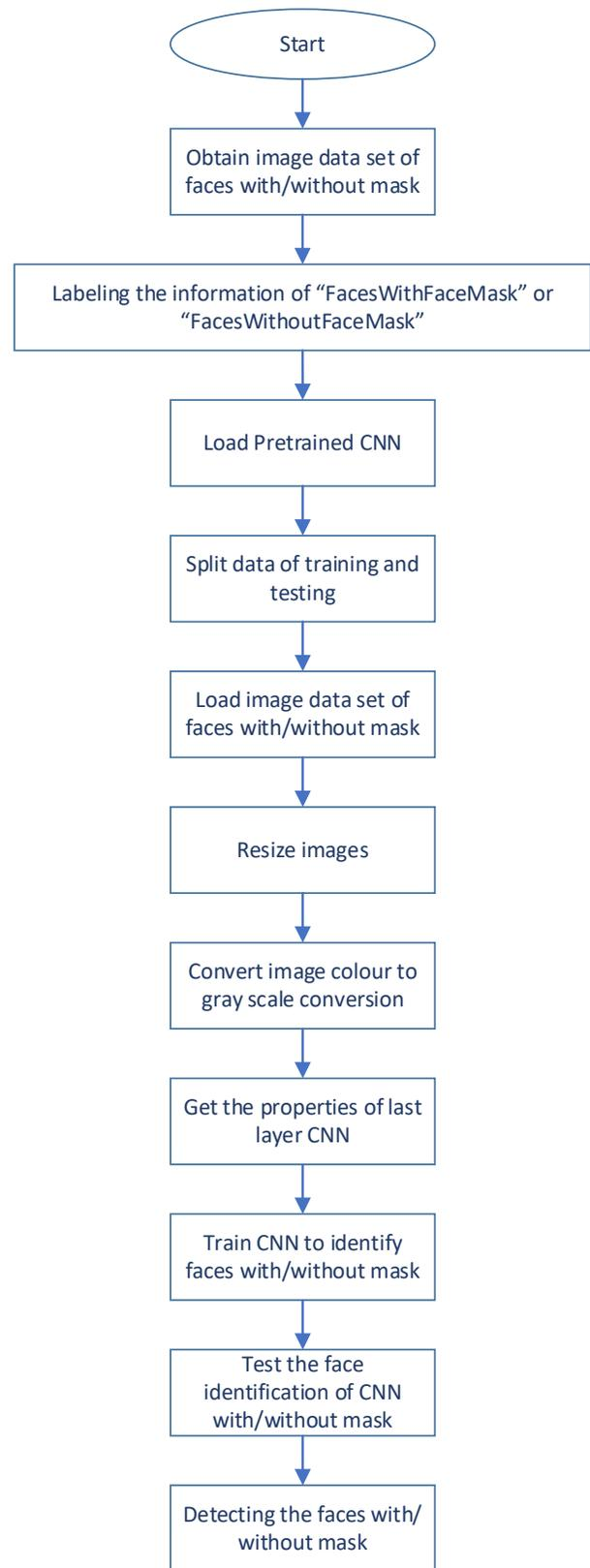
Fig. 9. Process Flow for the Transfer Learning.
