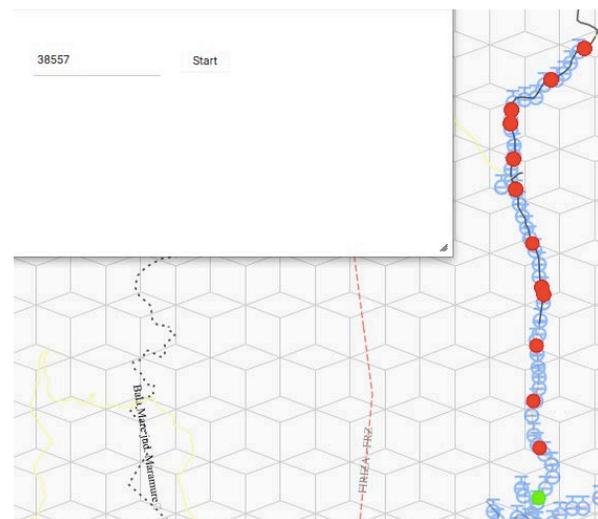
Fig. 9. Example of the Valves that Needs to be Closed for Node 38557.
