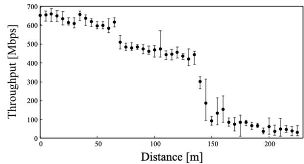
Fig. 9. Throughput of Upload; Increase in Distance between Nodes.
