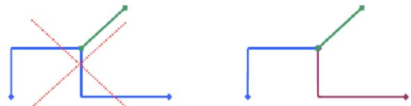
Fig. 1. Example of How to Break Pipes at Intersections in QWAT Databases.
