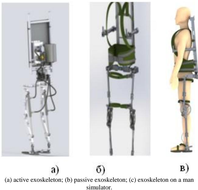
Fig. 1. D-model of Active and Passive Exoskeleton.
