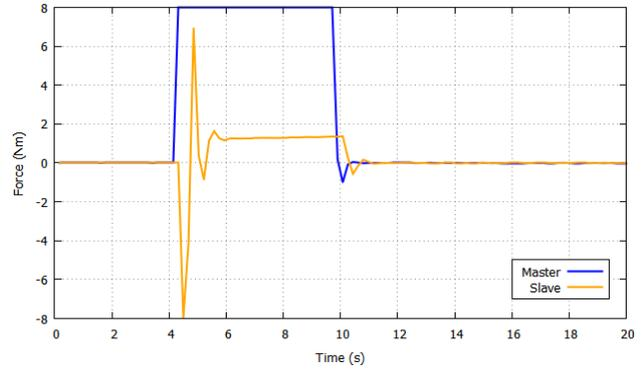
Fig. 10. Generated Force on both Subsystems across Period for  $\omega_n = 1$ .
