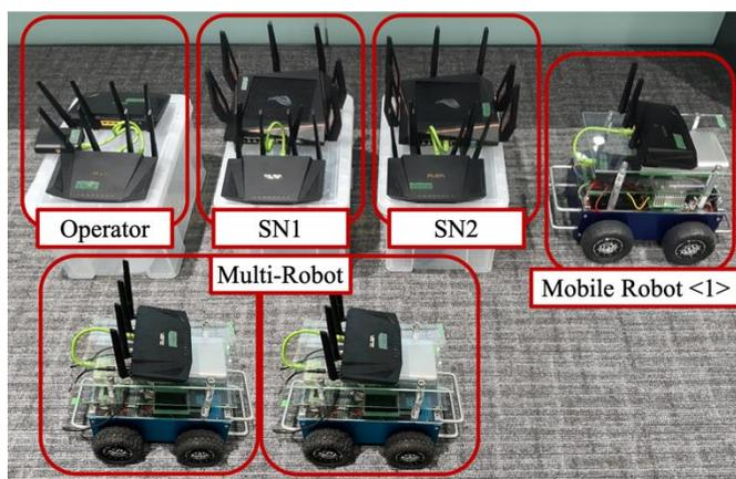
Fig. 6. Multistage Relay Network and Robots.
