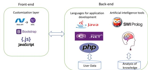
Fig. 2. Development Architecture Diagram.
