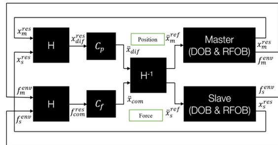
Fig. 5. A Simplified Block Diagram of Master-Slave Bilateral Control System with Proposed Tools.
