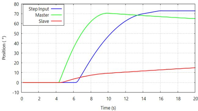
Fig. 21. Position Tracked on both Subsystems across the Period for  $\omega_n = 5$ .
