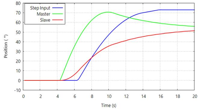
Fig. 23. Position Tracked on both Subsystems across the Period for  $\omega_n = 20$ .
