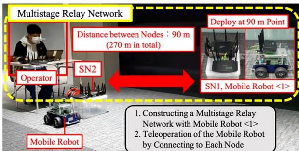
Fig. 11. Experimental Environment, Construction of Multistage Relay Network and Teleoperation of Mobile Robot.
