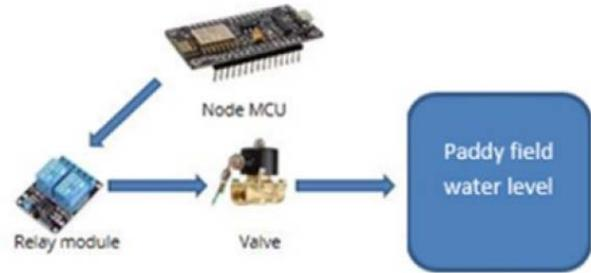
Fig. 4. Pictorial Representation of the Valve System for Paddy Cultivation.
