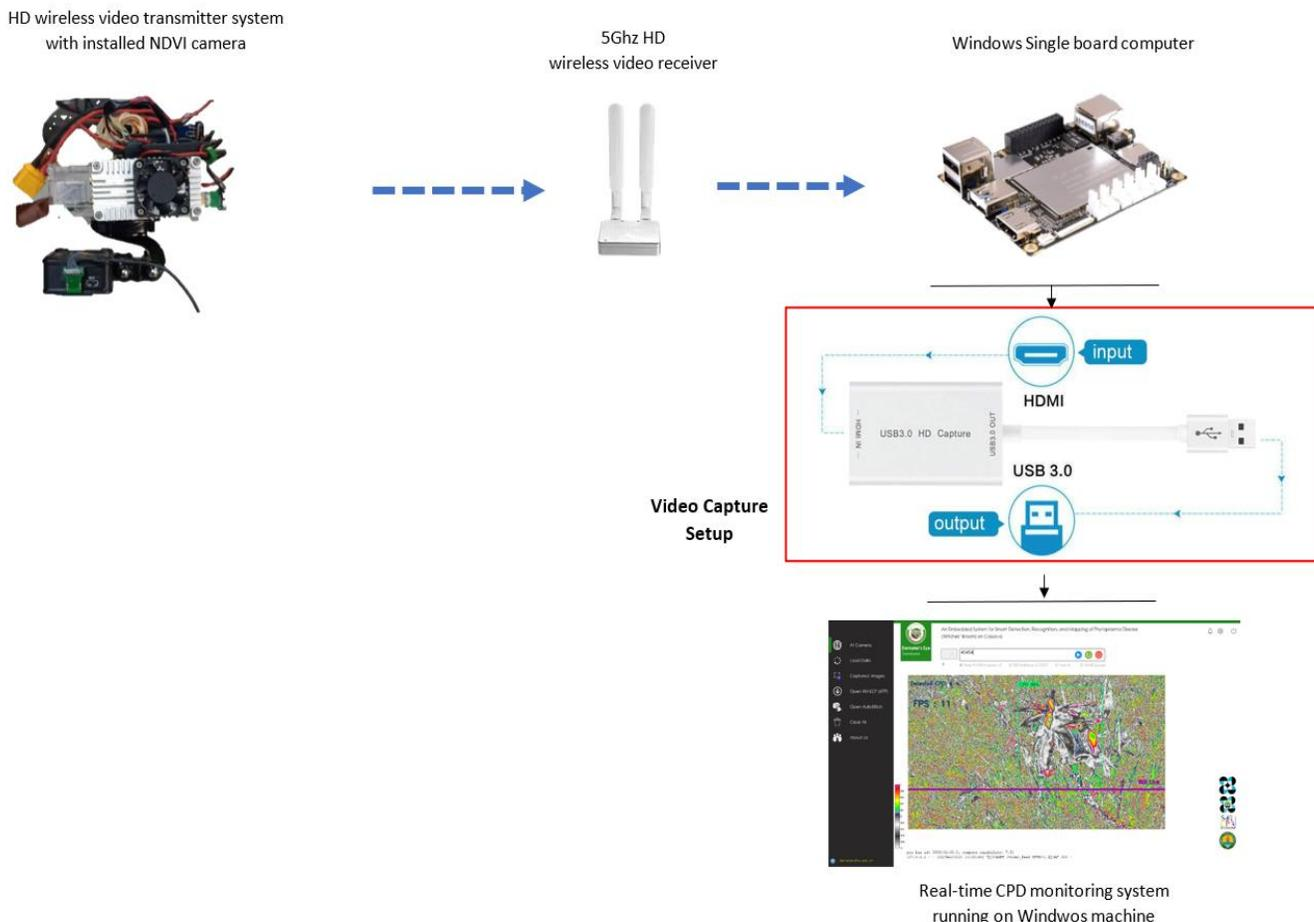
Fig. 8. Video Capture System Layout.
