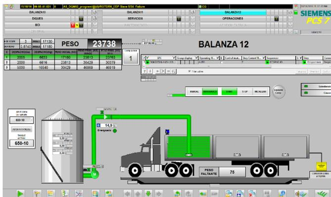
Fig. 13. SCADA System Commissioning: Filling System Control, Valve Restriction to 75%.
