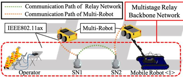
Fig. 2. Multi-Robot System using Multistage Relay Network.
