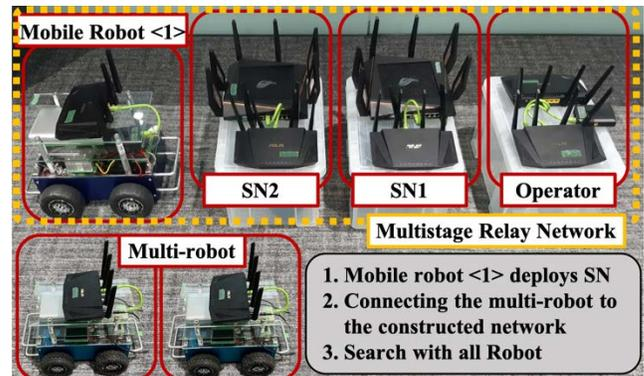
Fig. 4. Device of each Node that Constitutes Multi-robot System.
