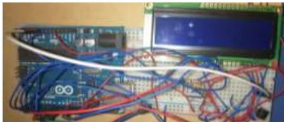
Fig. 3. Breadboard with Arduino and LCD Screen Wired
