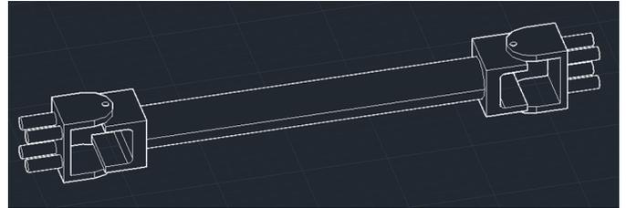
Fig. 7. DustyTRON 3 Proposed Steering System.
