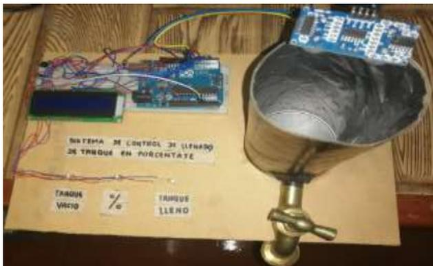
Fig. 5. Water Monitoring System
