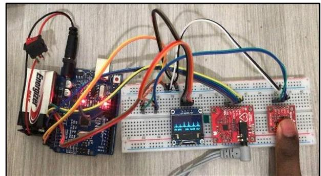
Fig. 18. CKD Monitoring System Hardware.
