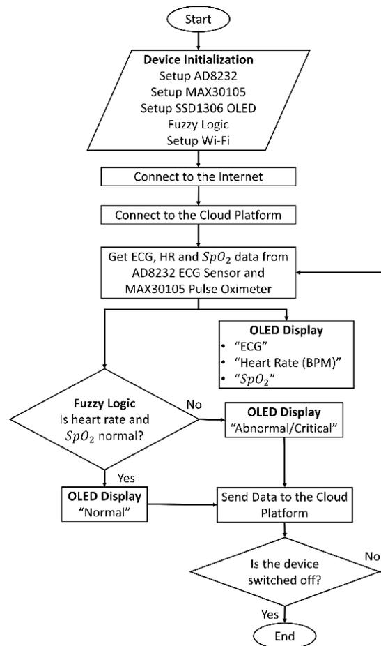
Fig. 17. Flowchart of the Microcontroller Program.
