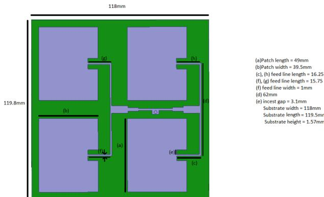
Fig. 4. 4-Element Rectangular Antenna Array
