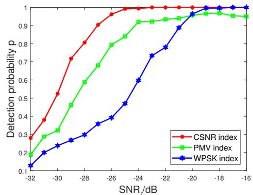
Fig. 5. The Single Frequency Signal Detection Probability by SR Systems with Different Indexes and Different Input Signal-to-Noise Ratios, where the Red, Green and Blue Curves are the Detection Probability with the CSNR, PMV and WPSK Indexes, respectively.
