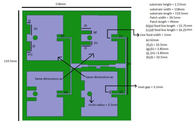
Fig. 6. 4-Element Modified H Shaped Patch Antenna Array
