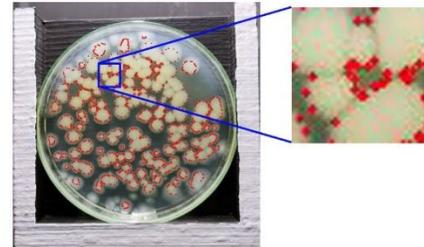
Fig. 16. An Example of a Gap inside a Colony Group, which Causes Creation of Inadvertent Extra PIDs that Disrupt the Formula for Counting Colonies.
