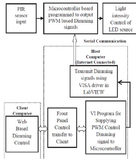
Fig. 3. System Block Diagram for Intelligent Dimmer Circuit.
