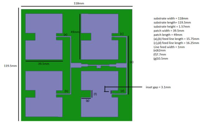
Fig. 5. 4-Element H-Shaped Patch Antenna Array
