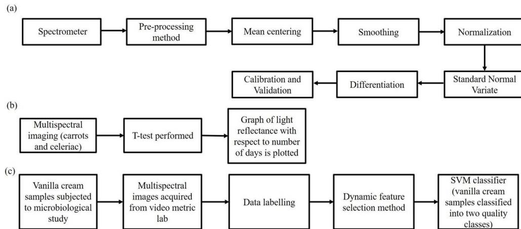
Fig. 6. Block Diagram for Fruit Quality. (a) Chemometric Block Diagram to Extract the Information of Pomegranate Fruit. (b) Block Diagram to Calculate Optical Reflection Changes in Carrots and Celeriac using Multispectral Imaging. (c) Block Diagram of SVM Classifier to Classify Vanilla Cream Samples in Two Quality Classes.
