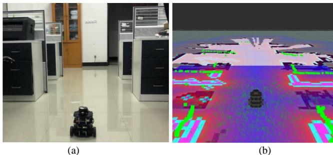
Fig. 6. (a) Robot's Environment in Laboratory (b) Green Squared Dots Represent LIDAR Measurements Readings. Turtlebot Real EKF Implementation under ROS Robot Operating System.
