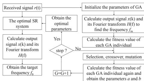
Fig. 3. The Frequency Detecting Process of SR System.
