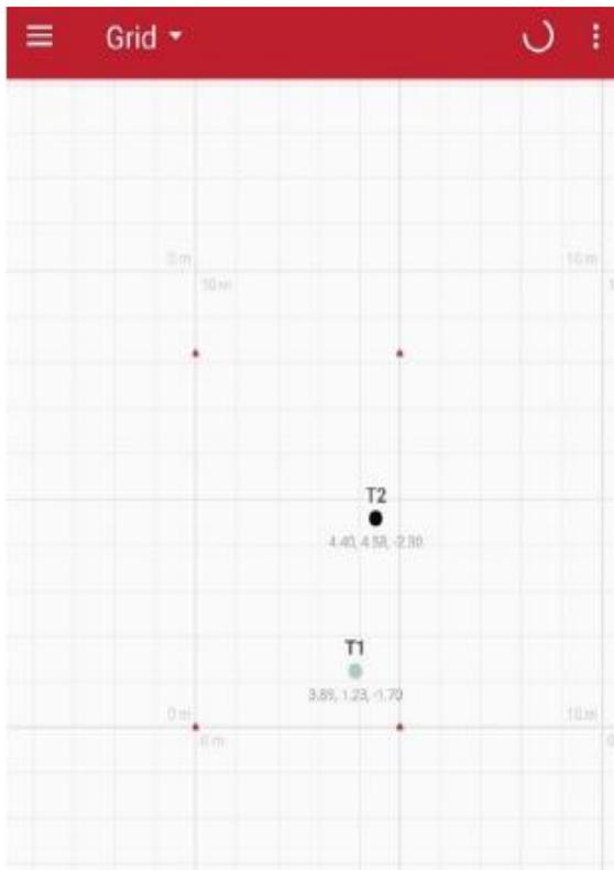
Fig. 6. DRTL Application showing the Location of the 2 Tags in the Room.
