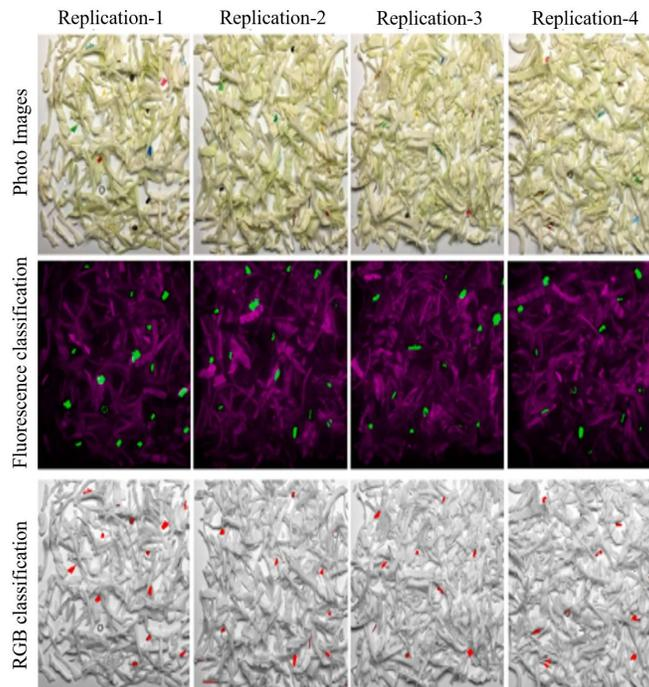
Fig. 19. Colour Images of Cabbage Samples Mixed with Foreign Materials (FM) are shown in the Top Row. Classification Images based on Fluorescence are shown in the Middle Row. Classification Images based on RGB are shown in the Bottom Row [20].
