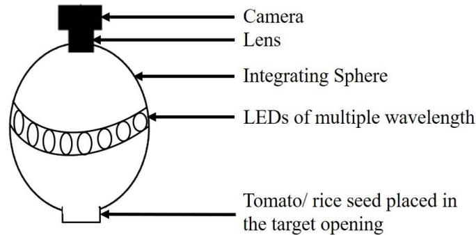
Fig. 4. Structural Setup for Capturing Multispectral Images using the VideometerLab Instrument [8].
