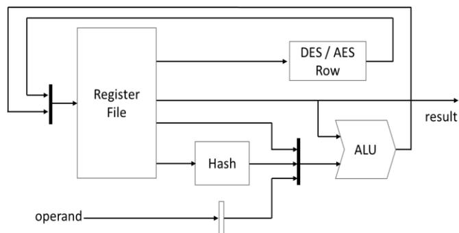
Fig. 1. Block Diagram of the CAU Module [22].
