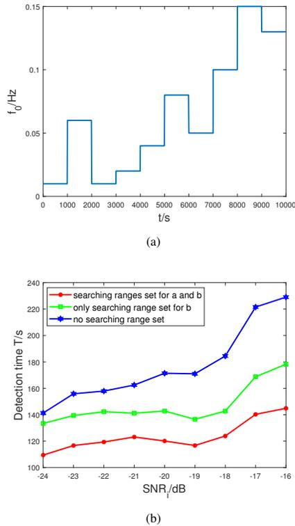
Fig. 9. (a) The Frequency of Original Frequency-Hopping Signal. (b) With the different Searching Ranges of Parameters  $a$  and  $b$ , the Frequency-Hopping Signal Detection Time by SR System with the CSNR Index.
