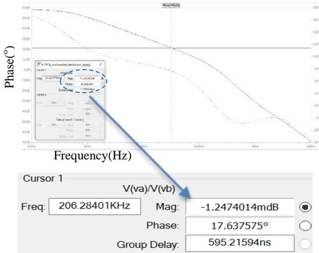
Fig. 9. Phase Margin Results using the Noninvasive Method.
