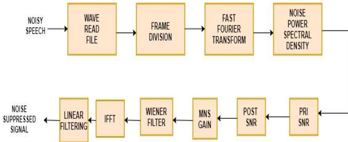
Fig. 3. Modified Noise Reduction Method in DHA.
