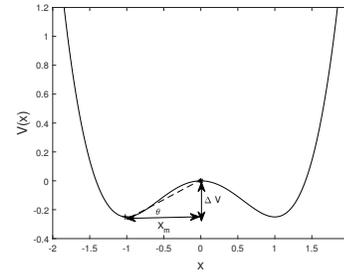
Fig. 1. The Potential Function Curve of  $V(x)$ , when  $a = b = 1$ .  $\Delta V$  is the Potential Height,  $x_m$  is the Half Width of Potential well,  $\tan \theta = \Delta V/x_m$ .
