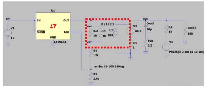
Fig. 5. LVR Circuitry for Noninvasive Stability Measurement.
