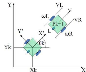
Fig. 2. Real Robot and its Kinematic Model.
