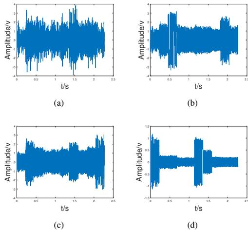
Fig. 13. The Signal in Time Domain. (a) Frequency-Hopping Signal  $s$ , (b) the Output Signal with no Searching Range Set, (c) the Output Signal with Searching Range Set for Parameter  $b$  only, (d) the Output Signal with Searching Ranges Set for Parameters  $a$  and  $b$ .
