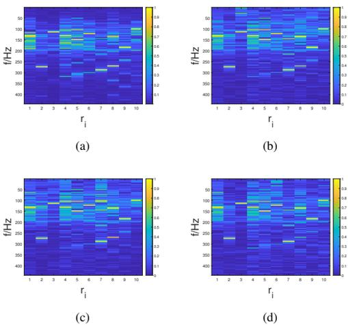
Fig. 14. The Signal in Time-Frequency Spectrum. The X-Label Represents Signal  $r_i$  ( $i = 1 \dots 10$ ) and Y-Label Represents the Output Signal Frequency (from 0 to 500 Hz). (a) Frequency-Hopping Signal  $s$ , (b) the Output Signal with no Searching Range Set, (c) the Output Signal with Searching Range Set for Parameter  $b$  only, (d) the Output Signal with Searching Ranges set for Parameters  $a$  and  $b$ .
