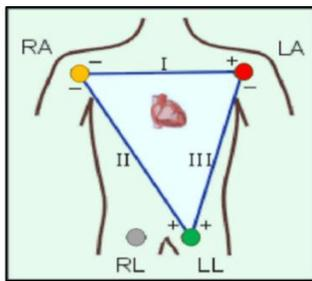
Fig. 20. Einthoven's Triangle for ECG Lead Placement [40].
