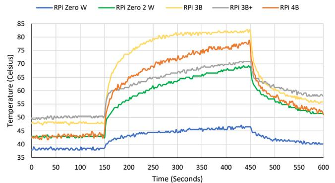
Fig. 3. Results of Stressberry for Different RPi Models.
