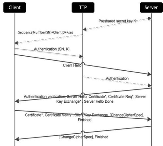
Fig. 3. Communication in the E-Lithe Scheme [8].
