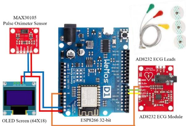
Fig. 16. Wiring Diagram of the Implemented Hardware using ESP8266.
