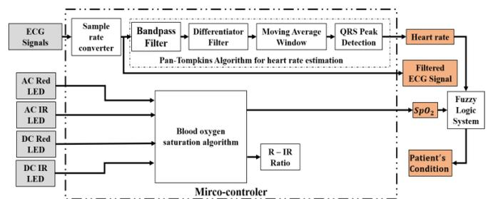
Fig. 5. Block Diagram of Proposed CKD Monitoring System.
