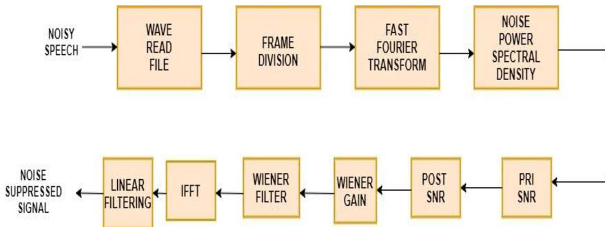
Fig. 2. Noise Reduction by Wiener Filter in DHA.
