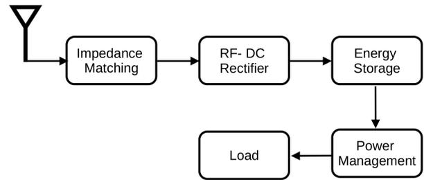
Fig. 1. Typical Block Diagram Representation of RF Energy Harvesting System.
