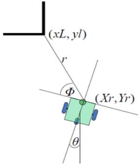
Fig. 3. Robot Pose from the Landmark.
