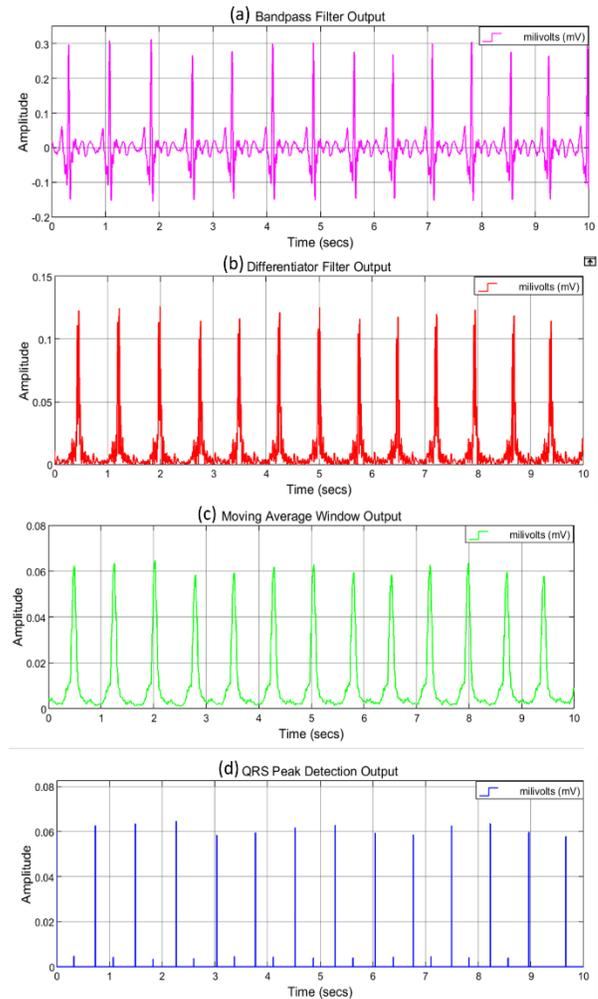
Fig. 8. Phases in Digital Signal Processing and QRS Peak Detection a. Bandpass Filter Output. b. Differentiator Filter Output. c. Moving Average Window Output. d. QRS Peak Detection Output.
