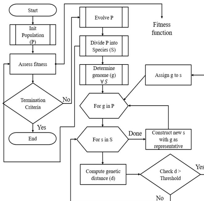
Fig. 3. Flow Process of Topology Augmentation using NEAT.
