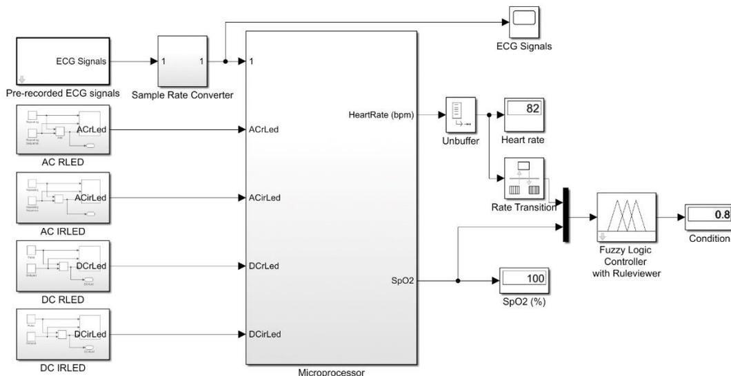
Fig. 6. Simulink Model of CKD Monitoring System.
