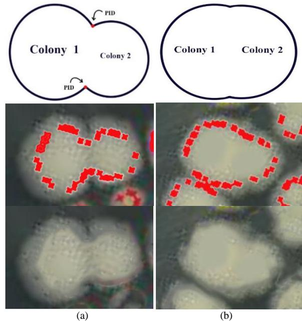
Fig. 17. Examples of Overlapping Colonies in which (a) the Perimeters are Sufficiently Distinguishable to Generate PIDs and be Counted Correctly and (b) the Perimeters are too Similar to Generate PIDs and an Undercount can occur.
