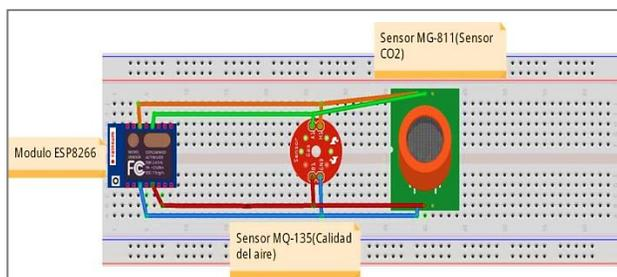
Fig. 2. Prototype Design.
