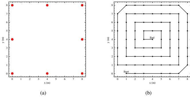
Fig. 3. (a) Wi-Fi Reference Points marked as Red (b) User Route where Black Marks Indicate Locations of RSSI Measurements
