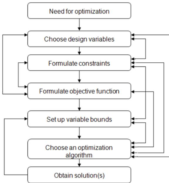
Fig. 5. Representing the Optimization Flow Diagram.
