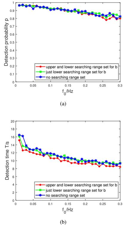
Fig. 8. With the Different Searching Ranges of Parameter  $b$ , the Single Frequency Signal Detection Probability and Detection Time with CSNR Index and Different Signal Frequencies.
