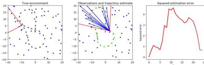
Fig. 5. True Robot Trajectory (Left), Estimated Trajectory (Middle) and Squared Positional Error (Right) using EKF Algorithm.
