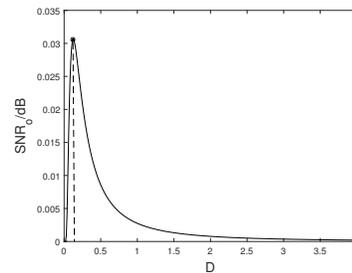
Fig. 2. The Curve of  $SNR_o$  with Noise Intensity  $D$ , when  $A = 0.1$ ,  $a = b = 1$ .
