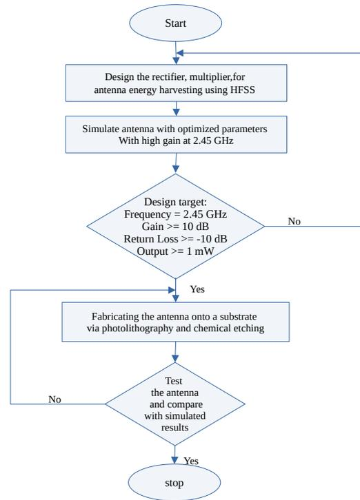
Fig. 3. RF Energy Harvesting Antenna Design Flow
