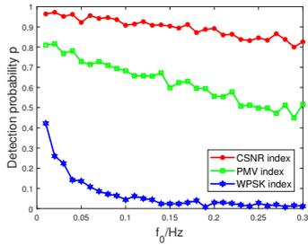
Fig. 6. The Single Frequency Signal Detection Probability by SR Systems with Different Indexes and Different Signal Frequencies, where the Red, Green and Blue Curves are Detection Probability with the CSNR, PMV, and WPSK Indexes, respectively.
