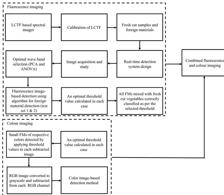
Fig. 12. Block Diagram for Detection of Foreign Material in Cabbage and Green Onion Samples using Reflectance and Fluorescence Images.
