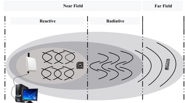
Fig. 2. Three Categories of WPT. Near Field, Far Field - Directional, and Far-Field Ambient Wireless Energy Harvesting
