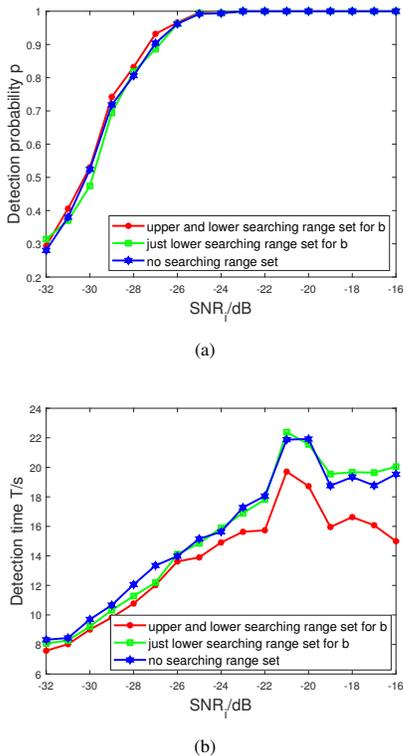
Fig. 7. With the Different Searching Ranges of Parameter  $b$ , the Single Frequency Signal Detection Probability and Detection Time with CSNR Index and Different Input Signal-to-Noise Ratios.
