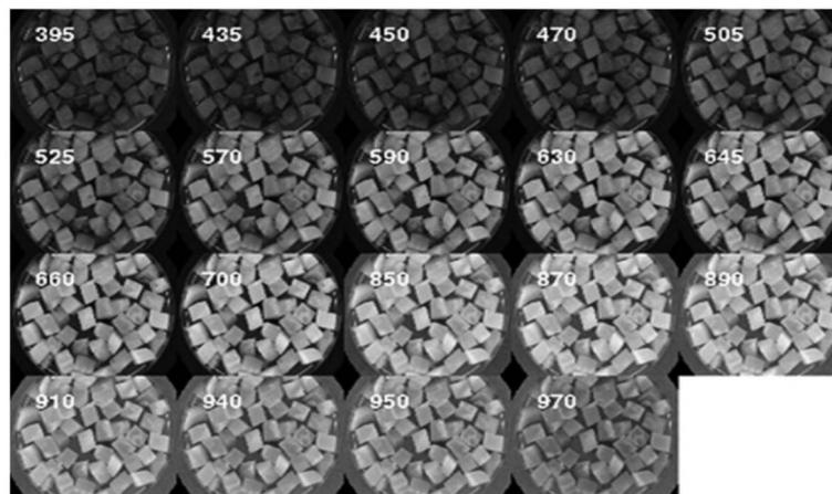
Fig. 5. Plot showing All Spectral Channels of a Celeriac Sample [9].
