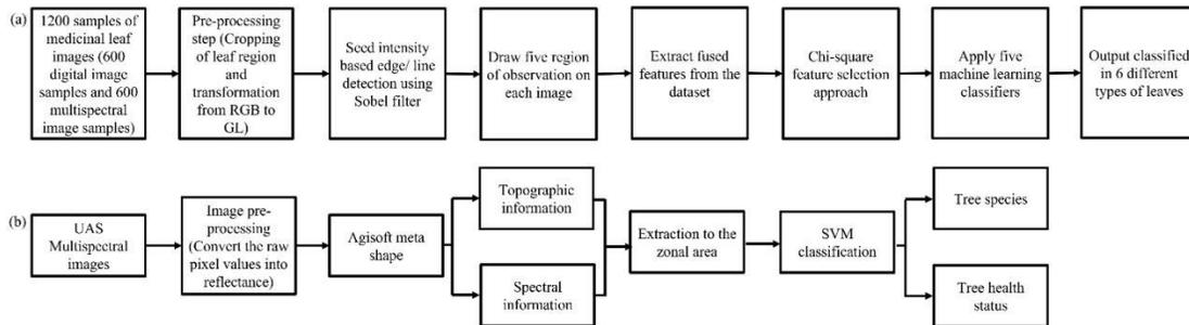
Fig. 11. Different Classification Strategies using Multi-Spectral Imaging on the Plant Data. (a) Block Diagram for Medicinal Plant Leaves Classification. (b) Block Diagram of Disease Detection in Tree Species to Recognize Healthy, Unhealthy and Dead Trees Affected by Bark Beetle Infection.
