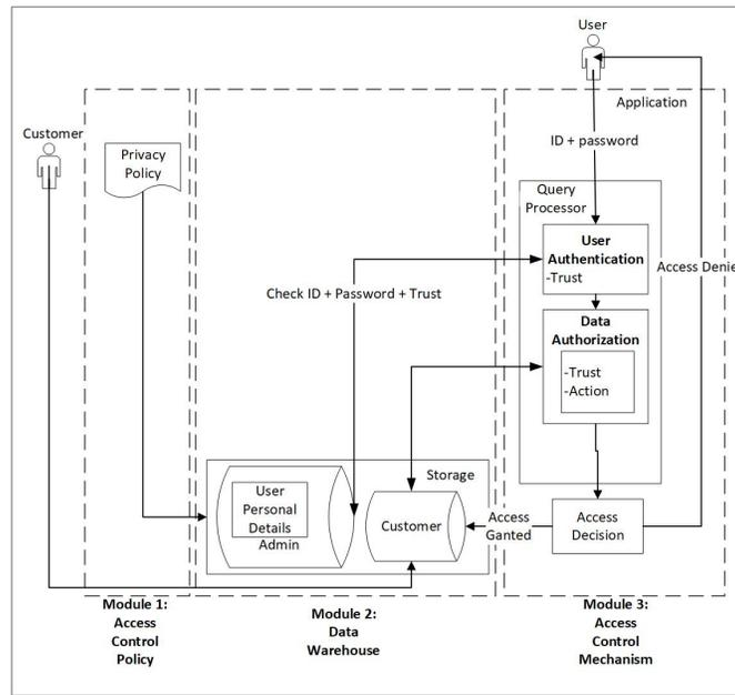
Fig. 2. The Proposed Trust-Based Access Control Model Framework
