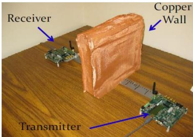
Fig. 7. Copper Wall Obstacle, Receiver and Transmitter.
