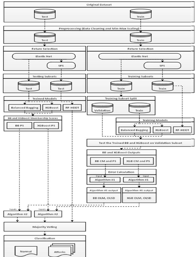
Fig. 2. Classifier Development Schematic Diagram
