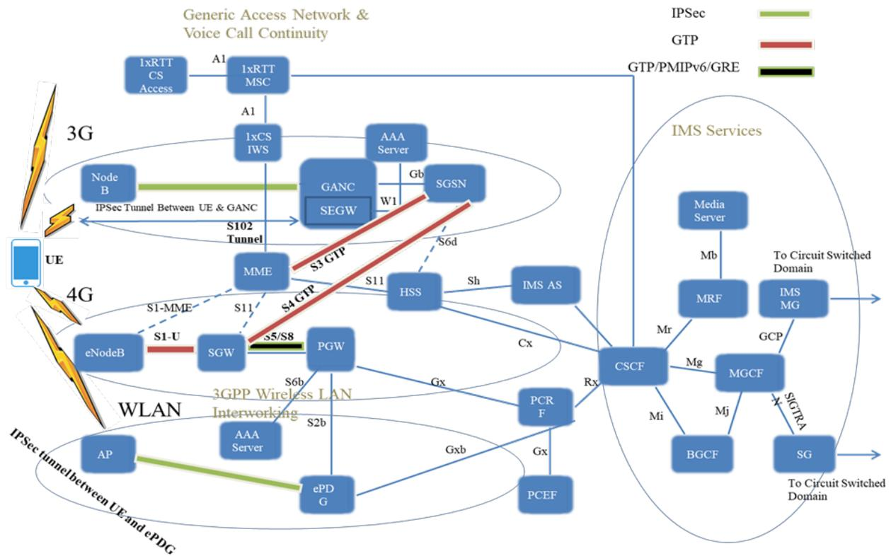
Fig. 1. Generic Heterogeneous Networks and Interworking Architecture.
