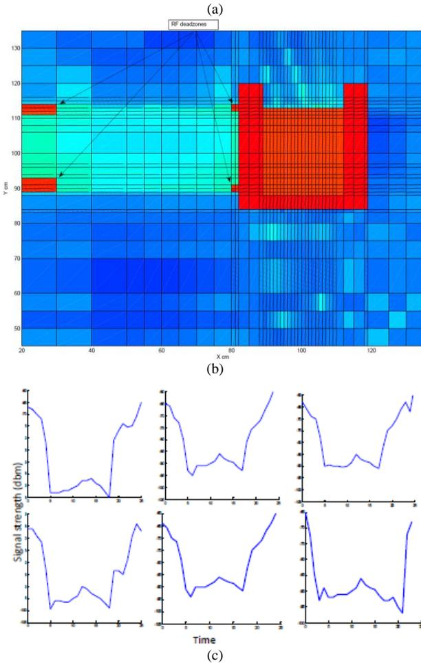
Fig. 5. Cage Obstacle (a) RF-SS Measurements (b) Top view of (a), and (c) Waveforms for Multiple Trajectories.
