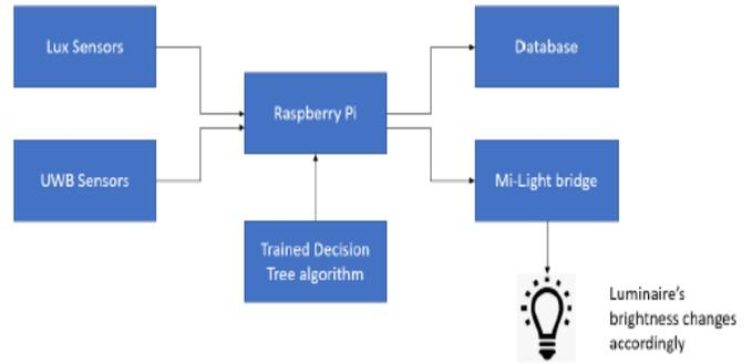
Fig. 24. Lighting Control System with the Trained Decision Tree Algorithm.
