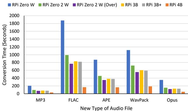
Fig. 22. Audio Conversion Performance with PTS for Different RPi Models.
