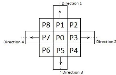
Fig. 1. Four Directions for Selecting Noise-Free Pixels [29].
