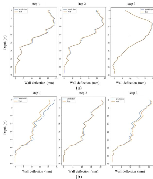
Fig. 7. Measured Wall Displacement Profiles versus Prediction (a) Excavation Site A, (b) Excavation Site B.
