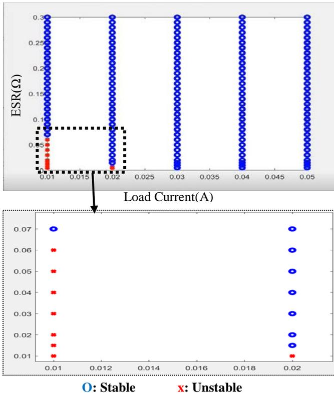
Fig. 10. ESR Tunnel Graph through Manual Characterization.
