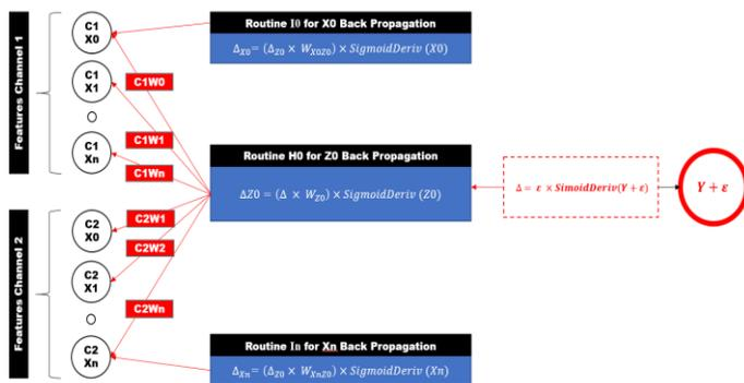
Fig. 9. Channeled Back-Propagation using Layer Set of Routines.
