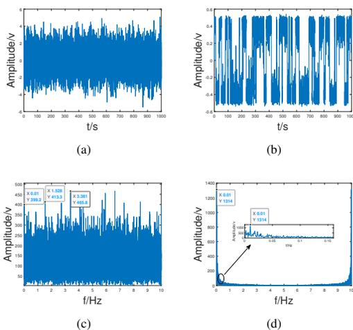
Fig. 4. (a) Received Signal in Time Domain, (b) Output Signal in Time Domain, (c) Received Signal in Frequency Domain, (d) Output Signal in Frequency Domain.
