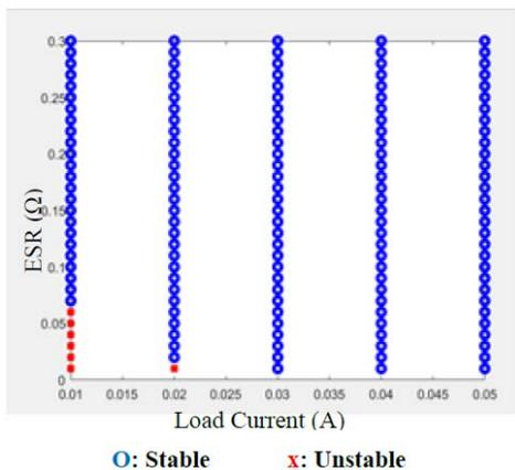
Fig. 15. ESR Tunnel Graph using the SI-NN Approach.
