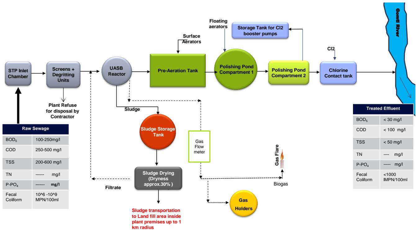
Fig. 3. Process Flow for 345 MLD UASB-based Bharwara STP.
