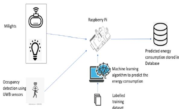
Fig. 27. Proposed System to Predict Energy Consumption.
