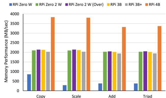
Fig. 14. Results of the Memory Performance with STREAM for Different RPi Models.
