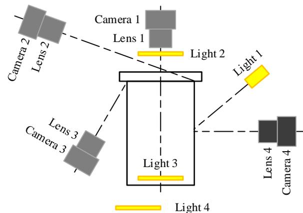
Fig. 2. Schematic Diagram of Machine Vision System for the Cylinder Liner Defect Detection.
