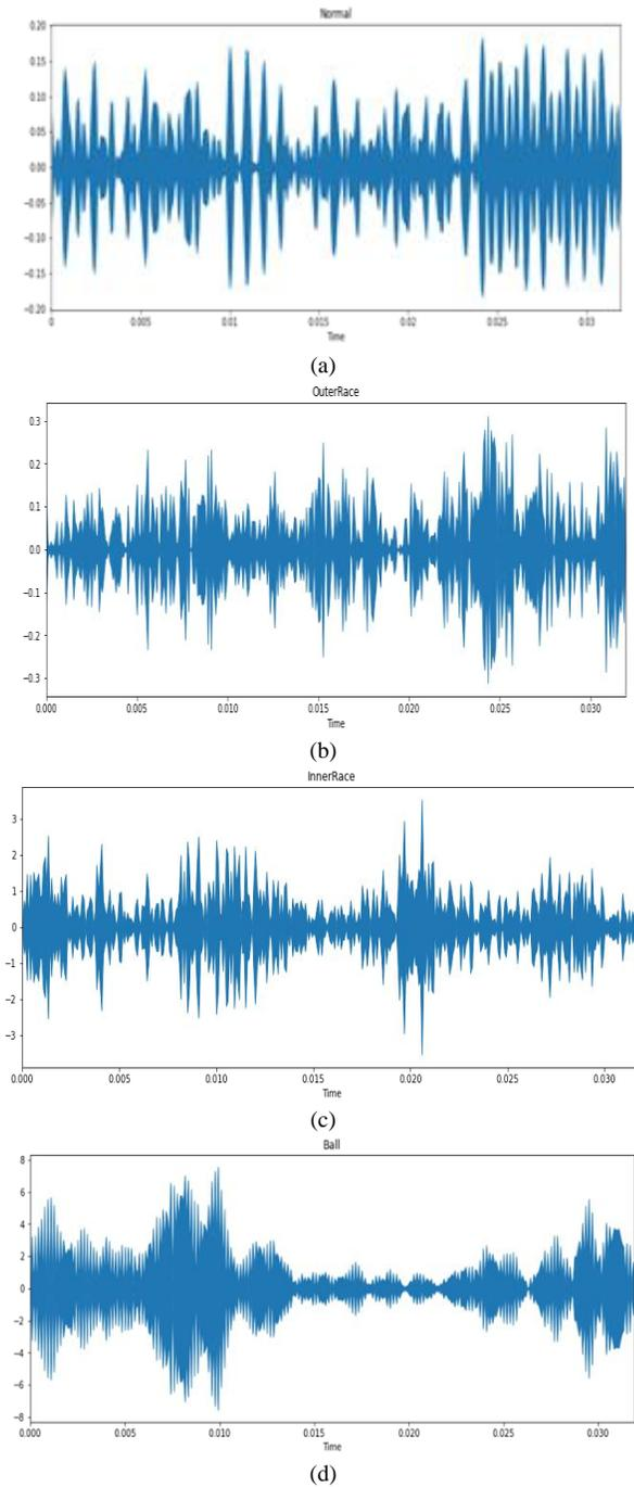
Fig. 6. (a). Time-domain Feature Representation for Normal Bearing, (b). Time-Domain Feature Representation for Outer Race Fault, (c). Time-Domain Feature Representation for Inner Race Fault, (d). Time-Domain Feature Representation for Ball Fault.
