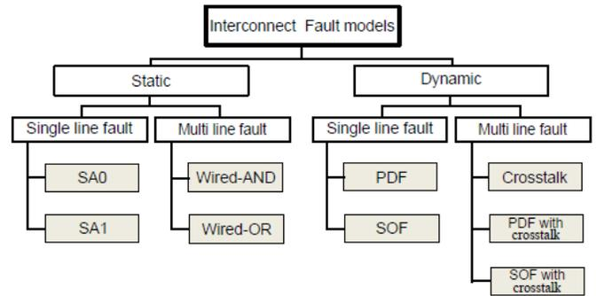
Fig. 2. Classification of Interconnect Fault Models [14]
