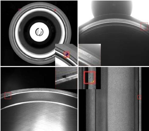
Fig. 4. Sand Defect Images of the Top Face, the Skirt, the Inner Wall and the Outer Wall of the Cylinder liner from Top Left to Bottom Right.
