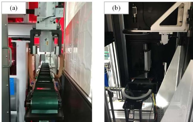
Fig. 10. Two subsystems. (a) is the Feeding Subsystem and (b) is the Imaging Subsystem.
