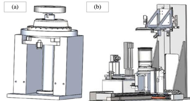
Fig. 12. Two Designs of Detection Room. (a) Rotating Platform and (b) Supports and Mechanical Interfaces.
