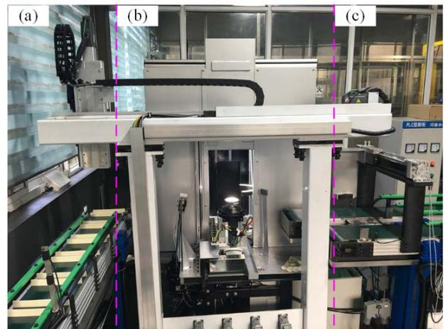
Fig. 9. On Site Cylinder Liner Defect Detection System. (a) is the Feeding Subsystem, (b) is the Detection Room and its Core Part is the Imaging Subsystem and (c) is the sorting Subsystem.
