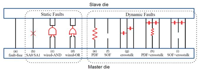
Fig. 3. Static and Dynamic Interconnect Faults [14]
