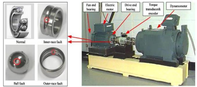
Fig. 5. Experimental Set-up of CWRU Data Collection.
