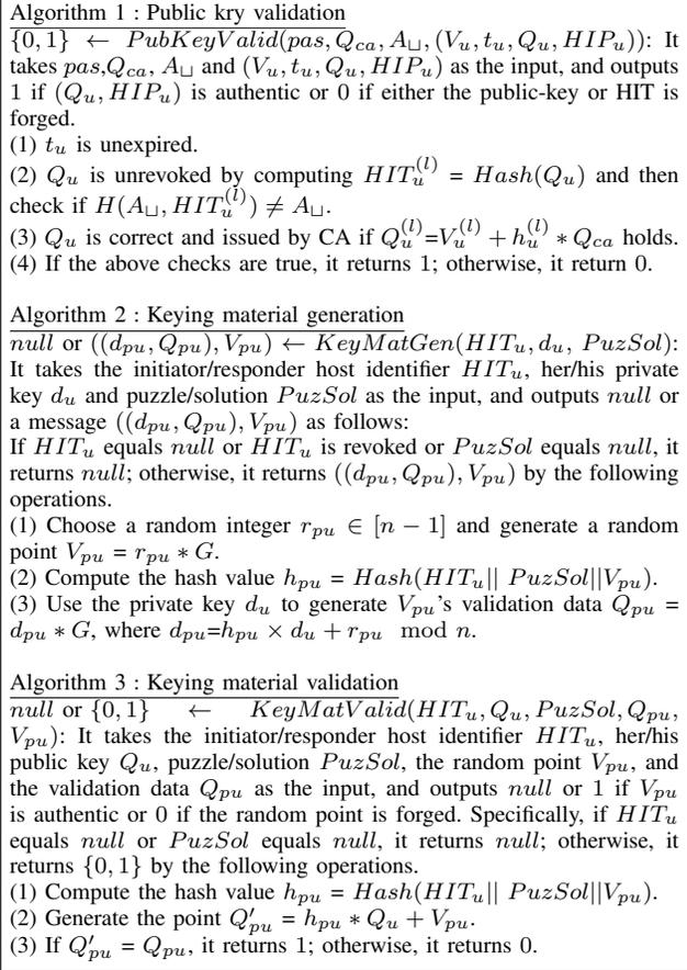
Fig. 6. The Algorithms in the Improved HIP
