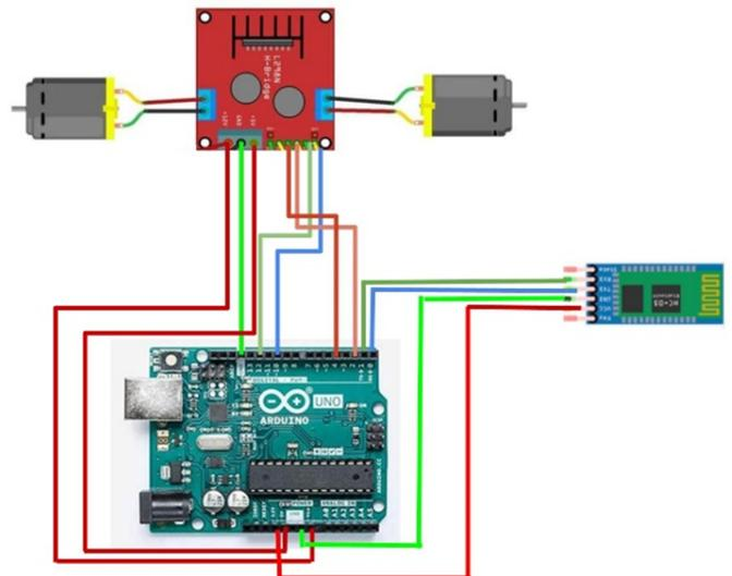
Fig. 4. Circuit Diagram of Robot Controlling with Bluetooth
