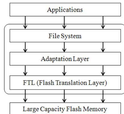
Fig. 1. Architecture of Flash File System.
