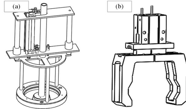
Fig. 11. Two submodules. (a) is the Cleaning Subsystem and (b) is the Grasping Device.
