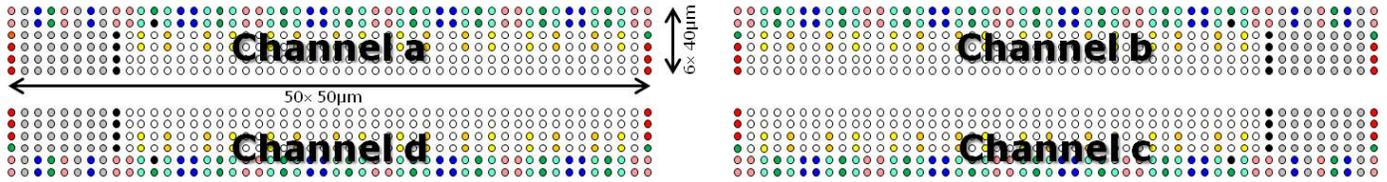
Fig. 5. The Interface for JEDEC Wide-I/O [30]
