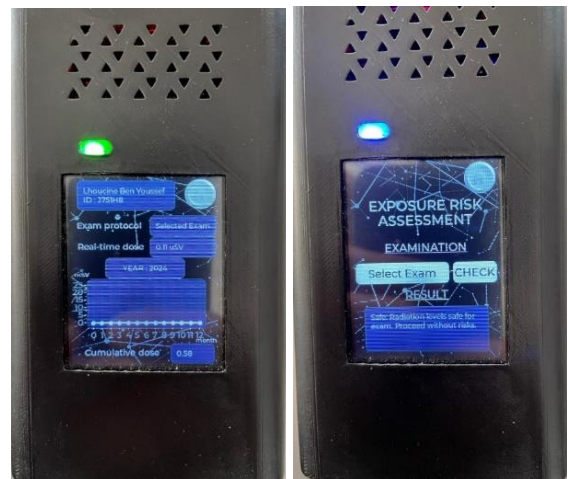
Fig. 4. Smart X-ray Geiger Data Logger for radiation dose measurement and monitoring.
