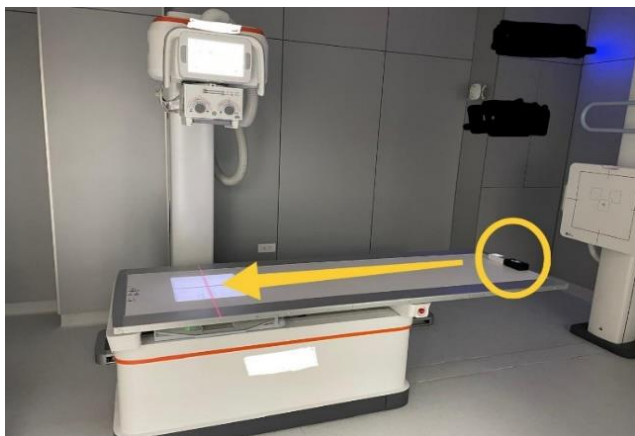
Fig. 6. Verification of scattered radiation measurements using smart X-ray Geiger Data Logger and BR-6 Geiger counter.
