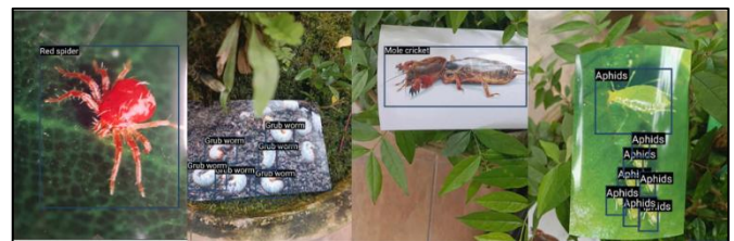
Fig. 18. Correct real-time predictions of pests using the YOLOv9t model integrated into a smartphone application in a simulated plant environment.
