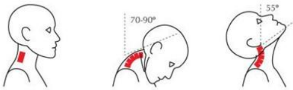
Fig. 9. Head movement conditionals to accelerate or decelerate the vehicle.
