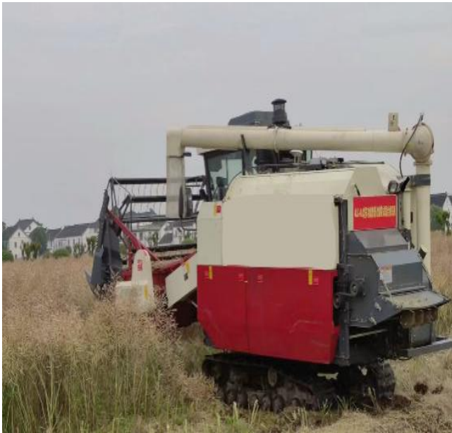
Fig. 6. Field experiment of harvesting rapeseed.
