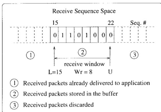
Fig 4: A receiver's receive window and related variables.
