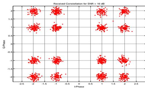
Figure 5. Received 16-QAM constellation with SNR =16 dB
