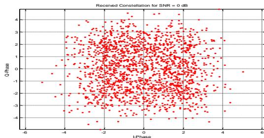
Figure 4. Received 16-QAM constellation with SNR =0 dB
