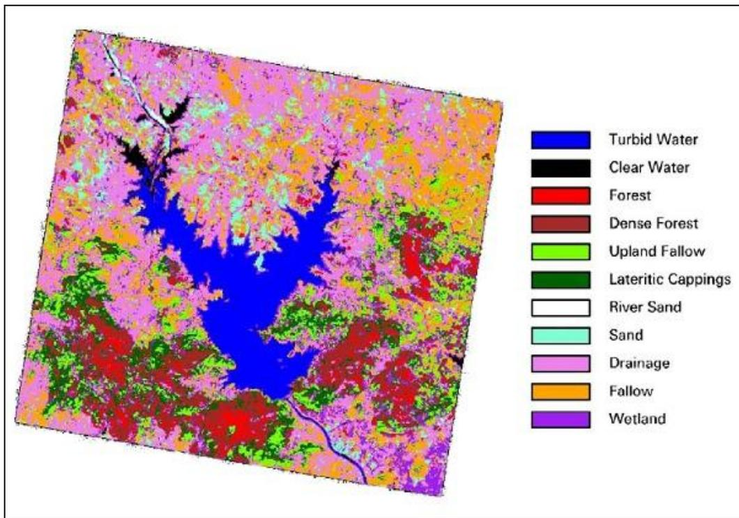
Figure 4. Classified image using standard Maximum Likelihood classifier.
