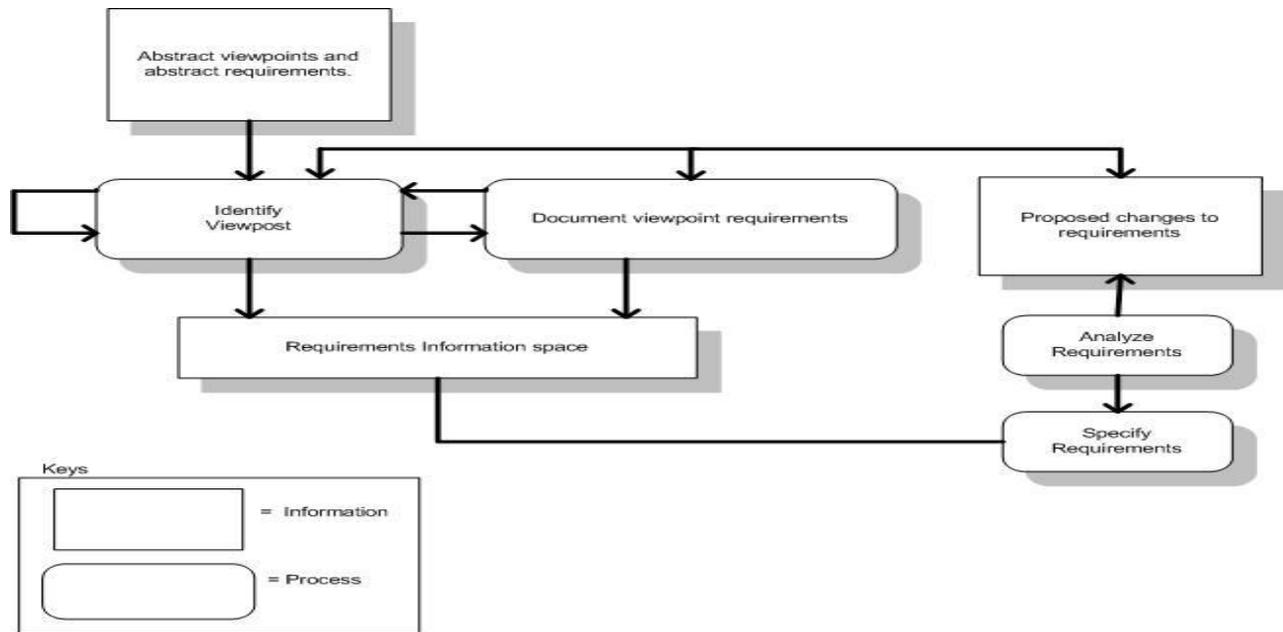
Figure 1. The VORD Process Model
