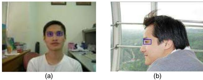
Figure 8. Two kinds of face pose. (a) Frontal face pose with two eyes extracted. (b) Profile face pose with only one eye extracted.
