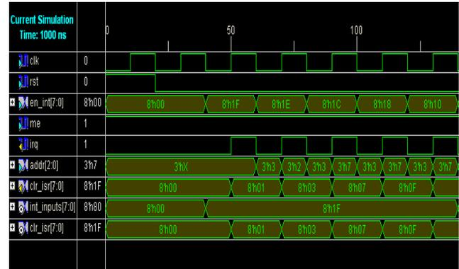
Figure 10. Top level timing diagram of Interrupt Controller
