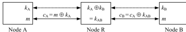
Figure 4 Forwarding with link-specific keys
