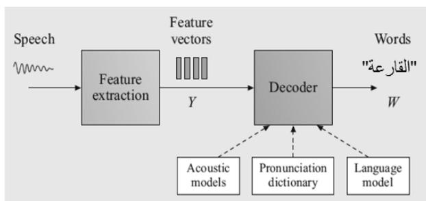
Figure 2. Architecture of an HMM based recognizer
