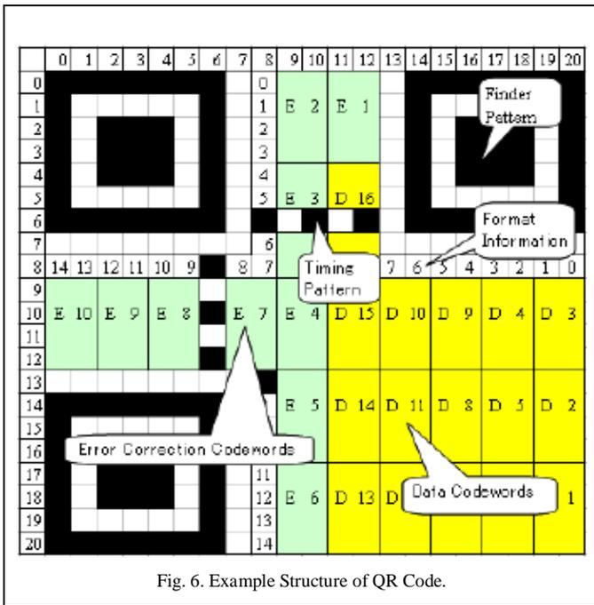
Fig. 6. Example Structure of QR Code.
