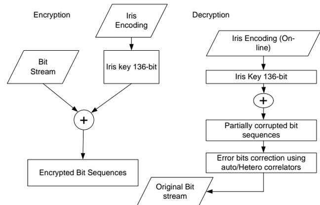
Figure 3. A sequence sketch of Non-repudiation cryptosystem.
