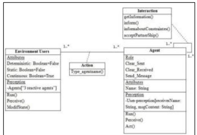
Figure 8. UML Class diagram for a chat application
