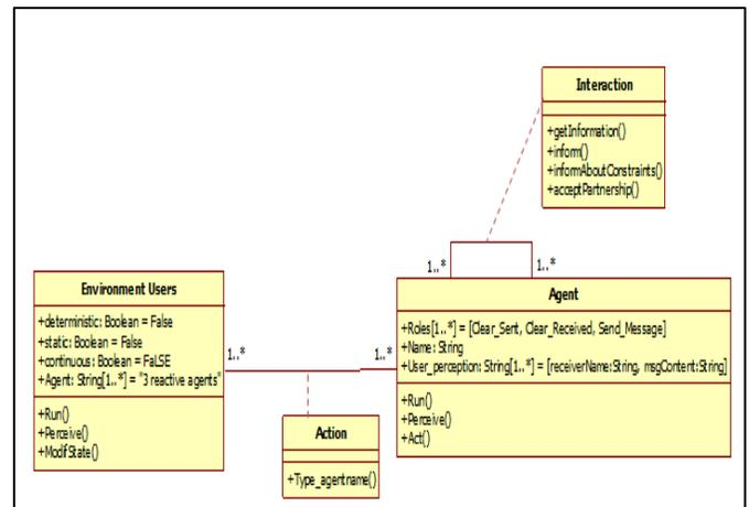
Figure 7. AUML Class diagram for a chat application
