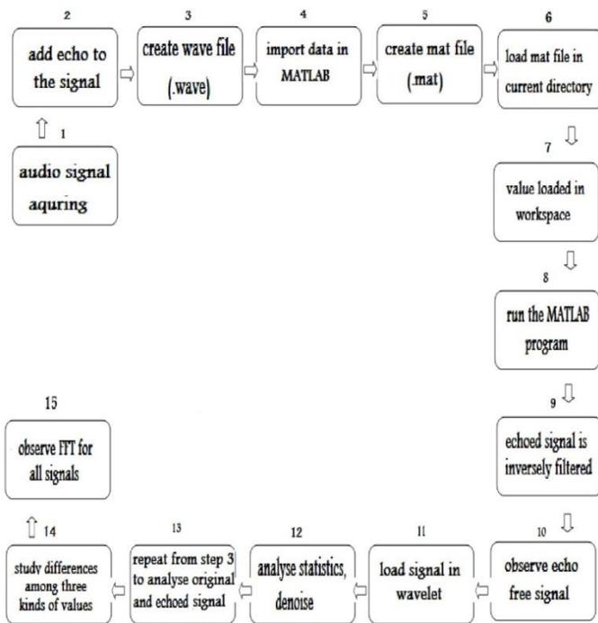
Figure 1. Flowchart for echo cancellation using MATLAB
