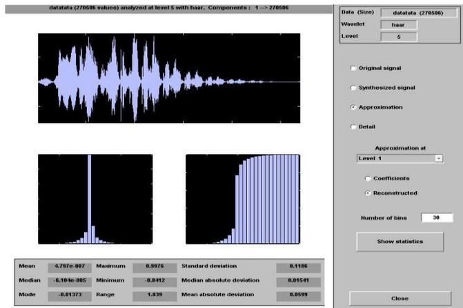
Figure 6. Analyzing signal with echo with wavelet
