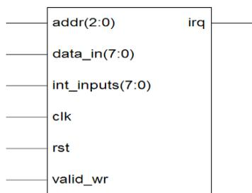
Figure 13. Signals of Interrupt Controller(IC)
