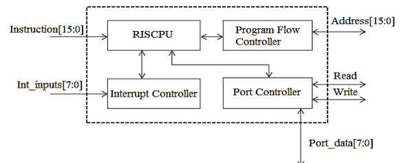
Figure 1. Block diagram of a RISI Controller
