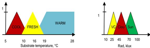
Figure 1. Temperature and radiation membership function
