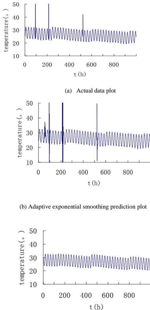
(c) Adaptive fault-tolerant exponential smoothing prediction plot
