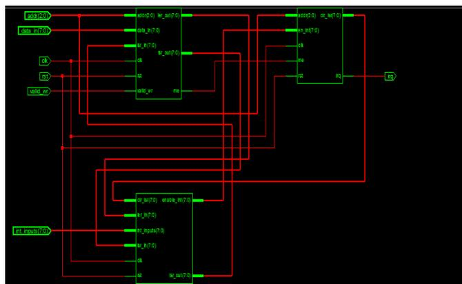
Figure 14. RTL Schematic of Interrupt controller of RISI Controller
