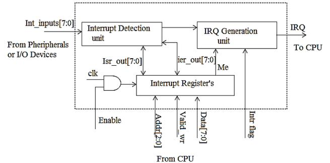
Figure3. Block diagram of Interrupt Controller
