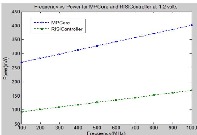
Figure 20. Power consumption of RISI CONTROLLER at 1.2v
