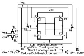
Fig.8. PP-SRAM Cell (Holding '0') with Gate Leakage Current [3]
