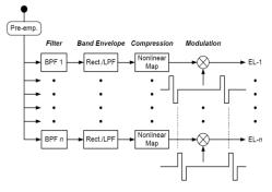
Figure4: Block Diagram of CIS Algorithm
