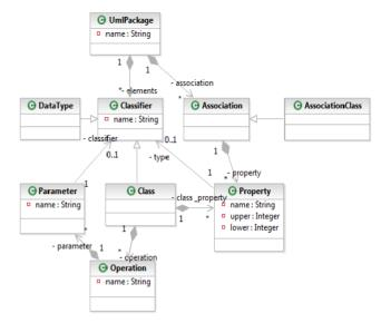
Figure 4. Simplified Meta-Model class diagram of UML.
