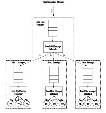
Figure 2. Grid Computing Queueing Model
