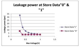
Fig.15: Leakage Power vs Substrate Bias Voltage for Data Hold '0' and '1'
