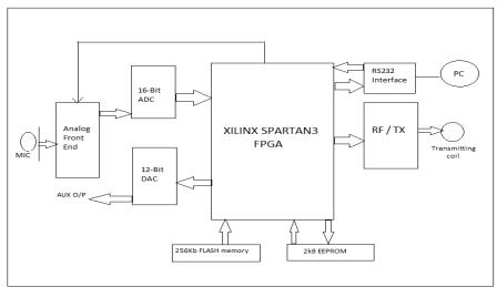
fig:1. Functional Block Diagram for Speech Processing
