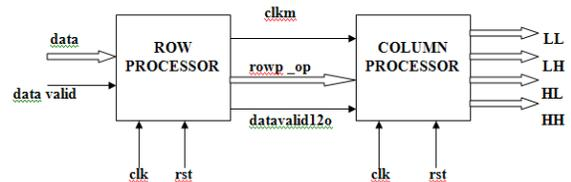
Fig .7.1 Block diagram for 1-level 2d-dwt
