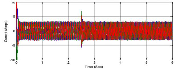
Fig. 9.b (Simulation) Motor three phase current for step up of reference speed
