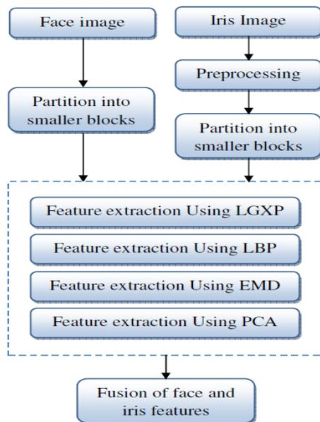
Fig.1: The Overall block diagram
