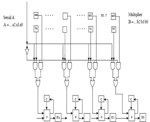
Figure 9. Array Multiplier for Soft Computing based Arithmetic
