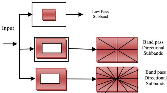
Fig 3: Block diagram of NSCT
