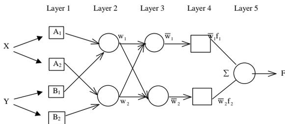
Figure 1. Anfis Structure of Two Rule Sugeno System
