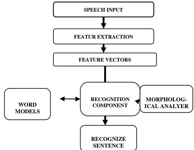
Fig. 5. Functional block diagram of the Speech Recognition Module
