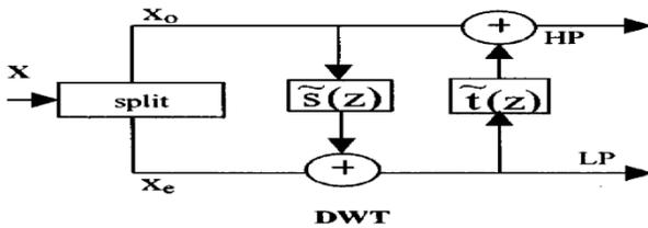
Fig. 1 Lifting Scheme
