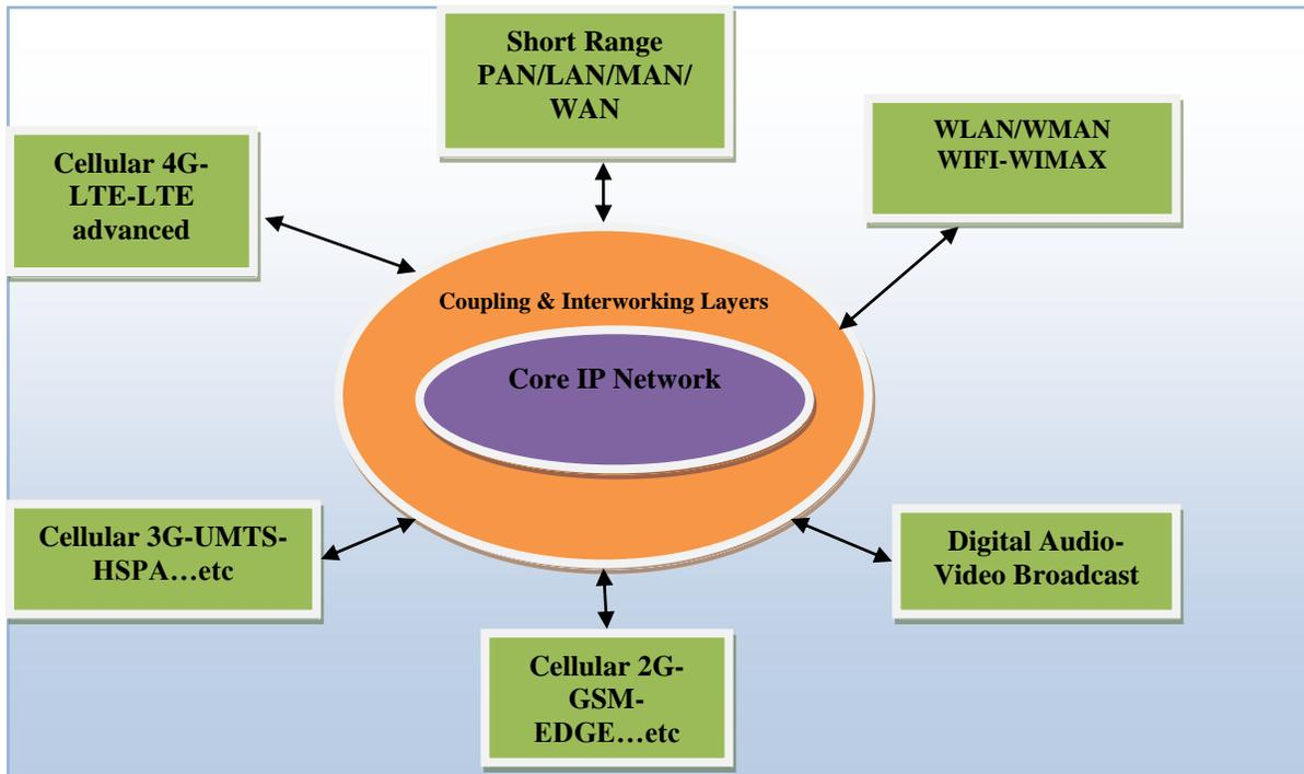
Figure 5: Core IP Network, different access systems' provision.
