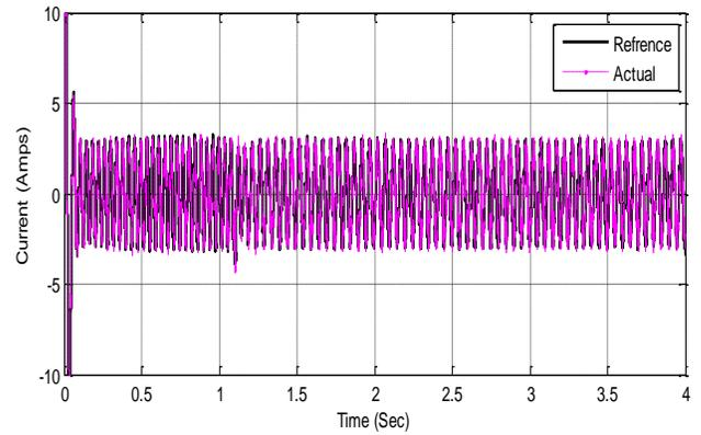
Fig. 5a (Simulation) Motor phase current and its reference command for step down of reference speed
