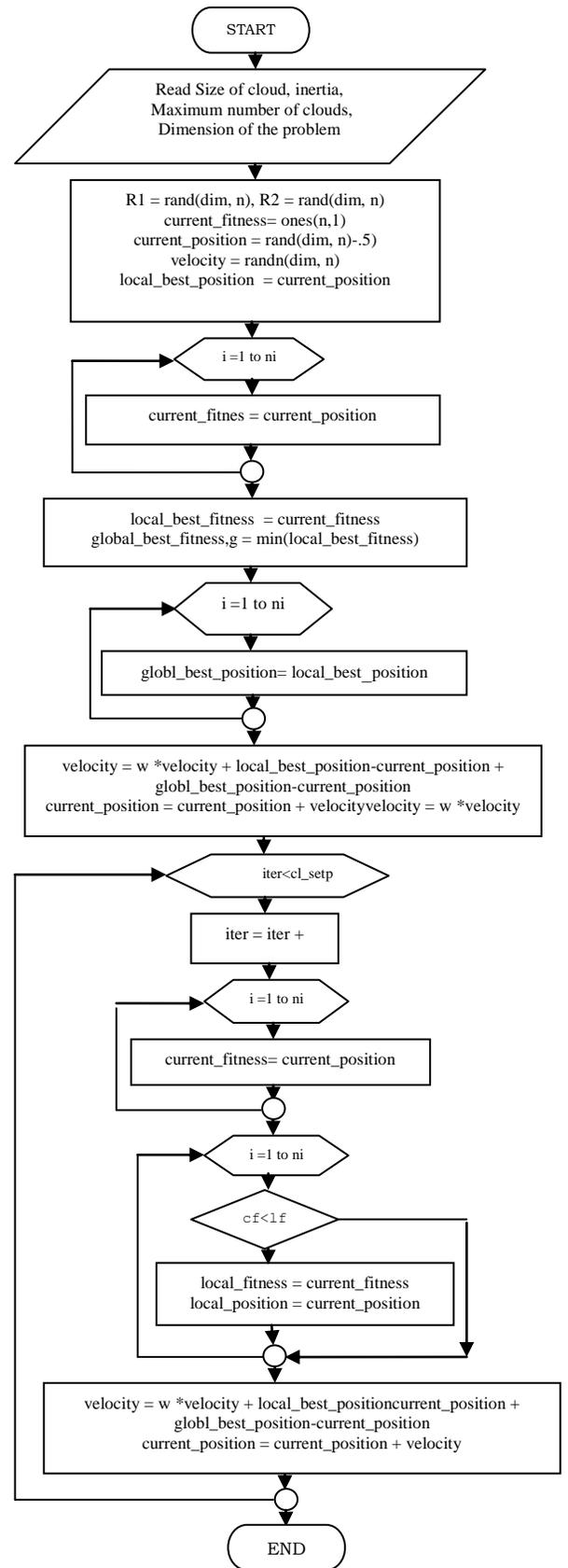
Fig. 3 Flowchart of proposed cloud computing algorithm
