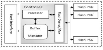
Figure 1. Basic Architecture of Solid State Disk (SSD) Storage Media
