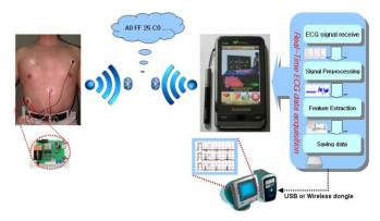
Figure 1. Real-time ECG system block diagram
