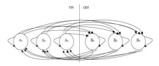
Figure 5. Markov model of error packetization algorithm
