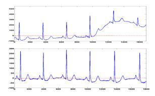
Figure 5. Baseline wandering correction (X-axis: samples, Y-axis: amplitude)
