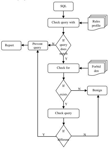
Figure 5. anomaly misuse detection flow phase
