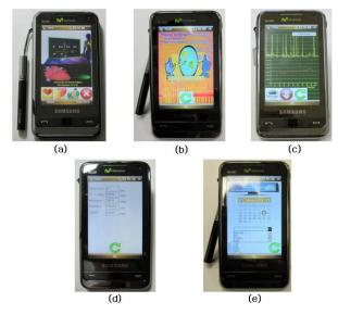
Figure 7. Mobile Phone Configuration: (a) monitoring system main view; (b) wireless connectionl; (c) real-time display of the ECG measurement; (d) the ECG parameters calculation value; (e) data history and management
