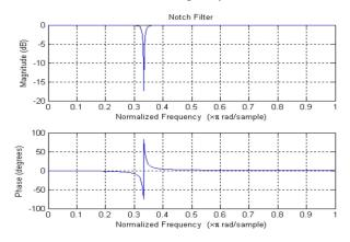
Figure 4. Magnitude and phase response of an Infinite Impulse Response(IIR) notch filter to remove 60Hz power line noise
