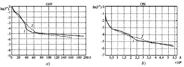
Figure 6. DF of simulated samples of the length of OFF-(a) and ON (b) - periods: curve 1 - experiment, curve 2 - simulation
