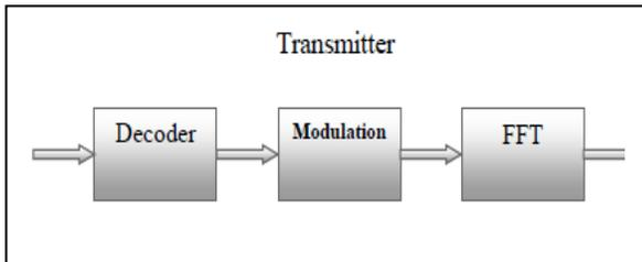
Figure. 5 OFDM Transmitter
