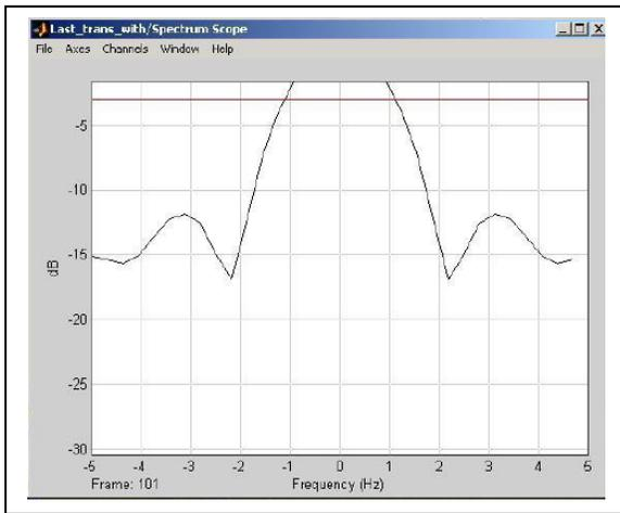
Figure 10. Output of the Transmitter with OFDM
