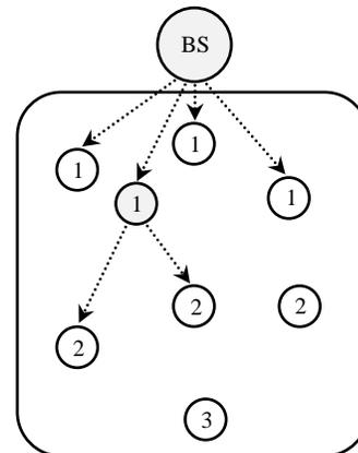
Figure 3. Initialization phase. Determination of levels and exchange of information. The base station (BS) broadcasts a message to the 1-hop nodes. A node explores the next-hop.
