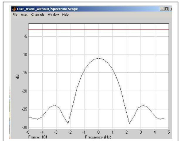
Figure 8. Output of the Transmitter without OFDM
