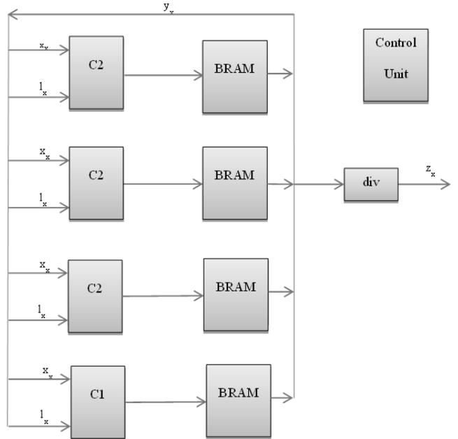
Fig. 10. A scalable architecture for Cholesky decomposition.
