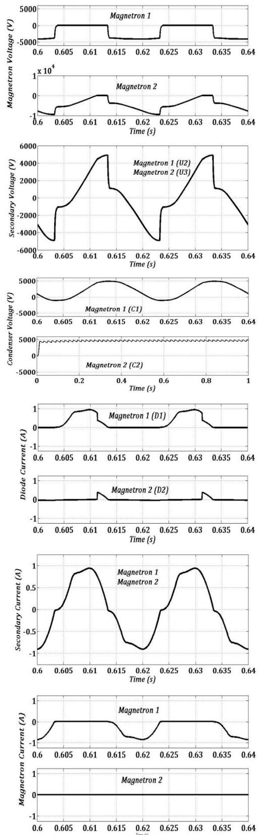
Fig. 11. Oscillograms of currents and voltages of the modeled circuit during the simulation in non linear regime with Matlab-Simulink code (M<sub>2</sub> in failure)
