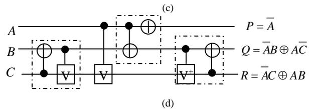
Fig. 7. Quantum cost of proposed SAM gate.
