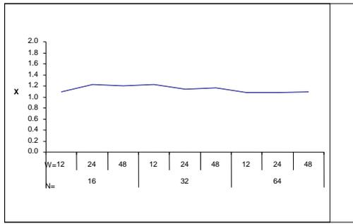
Fig. 9. Ratio of SD- to CSA FIR filter delays
