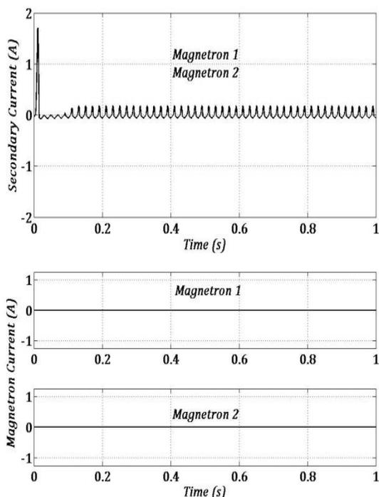
Fig. 14. Oscillograms of currents and voltages of the modeled circuit during the simulation in non-linear regime with Matlab-Simulink code (M<sub>1</sub> & M<sub>2</sub> in failure)
