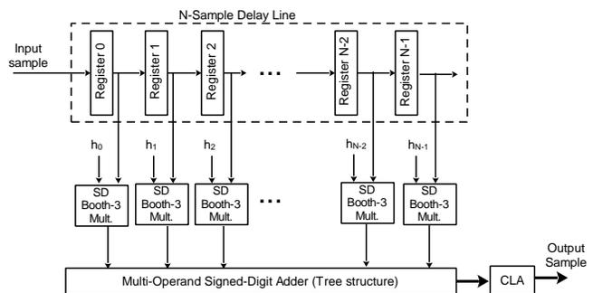
Fig. 4. Signed Digit FIR Filter [12]
