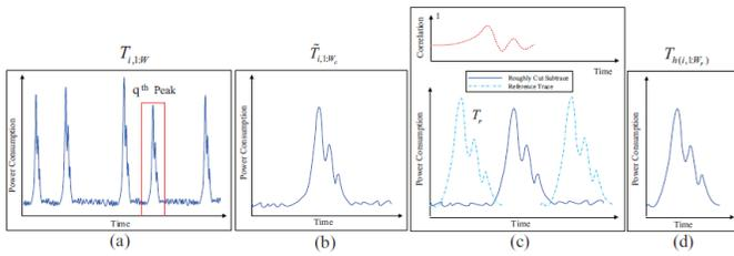
Fig. 5. Steps of aligning power traces (A)Find the  $q^{\text{th}}$  peak, (B) Coarse Extraction, (C)Fine Tuning, and (D)Fine Tuned Extraction
