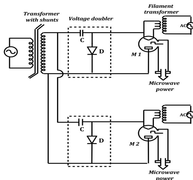
Fig. 1. New single-phase high voltage power supply for N= 2 magnetrons (Amperex Technology)
