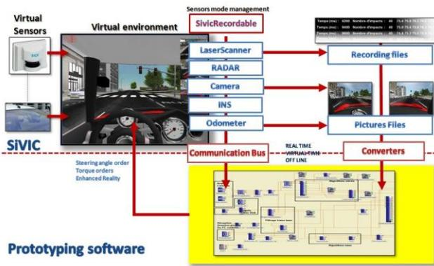
Fig. 1. General architecture of ADAS prototyping with SiVIC
