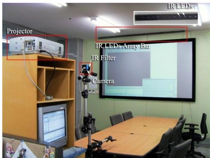
Fig. 8. The experimental environment for the proposed system.
