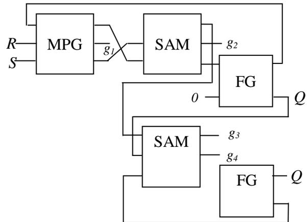
Fig. 12. Proposed Design of Master Slave SR flip-flop with only  $Q$  output
