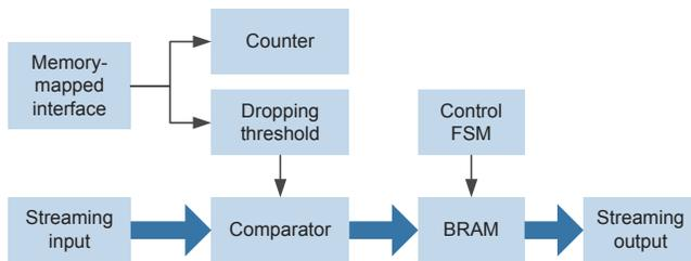
Fig. 17: The proposed structure for DMP dropping module.
