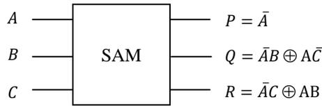
Fig. 6. Block diagram of a 3\*3 SAM gate
