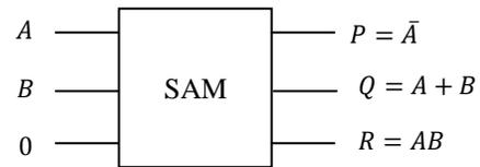
Fig. 8. SAM gate as two input universal gate.
