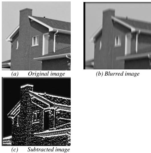
Fig. 7. Edge Extraction using FIR filter [12]
