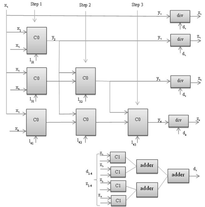
Fig. 9. A pipeline architecture for Cholesky decomposition.
