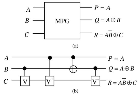
Fig. 9. (a) Block diagram of 3\*3 MPG and (b) Equivalent quantum representation
