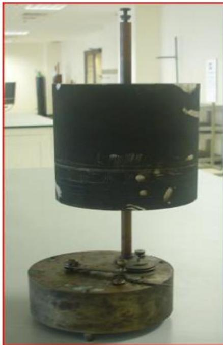
Fig. 1. Conventional Kymograph (front view)
