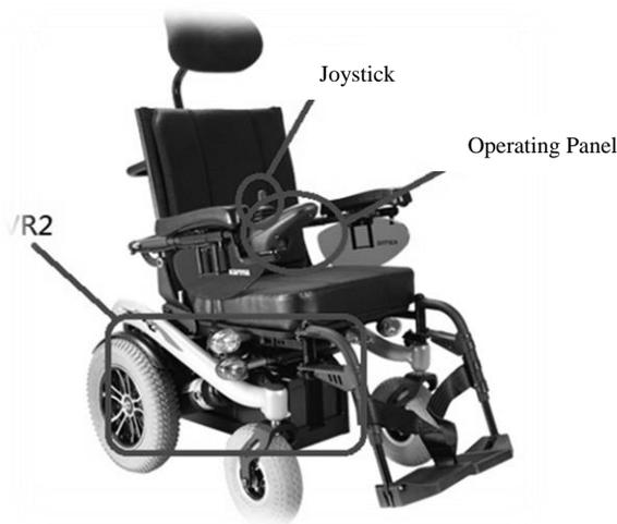
Fig. 7. VR2-controlled electric wheelchair
