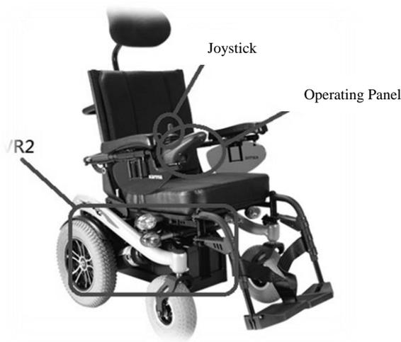
Fig. 7. VR2-controlled electric wheelchair
