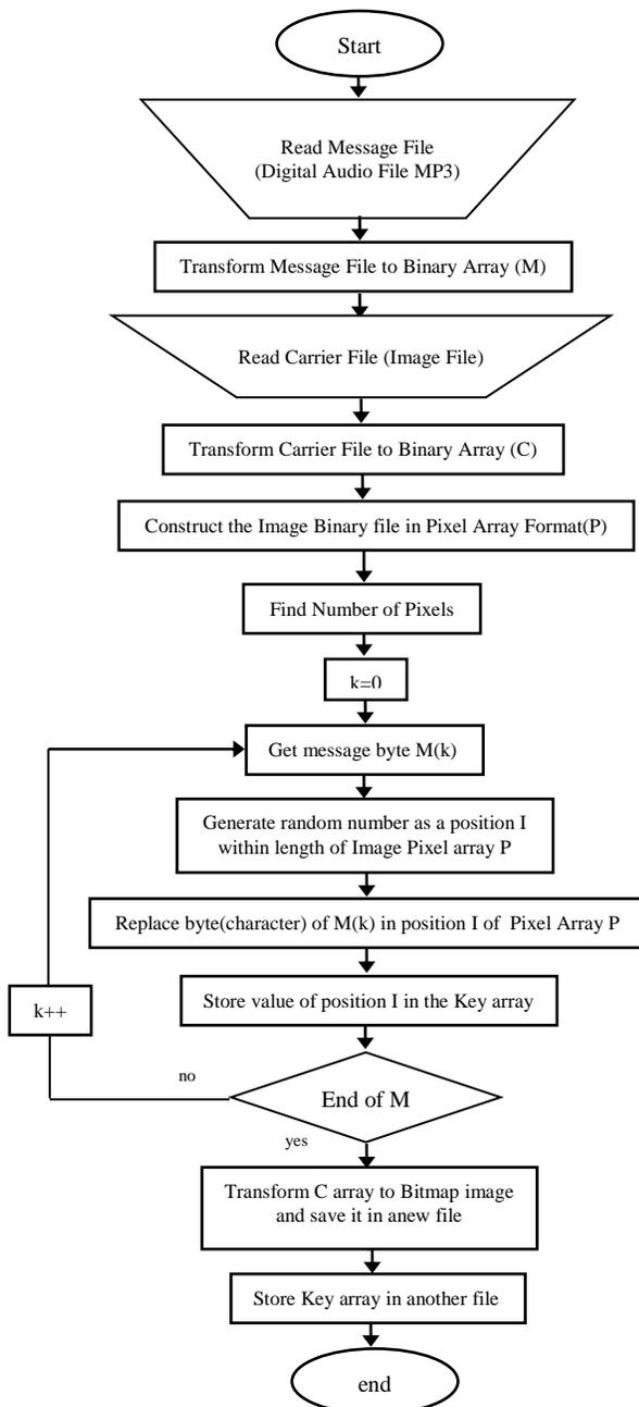
Fig. 7. Algorithm of steganography in images using pixels
