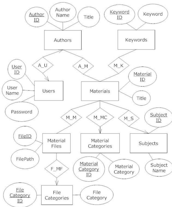
Fig. 2. ER diagram of the database ElibraryDB
