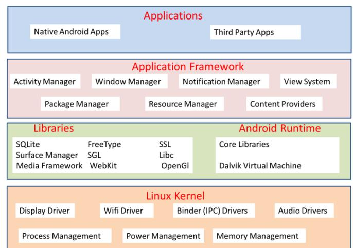
Fig. 1. Android operating system architecture
