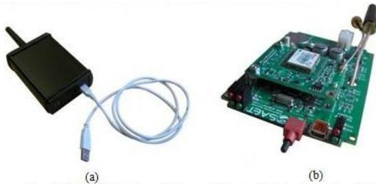
Fig. 1. SAT-SURF: view of the case (a) and of the hardware board (b)
