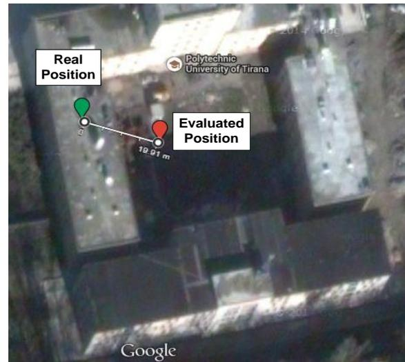
Fig. 10. Estimated user's position from the adaptive PVT algorithm
