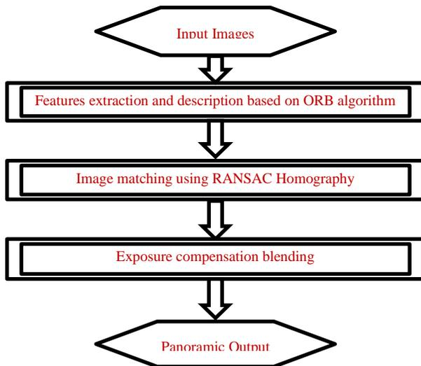
Fig. 2. The block diagram of the proposed panoramic image system
