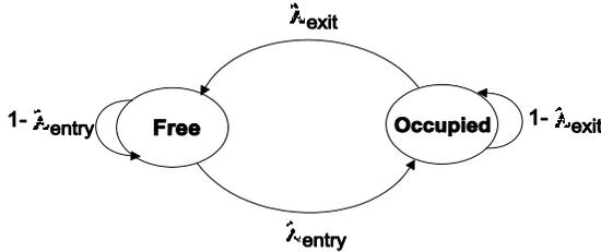
Fig. 4. Grid model – a two state Markov chain[16]
