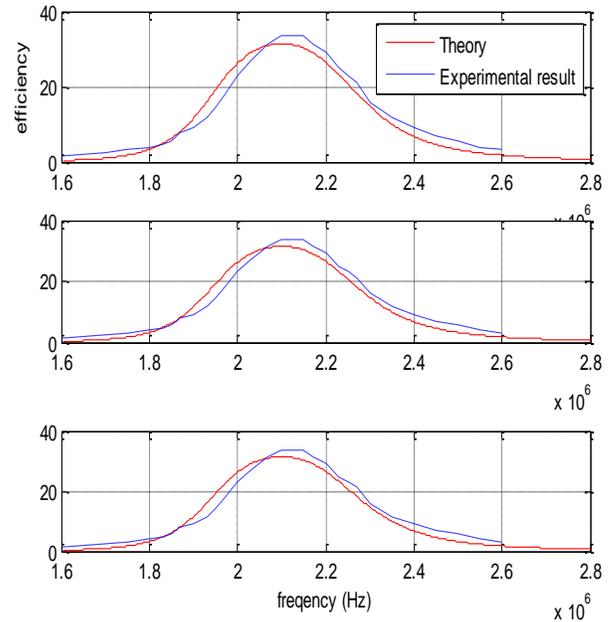
Fig. 15. Efficiency versus frequency for three receivers system
