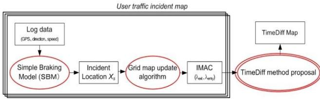
Fig. 3. Process for generating traffic safety map
