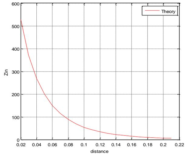
Fig. 11. Input resistance versus distance at resonant frequency
