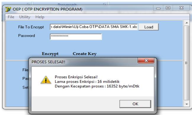
Fig. 7. Excel file encryption process
