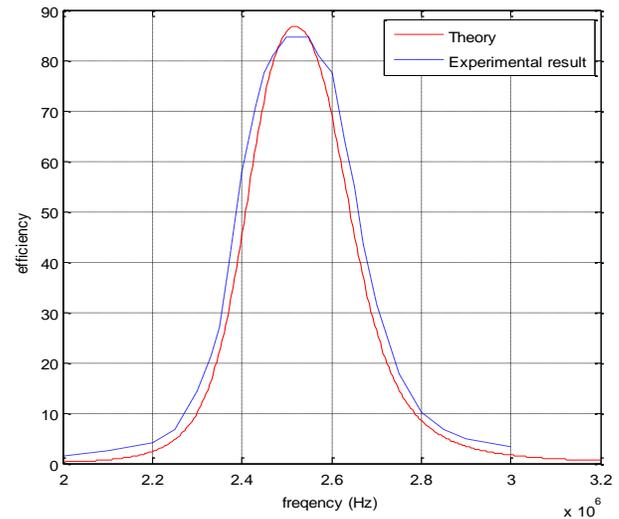
Fig. 12. Efficiency versus frequency at 15.5cm distance and  $f_0=2.5\text{MHz}$  (Resonance Frequency Effect)
