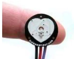
Fig. 4. Pulse rate sensor SEN-11574
