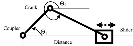
Fig. 4. A crank–slider linkage system (Modified – Re-drawn from [9])
