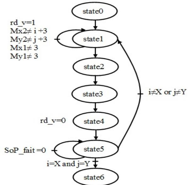
Fig. 4: FSM of the control unit
