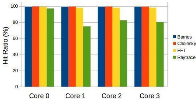
Fig. 5. Hit Ratio in L1-Data cache of CMP when running four applications
