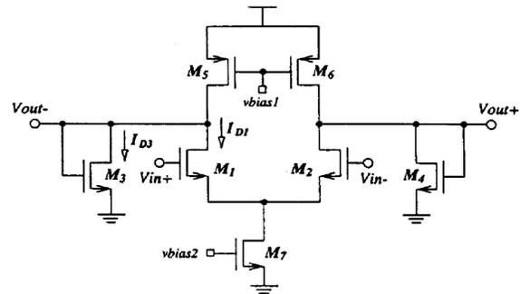
Fig. 9. Proposed limiting amplifier
