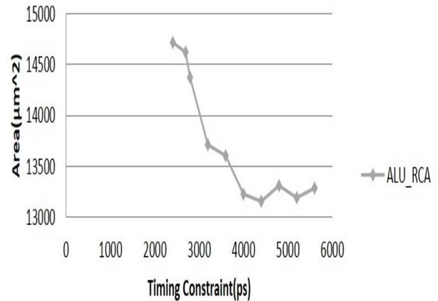
Figure 4: Scaling of Area of ALU-RCA with Timing Constraint
