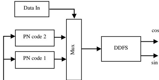
Fig. 4. Block diagram of the modulator
