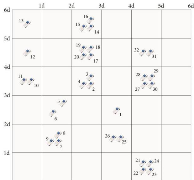
Fig. 1. An example of a grid-based MANET environment
