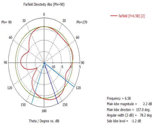
Fig. 13. 1D plot of Directivity at Resonant Frequency of 6.58 GHZ
