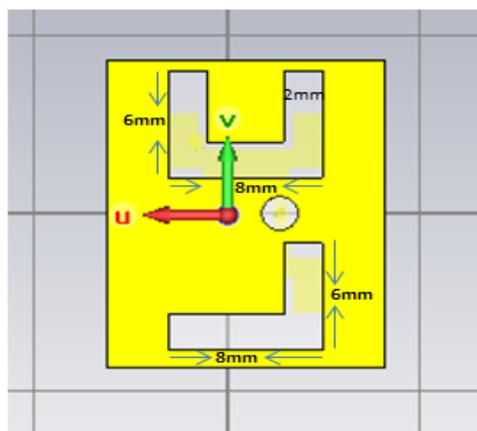
Fig. 2. Back view of Dual Fractal Patched Pi Antenna
