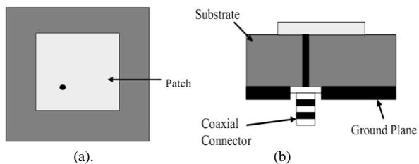
Fig. 1. (a) Top view of Micro strip patch antenna (b) Side view of patch antenna (Coaxial Cable Feed)
