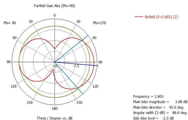
Fig. 6. 1D plot of Gain at Resonant Frequency Of 2.603 GHz
