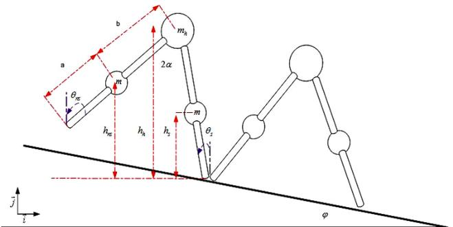
Fig. 2. Compass robot
