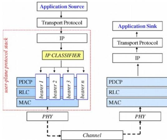
Fig. 1: Implemented model of VoLTE protocol stack [12]
