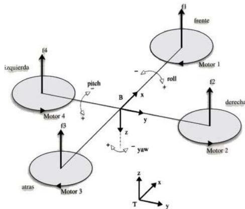
Figure 9: Principle of operation of Tetramotor.
