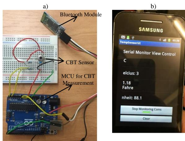
Fig. 12. (a) Experimental setup for Arduino based CBT measurement; (b) Monitoring of CBT results on the smartphone
