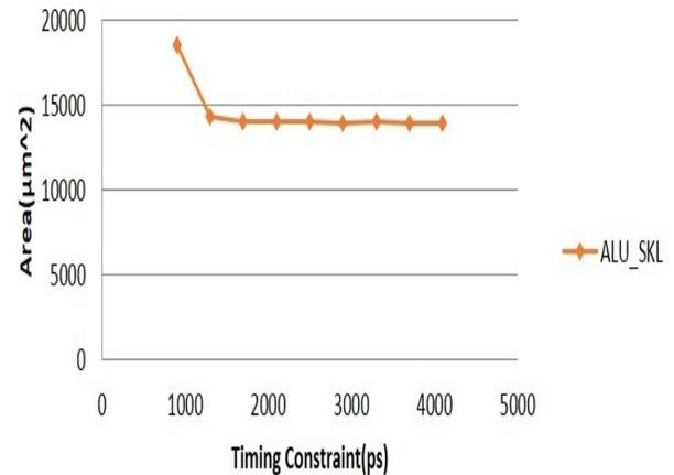
Figure 5: Scaling of Area of ALU-SKL with Timing Constraint
