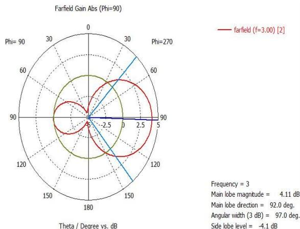
Fig. 9. 1D plot of Gain at Resonant Frequency Of 3.00 GHz
