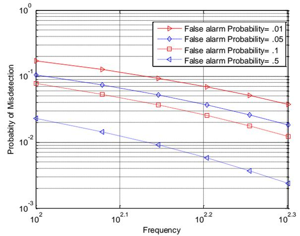
Fig. 7. Variation of the probability if misdetection against frequency for fixed false alarm rate
