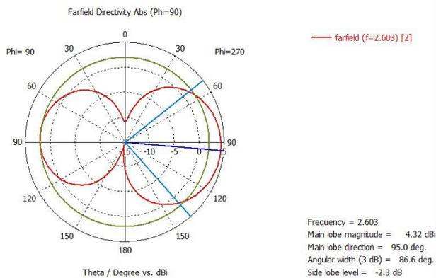
Fig. 7. 1D plot of Directivity at Resonant Frequency Of 3.00 GHz
