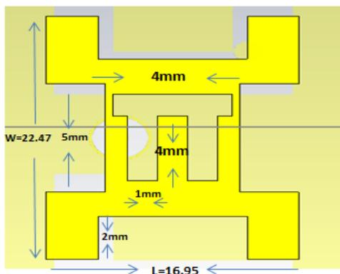
Fig. 4. Bottom View of Dual Fractal Patched Pi Antenna
