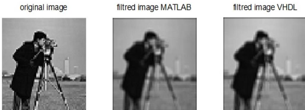
Fig. 9: Filtered image with sigma=1.5
