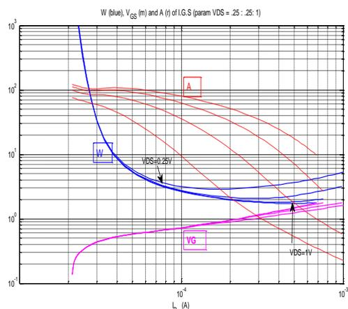
Fig. 11. Plot of the gate widths  $W$ ,  $V_{GS}(V)$  and gain  $A$  versus drain current for transistor frequency equal to 100 MHz
