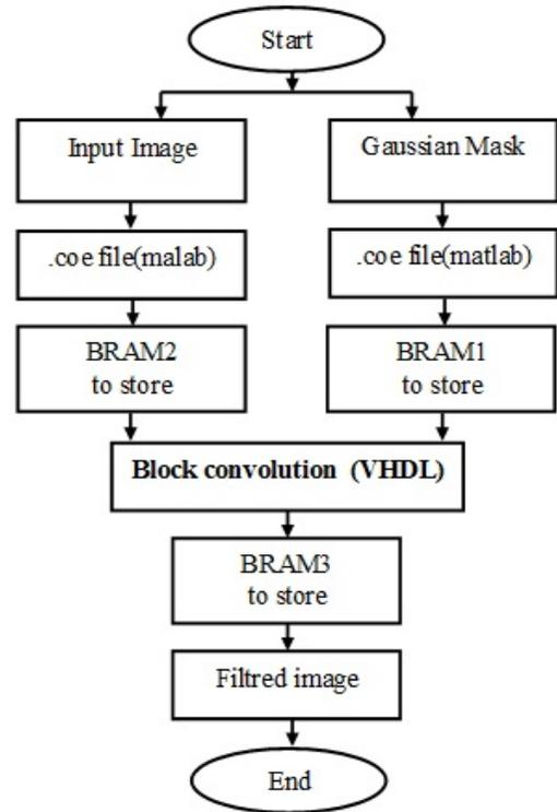
Fig. 2: Block diagram of image filtering
