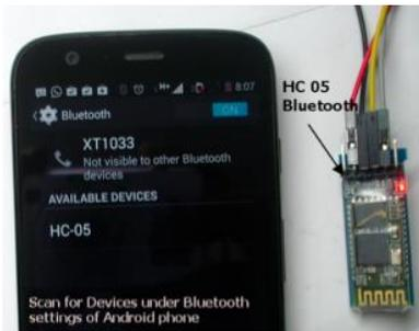
Fig. 16. The view of Bluetooth module while pairing with the smartphone
