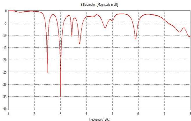
Fig. 8. Return Loss Plot of Teflon
