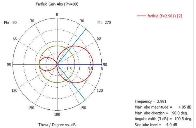
Fig. 15. 1D plot of Gain at Resonant Frequency of 2.98 GHZ
