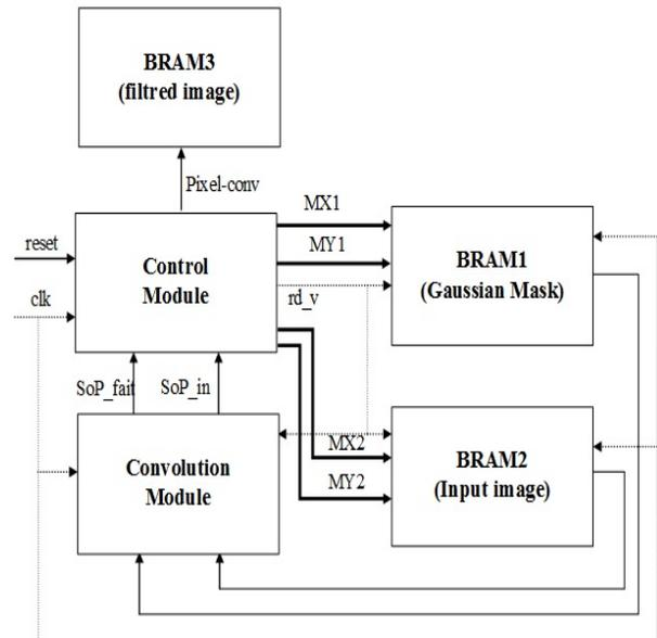
Fig. 3: Synchronous architecture of image filtering
