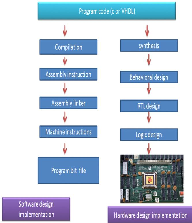
Fig. 2. Design process used in embedded system
