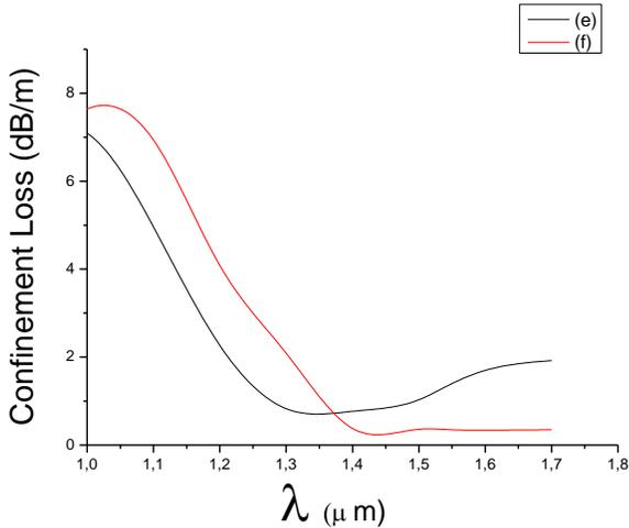
Fig. 5. Confinement loss plot according to wavelength
