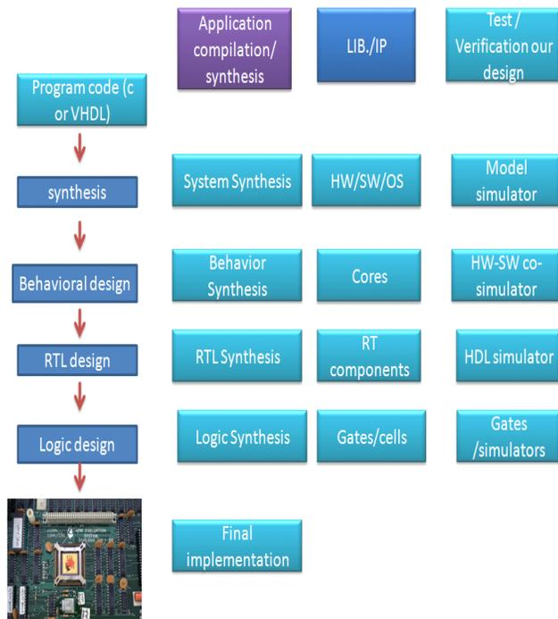
Fig. 3. Design process technology of embedded system
