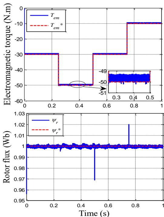
Fig. 5. Classical DTC strategy responses (reference tracking test)
