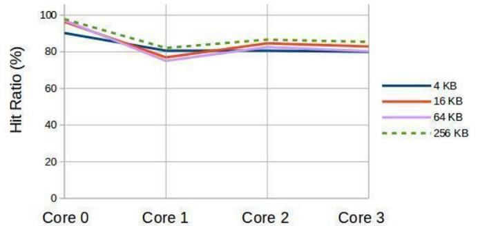
Fig. 6. Hit Ratio in L1-Data cache of 4 CMPs when running Raytrace
