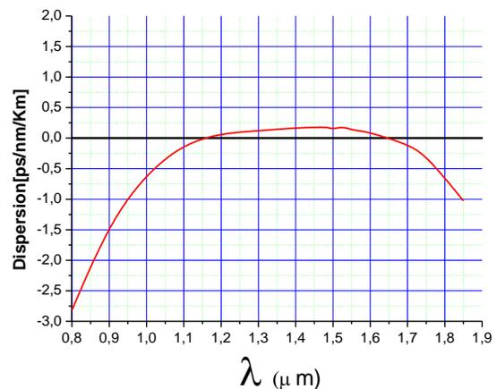
Fig. 7. Chromatic dispersion of structure (f) as a function of wavelength
