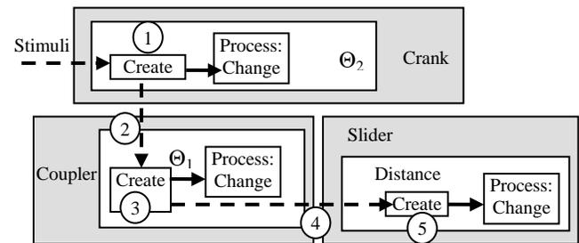
Fig. 5. FM representation of the crank–slider linkage system
