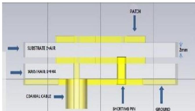
Fig. 3. Front View of Dual Fractal Patched Pi Antenna
