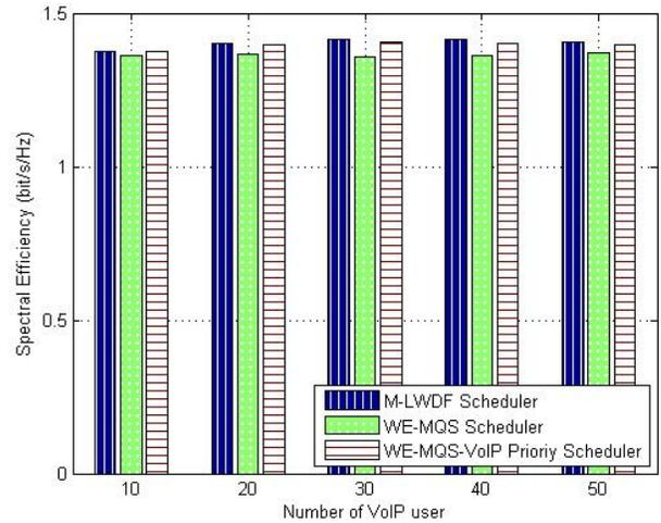
Fig. 8: Spectral efficiency vs number of VoIP user
