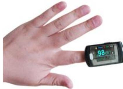
Fig. 6. Bluetooth finger PPG sensor
