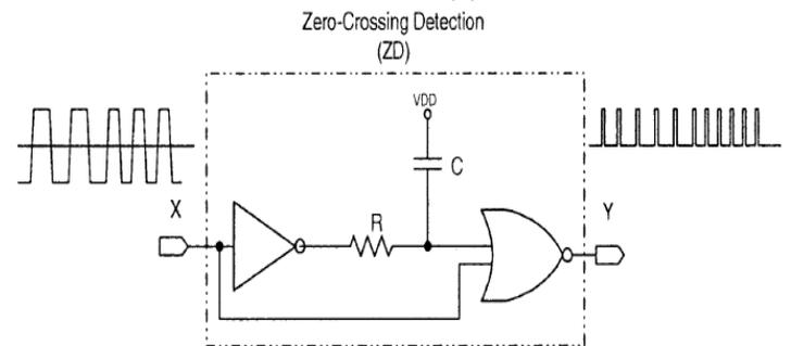
Fig. 11. Zero-crossing Detection
