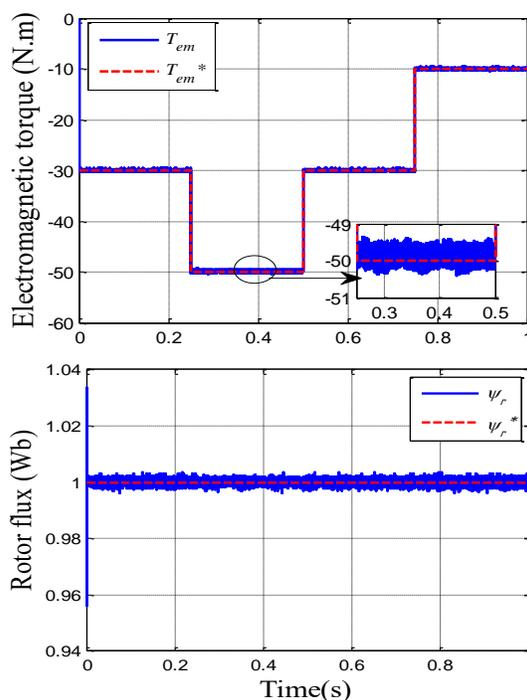
Fig. 6. DTC-HOSMC strategy responses (test of reference tracking)
