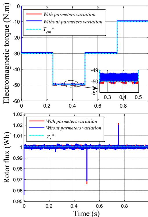
Fig. 7. Classical DTC strategy responses (test of robustness)
