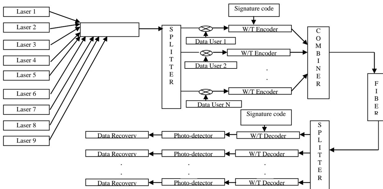
Fig. 1. OCDMA system Block Diagram
