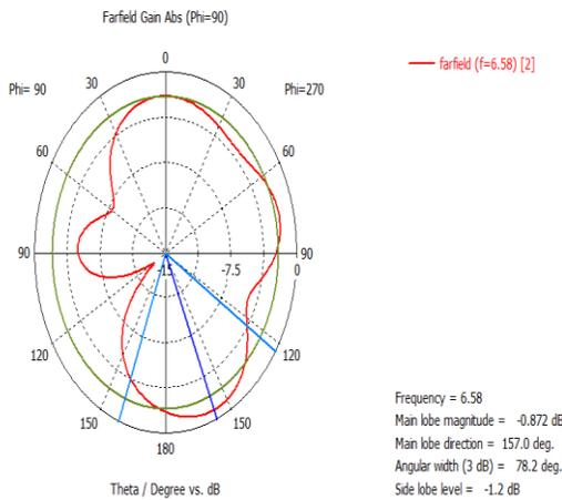
Fig. 12. 1D plot of Gain at Resonant Frequency of 6.58 GHZ
