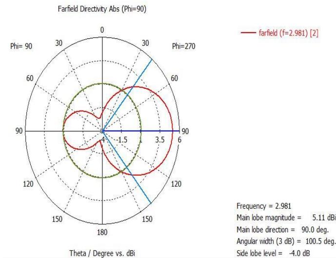
Fig. 16. 1D plot of Directivity at Resonant Frequency of 2.98GHz
