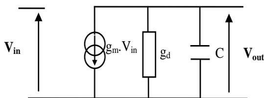
Fig. 8. Small signal equivalent circuit of elementary amplifier
