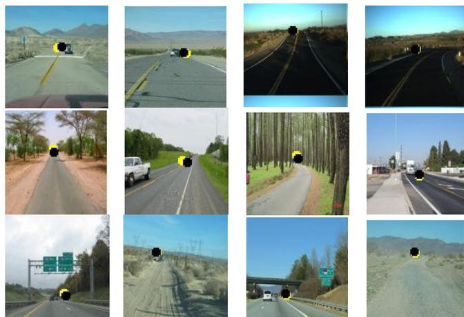
Fig. 7. Vanishing Point Detection results in yellow color with Ground Truth Positions marked with black color
