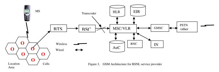
Base Station (BS): The base station is the gateway between the wireless network and wired network. It provides the wireless connection to the mobile subscribers within its coverage area (Cell). A set of base stations are connected to the MSC through a Base Station controller.
