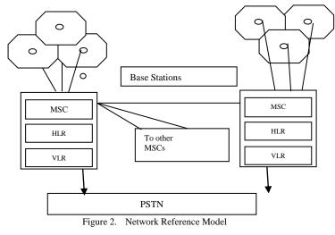
Mobile Switching Center (MSC): Responsible for switching the voice/data connection to the mobile host.
