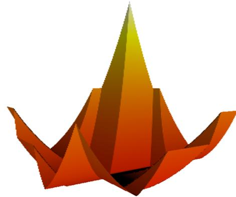
Figure 3. The 3-dimensional surface of a 2-dimensional function of a simple sensor location problem.
