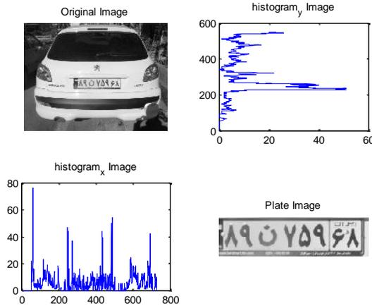
Figure 3. Extracted license plate using plate location technique
