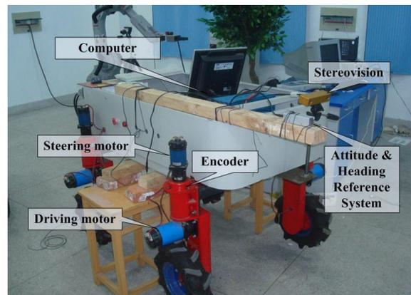
Figure 1. UGV used for navigation experiment.
