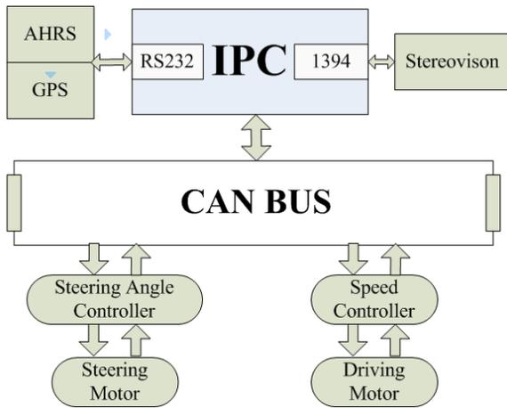
Figure 2. Hardware block diagram of UGV.
