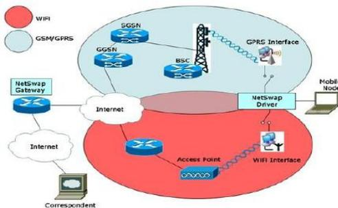
Figure 1. GPRS and Wi-Fi Interface
