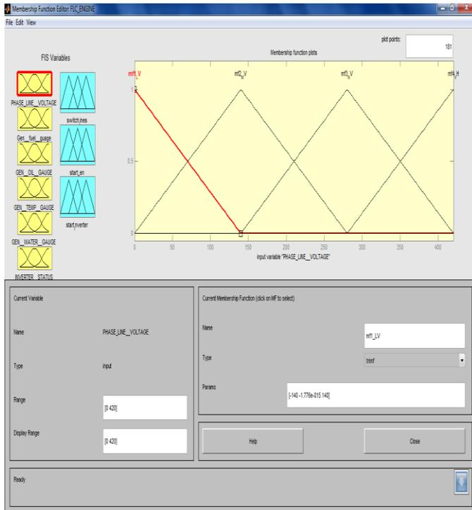
Fig. 6.1: Membership function of ICOFLS with FIS variable
