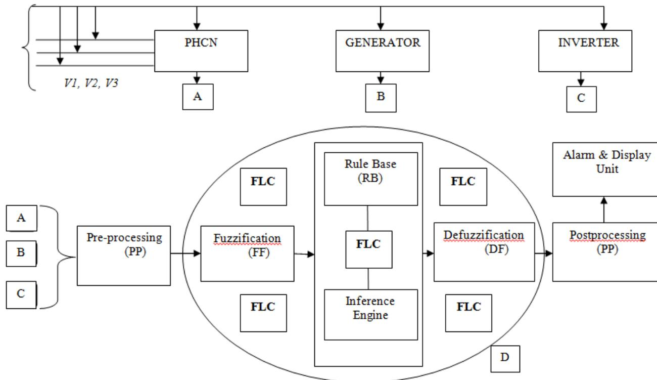
Fig. 2: System Architecture (ICOFLS)
