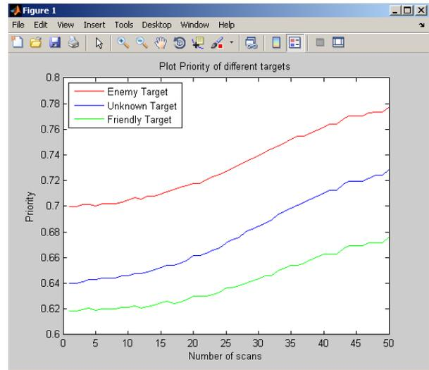
Figure 7. Priorities of 3 targets using Fuzzy logic
