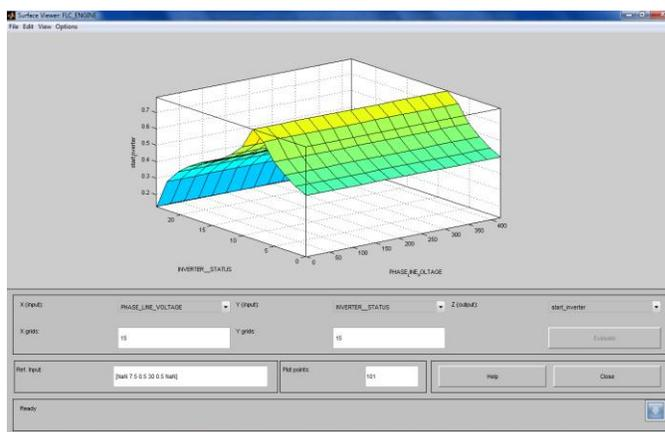
Fig. 6.10: ICOFLS surface viewer plots for the process variable (Inverter Status, phase voltage) and control variable start inverter.
