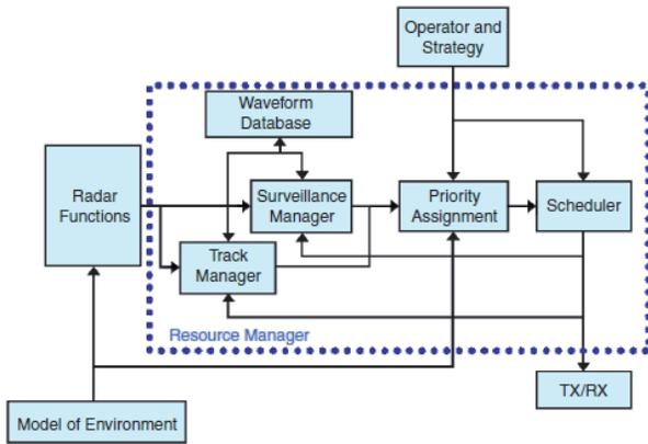
Figure 4. System architecture
