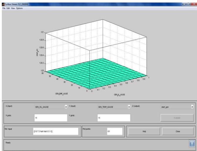
Fig. 6.8: ICOFLS surface viewer plots for the process variable (oil gauge, temp gauge) and Control variable: start gen
