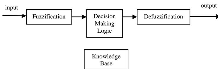
Fig. 4: Fuzzy Controller Block Diagram
