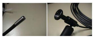
(a) Tip of fiber image scope (b)Outoptics of fiber image scope
