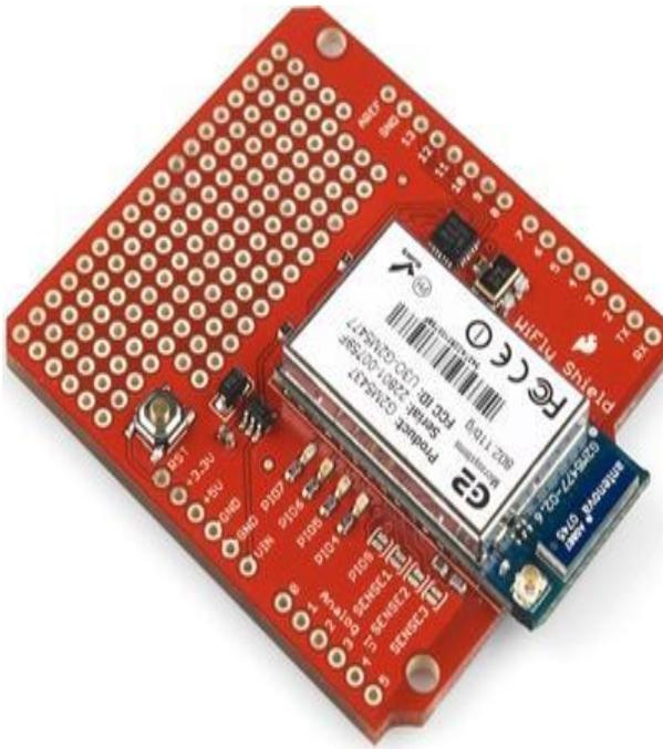
Fig. 3. Wi-Fi Shield (WiFly GSX)
